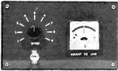
PAPER-SPEED control is first calibrated and then proper exposure is obtained by adjusting enlarger f-stop until needle is on line.
