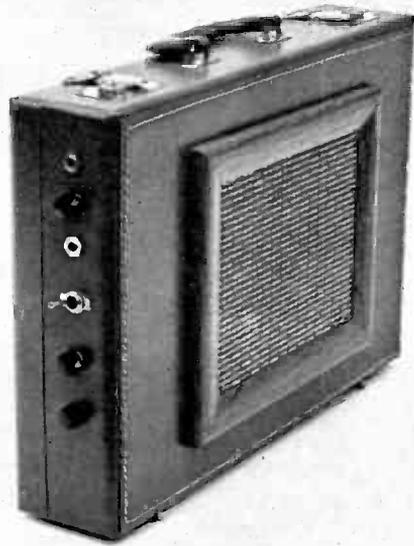
Fig. 4—Top jack is input, control below is volume. Next jack is for tremolo on/off foot switch. Bottom controls are tremolo speed and intensity
