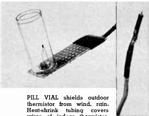
PILL VIAL shields outdoor thermistor from wind, rain. Heat-shrink tubing covers wires of indoor thermistor.
