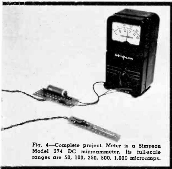
Fig. 4—Complete project. Meter is a Simpson Model 374 DC microammeter. Its full-scale ranges are 50, 100, 250, 500, 1,000 microamps.
