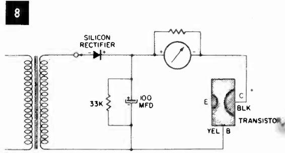
Shown here in simplified forms are circuit diagrams of Paco Engineering's T-65 tester, when set up for a short-circuit check, Fig. 7 above left; and when set up for base-to-collector current test, Fig. 8.
