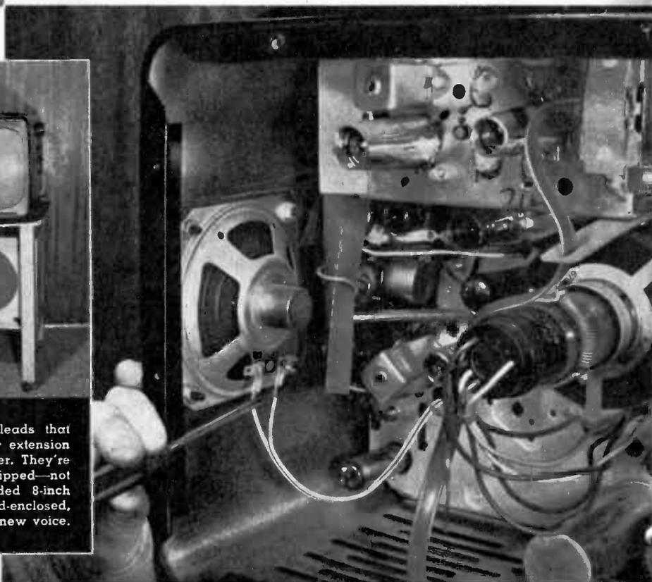
**T**HE PICTURE on my new 14-inch "portable" TV set was fine, but the sound was so miserable that something had to be done about it. The poor quality was due obviously to an inadequate little 3-inch loudspeaker. To make matters worse, this was mounted on the side of a thin metal cabinet, which rattled like a bunch of tin cans.
