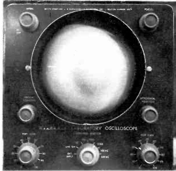
Alternating voltage on horizontal deflection plates (with no input on vertical) sweeps spot back and forth forming flat line. This voltage usually comes from "sweep" generator, an integral part of scope.
