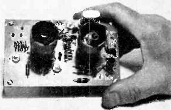
Completed converter is but a handful. Crystal is behind right-hand tube. Note how resistors, capacitors, and coils fit holes in the printed board.
