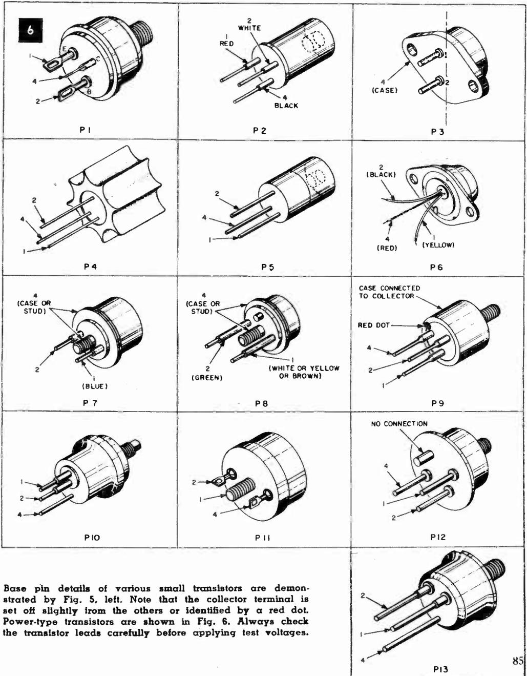
Base pin details of various small transistors are demonstrated by Fig. 5, left. Note that the collector terminal is set off slightly from the others or identified by a red dot. Power-type transistors are shown in Fig. 6. Always check the transistor leads carefully before applying test voltages.
