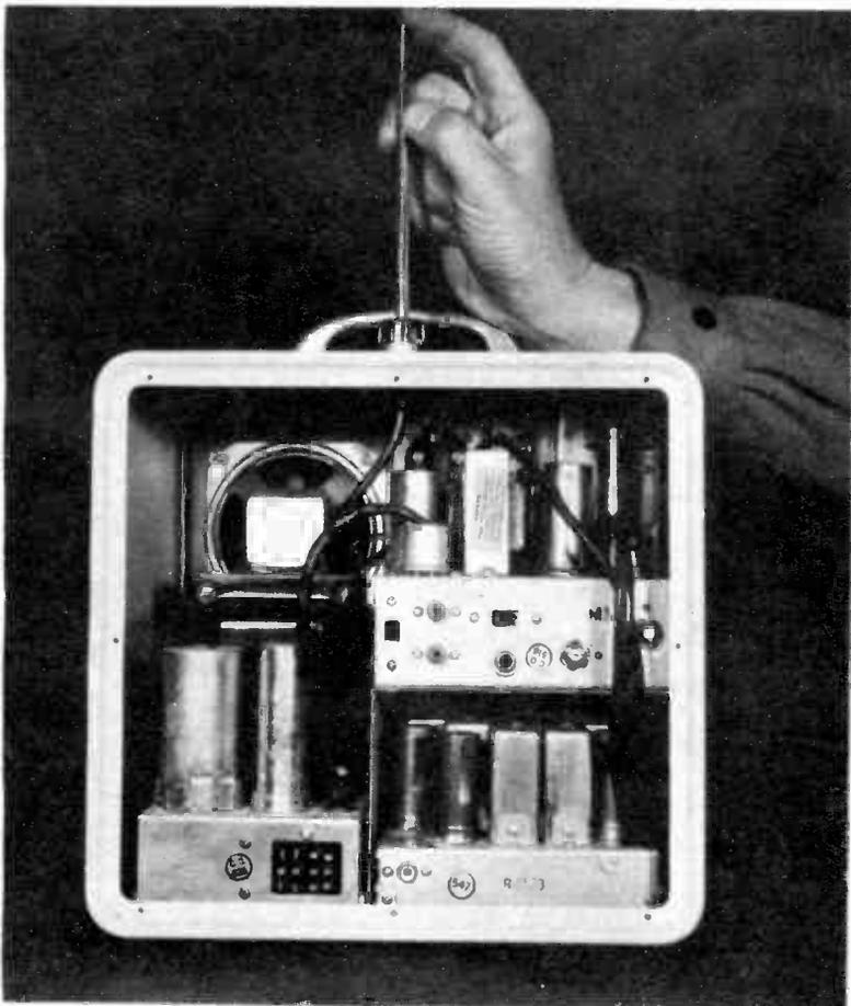
Rear view of Communicator III reveals its well-filled cabinet. Transmitter section is at upper right, receiver at lower right, convertible power supply and loudspeaker are at the left of photo.
