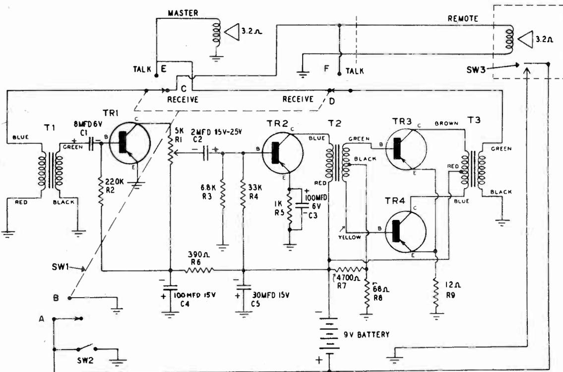
Wiring diagram of Lafayette Radio's KT-113 transistor intercom.
