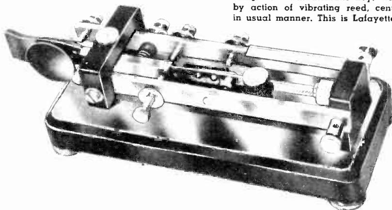
"Straight" key, the use of which is known as "pounding brass." In the early days of radio telegraphy, hand keys were of machined brass.
