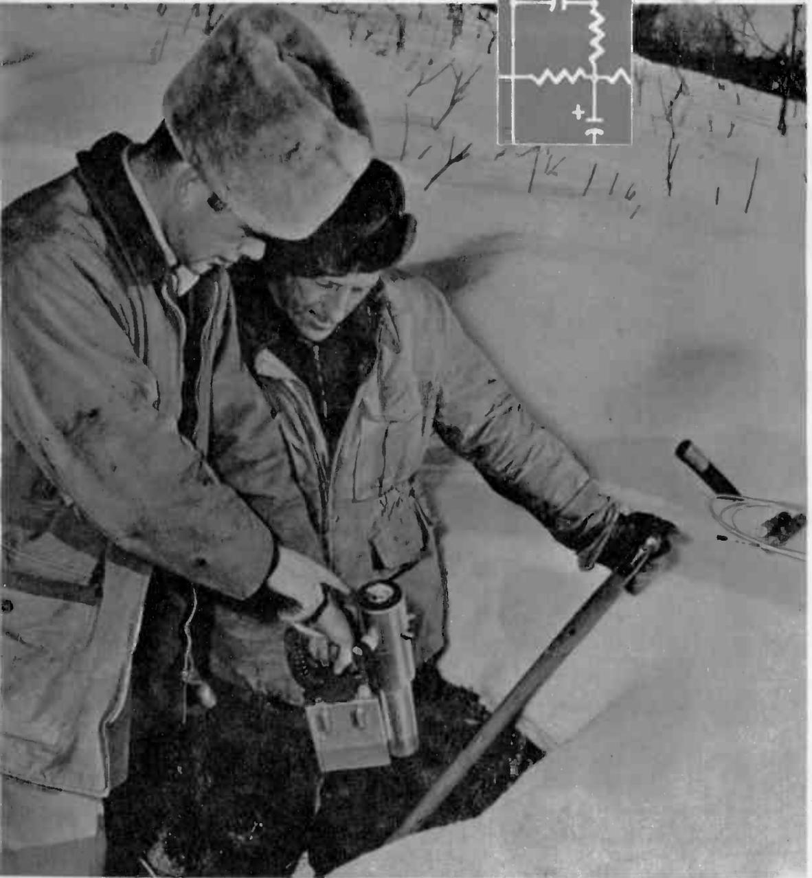
Radiation detectors and counters are among the many devices that require low-current high-voltage power sources. The uranium hunters above use a model made by Precision Radiation Instruments.
