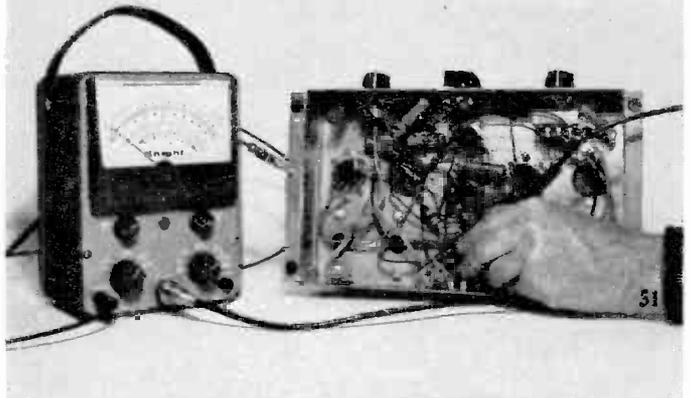
probes and turn on the amplifier. The meter reads between 4 and 6 volts, 5 being the rated filament voltage. Why the caution above removing the hands? Because points 2 and 8 happen also to represent the highest DC voltage in the circuit, in relation to the metal chassis. We'll come to that in a minute.
