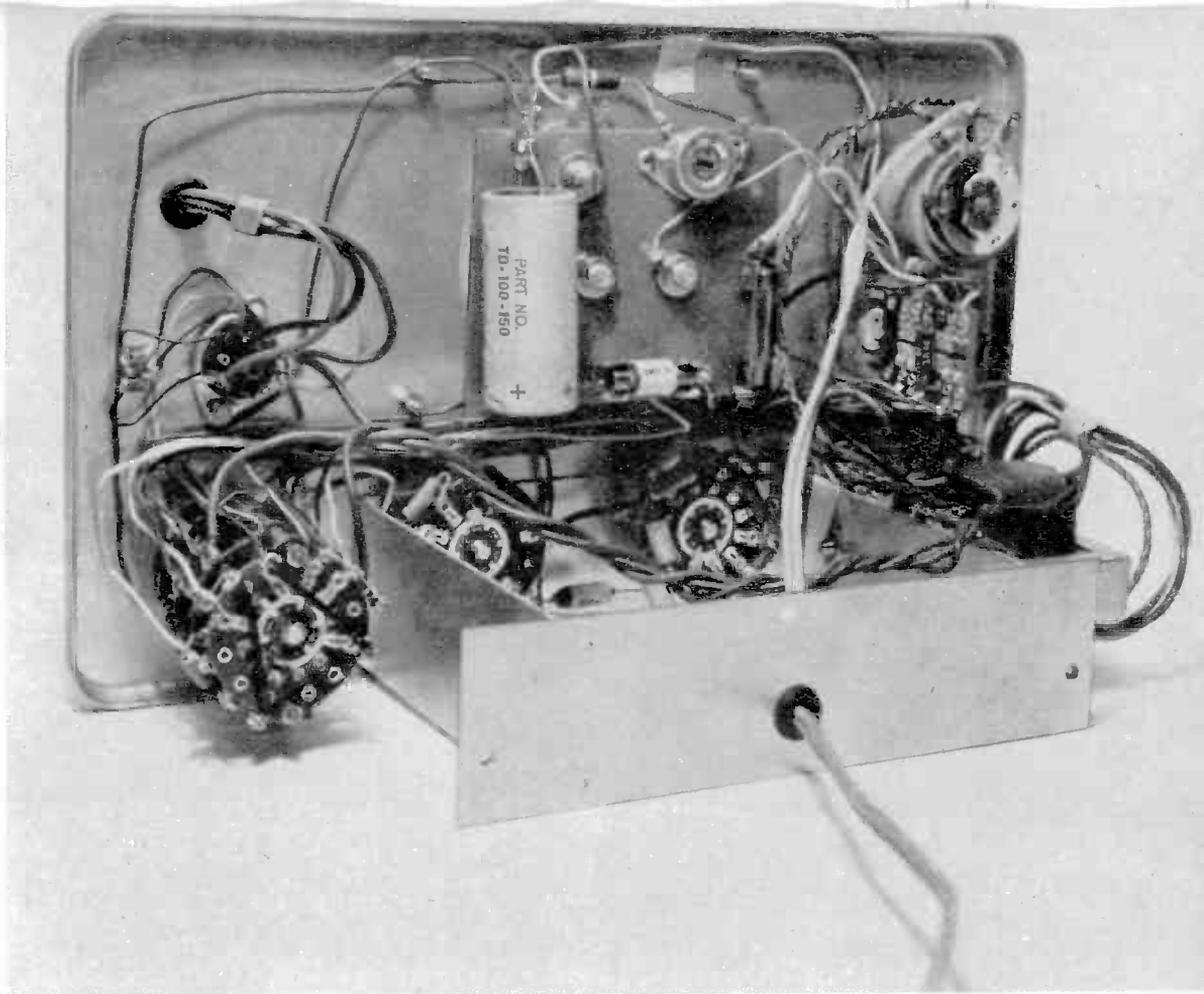
Seen in this photograph is the interior of the Paco transistor checker, which was assembled from a kit. The wires carry only 60-cycle AC and low-voltage AC, so they can be pushed together safely.
