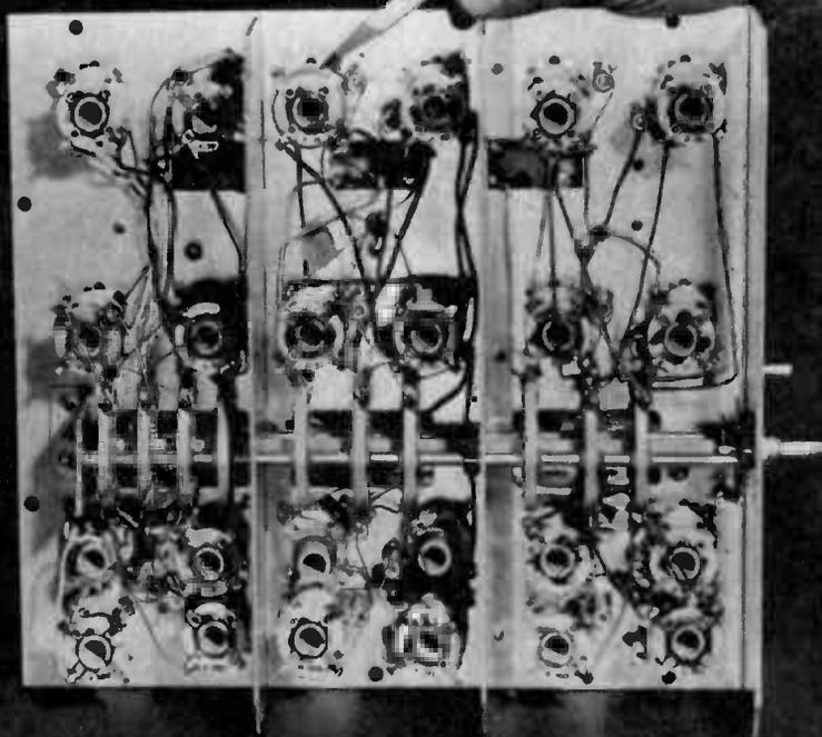
View from below front end of the Mohawk receiver. Pencil indicates one of 24 coils, all preset at the factory. Note ten-section bandswitch runs between the banks of coils.
