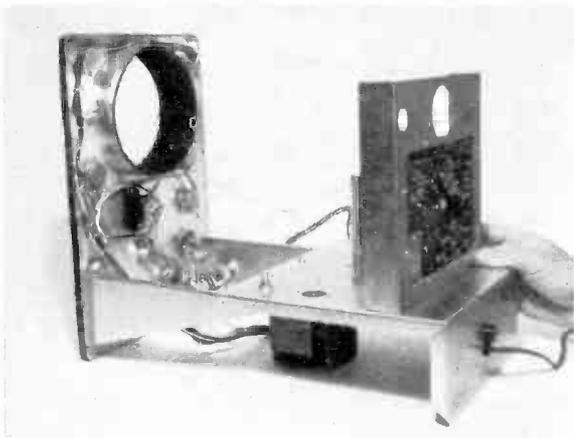
This shallow chassis bolts vertically to top of the power-supply section, as at left. This serves as support for the neck of the cathode-ray tube.
