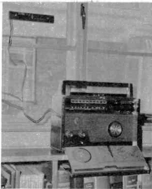
For broadcast reception, detachable Wavemagnet antenna is effective in shielded buildings, cars, etc. Suction cups hold it to the window.
