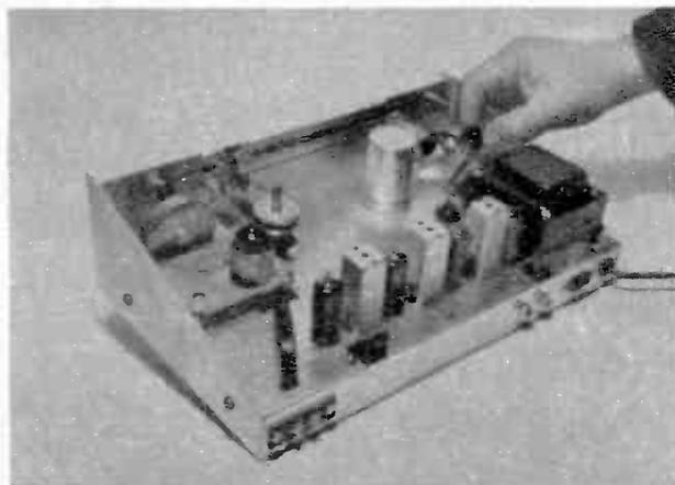
The completed tuner is shown in the photograph at lower left. The last tube is being inserted in its socket. It is installed at an angled position so that it will clear the tuner's metal enclosure.
