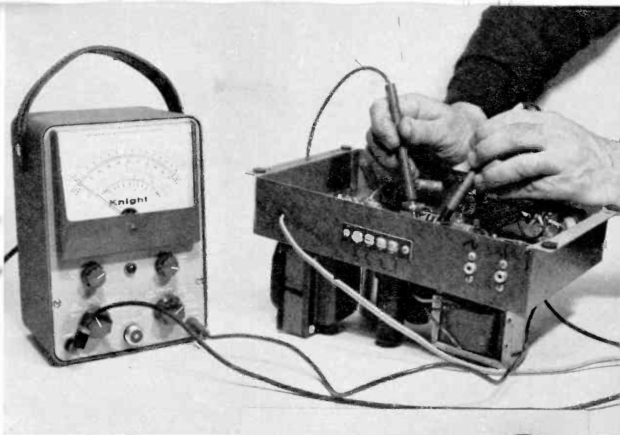
For checking AC voltages and making resistance measurements, it is usually convenient to use two long-handled probes with the VTVM (vacuum tube voltmeter) as demonstrated above.
