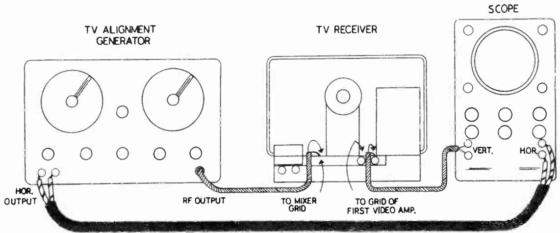
True "alignment" of a TV receiver, complicated and difficult by any other means, is accurately accomplished when the oscilloscope is used as a wave-form indicator. This is the typical bench setup.
