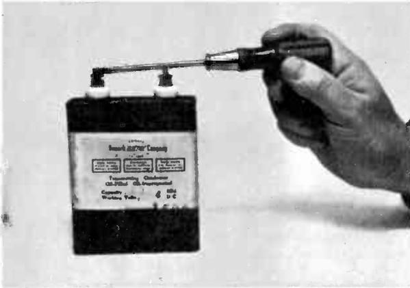
Avoid shock danger; discharge filter capacitors.
