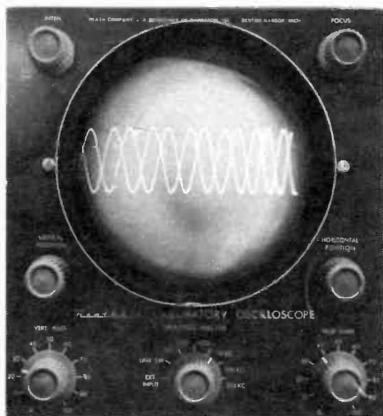
Flicker is no problem at high input signal frequencies; any number of stationary cycles can be obtained. Here, input is 1600 cps, sweep is at 100. The number of complete cycles is 16.
