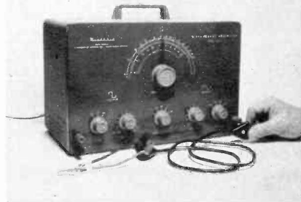
Front panel of the completed Heath AG-10. Upper central knob is tuning for different frequencies. Other knobs adjust strength of output signals.
