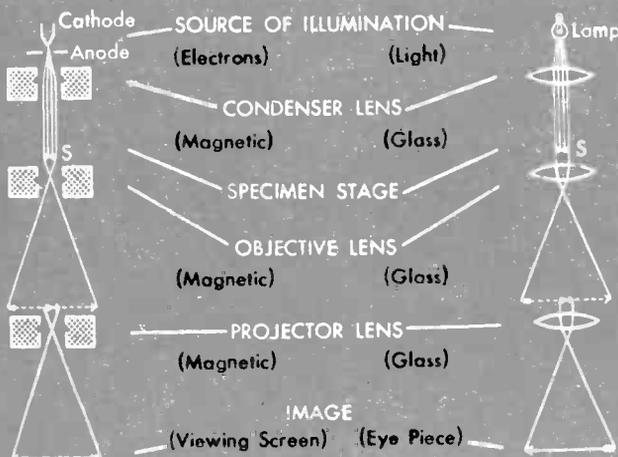
Similarities and differences of electron and light microscopes. Size differential is not indicated. RCA's EMU-3 more than seven feet high, almost five feet wide and deep, weighs 1400 pounds.
