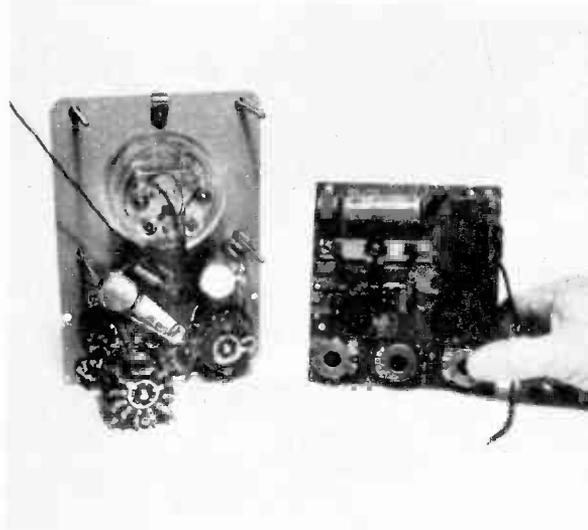
Tubes and other major circuit elements of the Knight VTVM mount on printed-circuit board, right of photo above. This in turn attaches by four long screws that surround meter. At the left is an interior view of the completed VTVM. Whole assembly job can be completed in two evenings.
