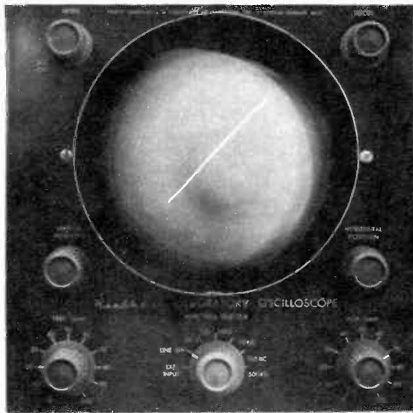
Such a flattened ellipse indicates 180° phase difference. Line leaning in other direction would mean in-phase condition. Intermediate phase relationships of signals can be readily determined.
