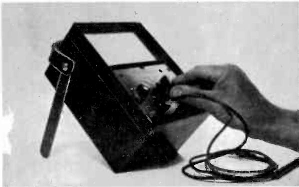
Meter to which  $\frac{1}{8}$  by  $\frac{3}{4}$ -inch Masonite legs have been added can be scanned quickly and easily.
