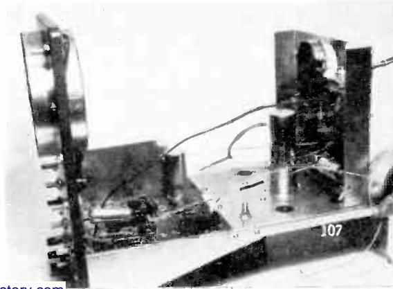
Circuitry of the Heath O-11 scope. As evident, ten tubes, many resistors and capacitors are employed.
