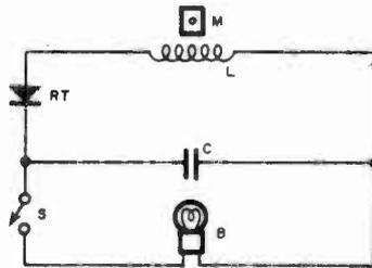
**T**HE CONVENTIONAL BATTERY has been eliminated entirely and replaced by a unique little generator system in a new flash gun introduced recently by Kodak. To charge the capacitor that actually fires the flashbulb, the user merely makes a half turn with a small nylon hand wheel that's approximately the size of an ordinary radio knob.
