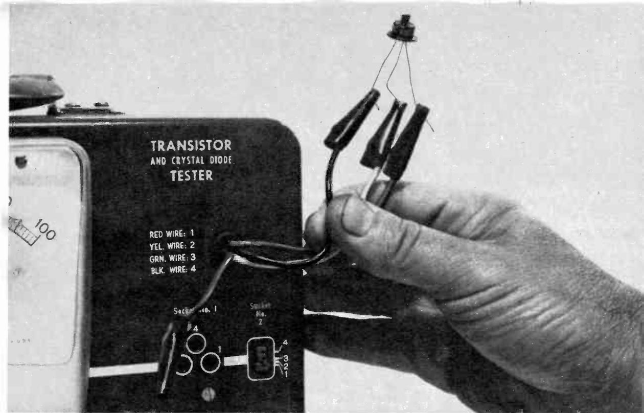
In most cases, you'll find that it's less trouble to connect a transistor for testing on the T-65 by means of these flexible wires with alligator clips. All of the wires parallel the socket connections.
