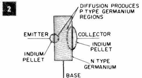
Figure 2. Cross-section construction of a typical transistor of the diffused germanium type.
