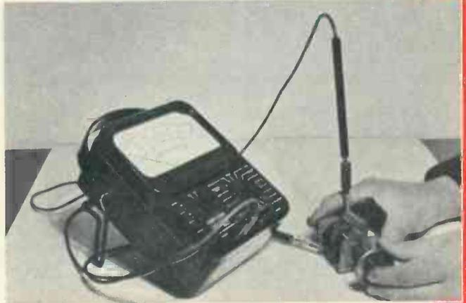
**NOISY RECEIVER?** If radio receiver is unaccountably noisy when dial is turned, check variable tuning capacitor. Remove from chassis, connect circuit tester, turn shaft, test for short as shown in photo.
