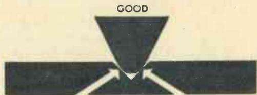
GOOD—STYLUS IN GOOD CONDITION RESTS ON SIDES OF GROOVE.
