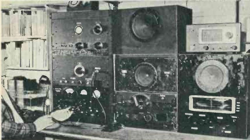
"Relay rack" construction is employed for unit at left of this impressive 3-receiver, 2-transmitter collection. In lower center is revamped Air Force BC-348 receiver; above it, speakers for it and other next to it on the left. Though combination is extremely heavy, weighing several hundred pounds, it's easily movable on casters.
