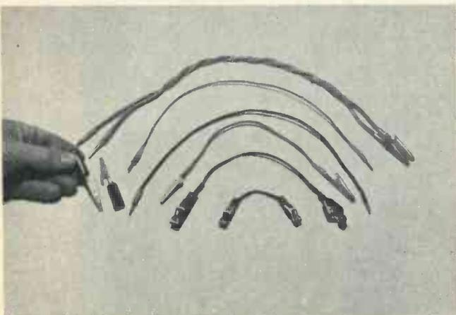
**HANDY TEST LEADS:** For quick temporary connections, a collection of flexible leads fitted with alligator clips is useful. Use No. 18 lamp cord; fit some wires with phone tips for connection to binding posts.
