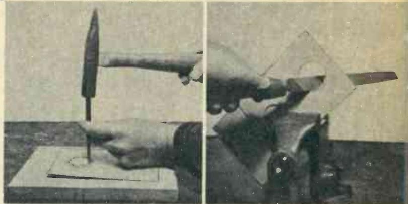
Typical construction requirement is a rectangular opening 1 1/2 x 2 1/4 inches for a transformer. The area has been covered with wrapping paper.
