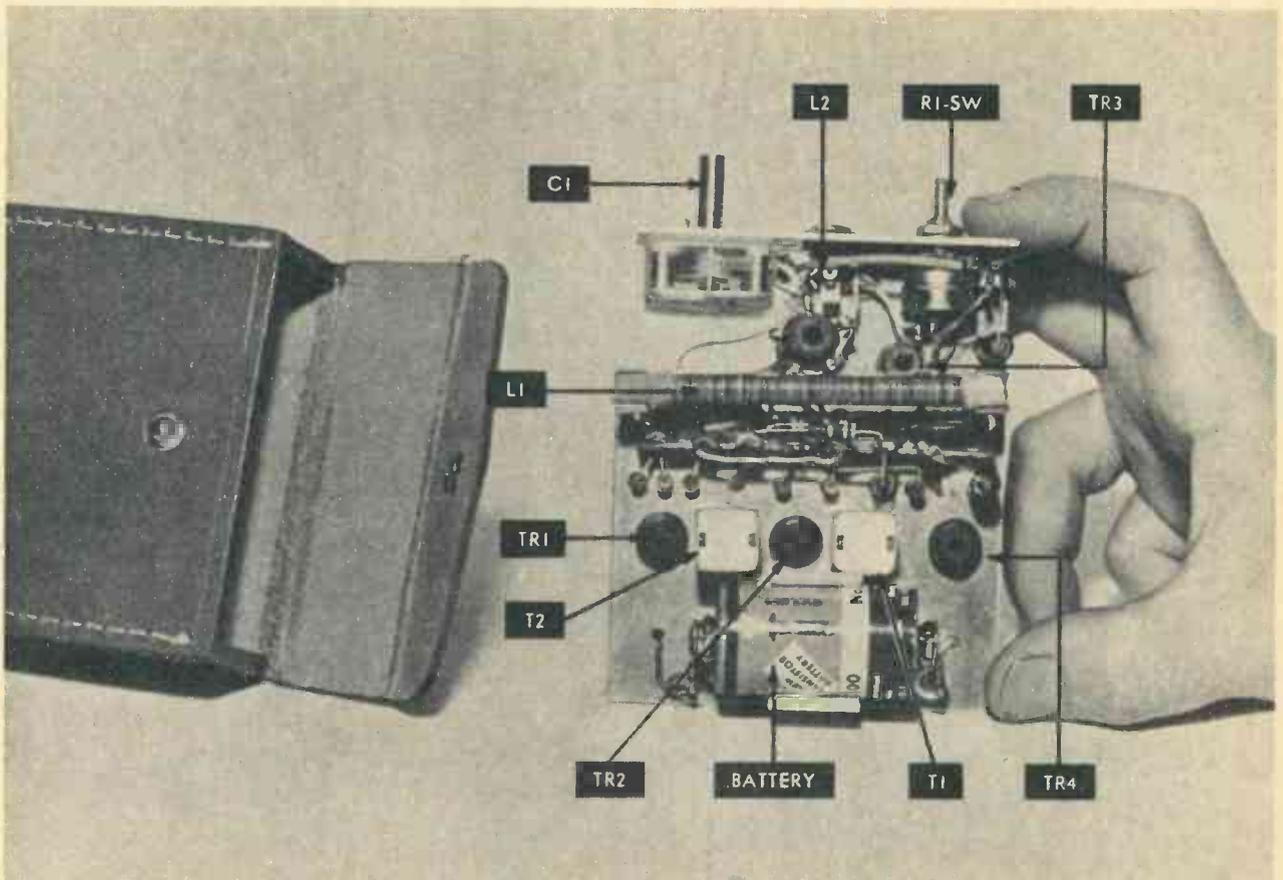
This is a top view of chassis, removed from carrying case, with parts marked to correspond with schematic diagram. Battery has snap connectors and fits in U-shaped clip. Other parts are very small. Transistors are size of an eraser on lead pencil. Tiny transformers T1 and T2 measure merely 1/2 inch square by 3/4 of an inch in height.
