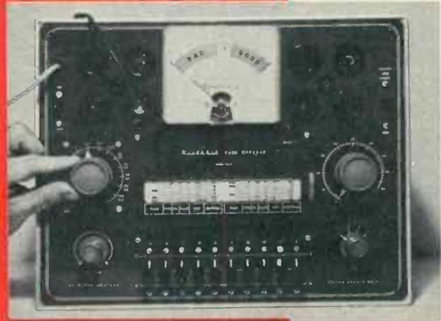
In front panel view, user turns roll chart to find proper tube-type. Note that lever switches, bottom, are centered.
