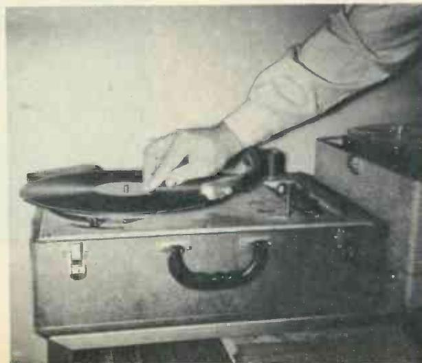
The disc to be taped is "cued up" by manually turning it until sound begins, then turning it back two revolutions.
