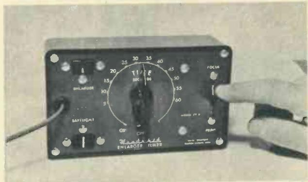
Main control switch, right, stays closed on "Focus." When pressed once to "Print," it starts enlarger timing cycle.
