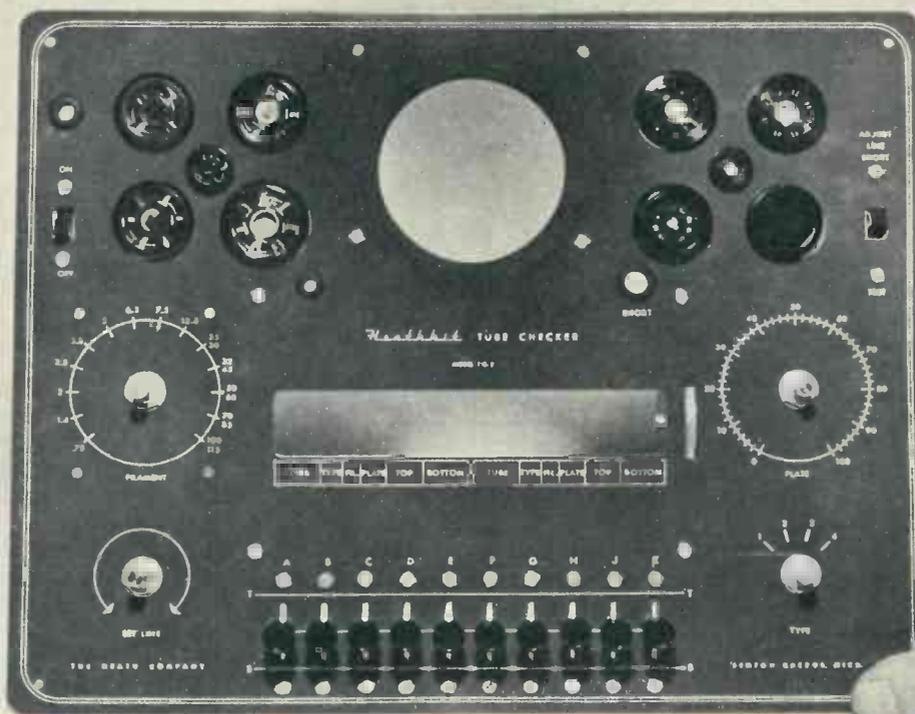
Front panel of Heathkit tube checker after assembly of the tube sockets, lever switches, at bottom, and other controls.
