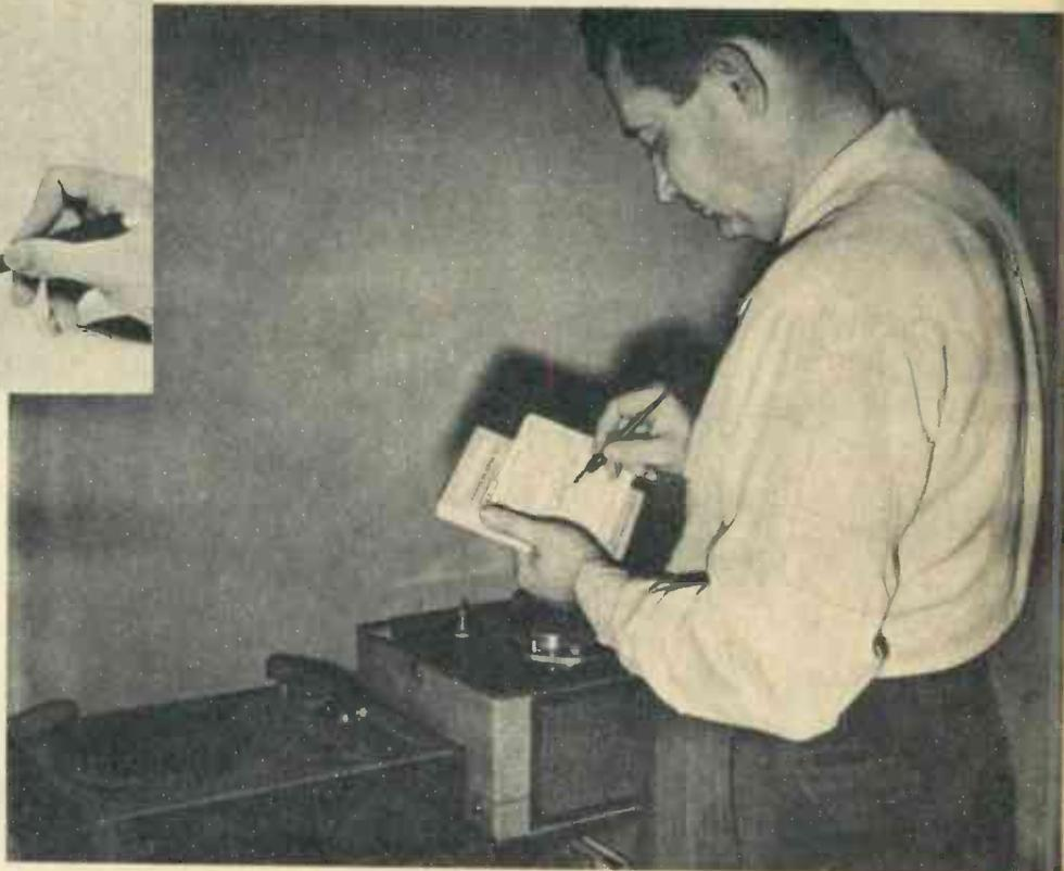
These bulk tape erasers will erase even the most powerful signals from a recorded tape in a few moments; these devices clean the entire tape at once.
