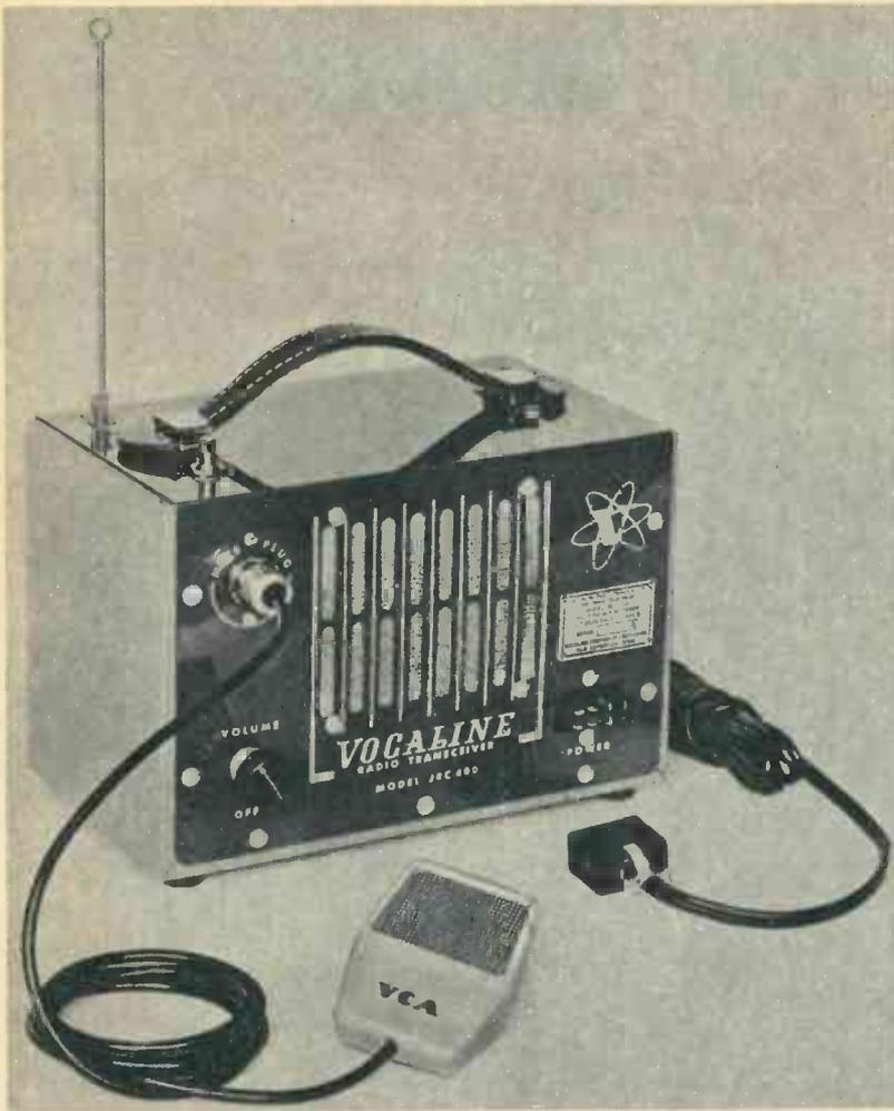
There are no external tuning controls on Vocaline JRC-400. To talk, operator presses the button in top of cabinet. To listen, he releases it. Price is \$69.75.
