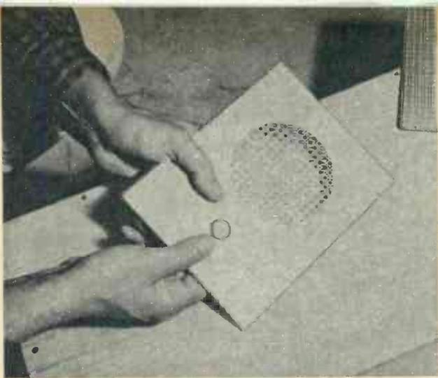
Cut button hole in aluminum over previously drilled hole in plywood. Install button from front as in photograph.
