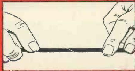
Align and butt together the tape ends, with the uncoated (shiny) side upward.
