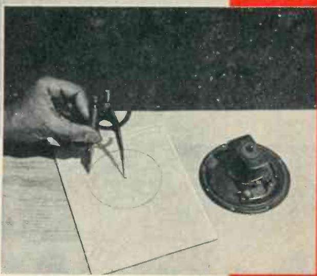
To make wall speaker, mark a hole on plywood rectangle with your compass to fit inside diameter of speaker flange.
