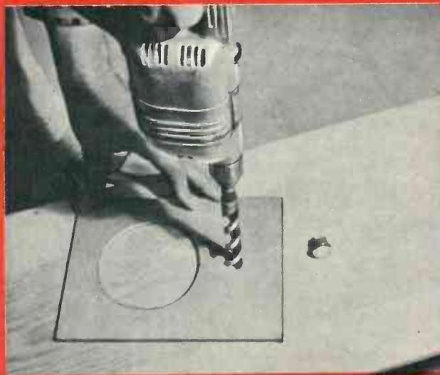
Drill hole in bottom of plywood shape to house the button. Such buttons are inexpensive at electrical supply stores.
