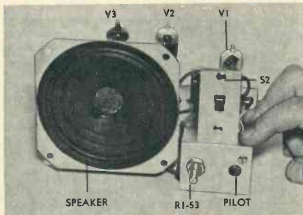
Master chassis is little more than a handful. The speaker, switch and volume control mount permanently; entire unit then slides into cabinet and volume control knob is added.
