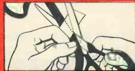
After tape is joined properly, trim and undercut it slightly to avoid sticking.
