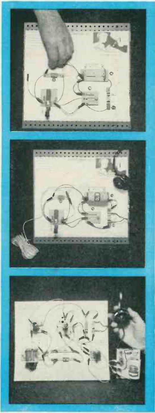
This is same peg board shown in preceding photograph, but parts are arranged to form a code practice oscillator. Template is included in kit.
