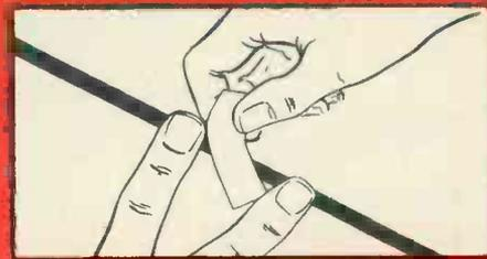
Smooth out the air bubbles after applying cellulose tape; do not use metal.
