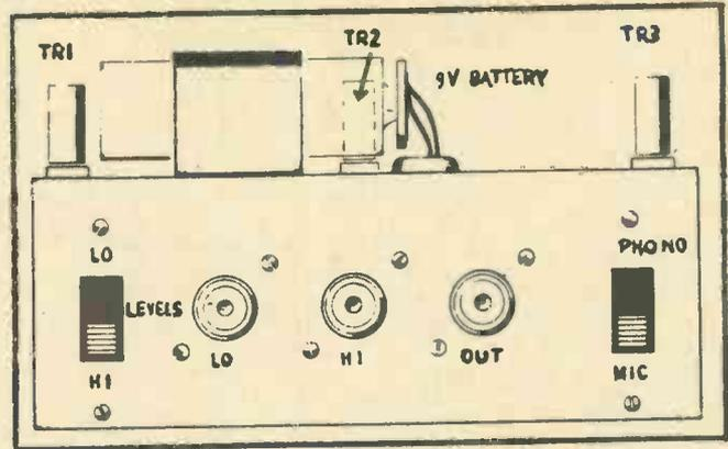
Above, right, a rear view drawing of the Lafayette kit; transistors used are all General Electric type 2N190.
