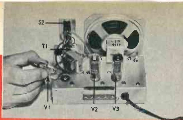
Back view of master chassis. Transformer T1 is angled to minimize magnetic coupling with Transformer T2 below it.
