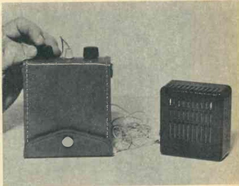
Loudspeaker unit on right contains its own amplifier and connects to receiver proper by a flexible cord. Speaker measures  $2\frac{3}{4} \times 3 \times 1\frac{1}{4}$  inches; set,  $3\frac{3}{4} \times 4\frac{1}{4} \times 1\frac{3}{8}$  inches.
