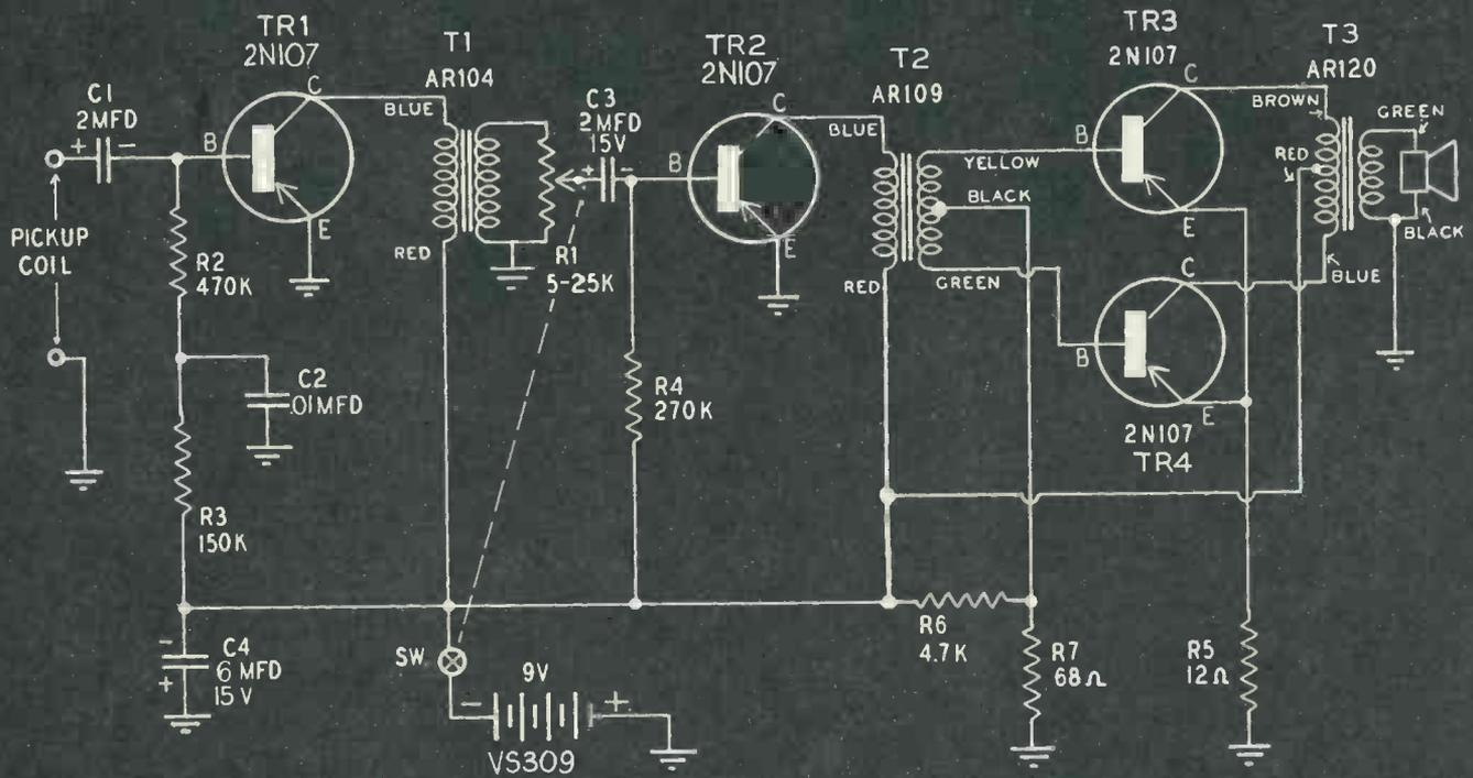
Circuit of telephone amplifier is conventional and straightforward. The letter "K" after resistor values indicates 1,000; therefore "150K" means 150,000 ohms. Pictorial wiring diagram shows parts marked as in schematic above.
