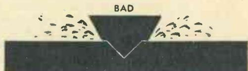
BAD—CHISEL-LIKE, WORN OUT STYLUS SINKS INTO BOTTOM OF GROOVE AND SCRAPES MUSICAL IMPRESSIONS OFF GROOVE WALLS.
