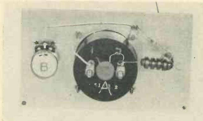
Simply assembled and operated, the R.F. power meter, shown in top and chassis views, contains but half a dozen components, weighs but a pound, case included.
