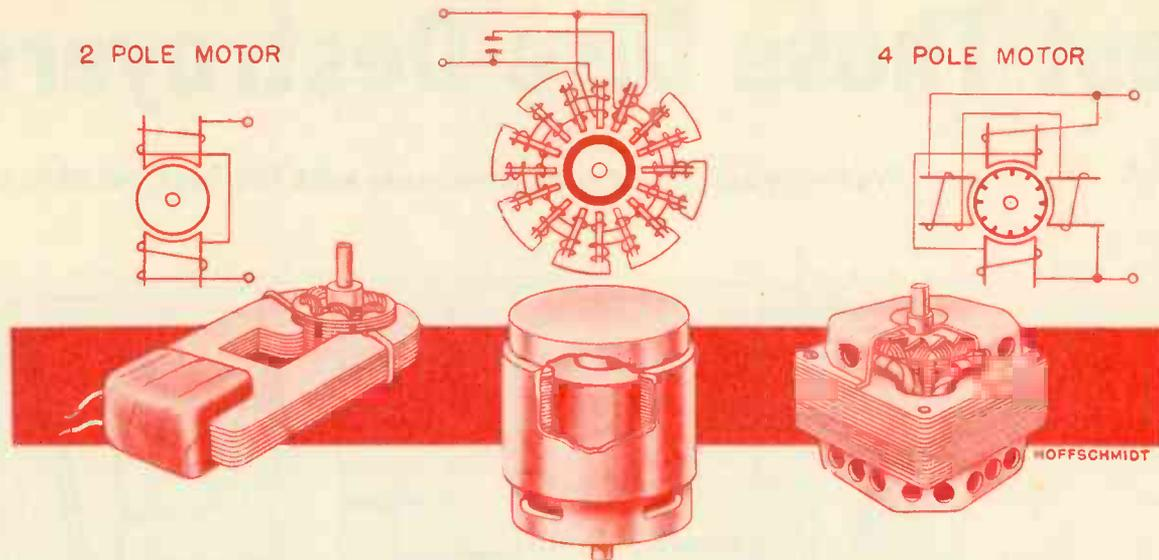
Three types of turntable motors are shown: hysteresis synchronous is best for avoiding low-frequency "rumble."
