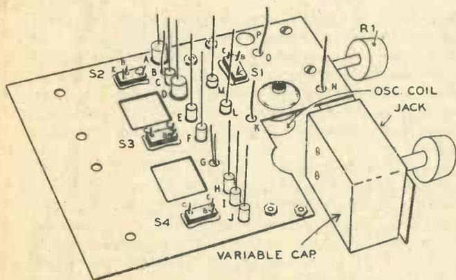
Wiring is simplified by having various small resistors and capacitors, lettered A through M, sitting vertically in holes in chassis. Pig-tail leads go to next soldering point.
