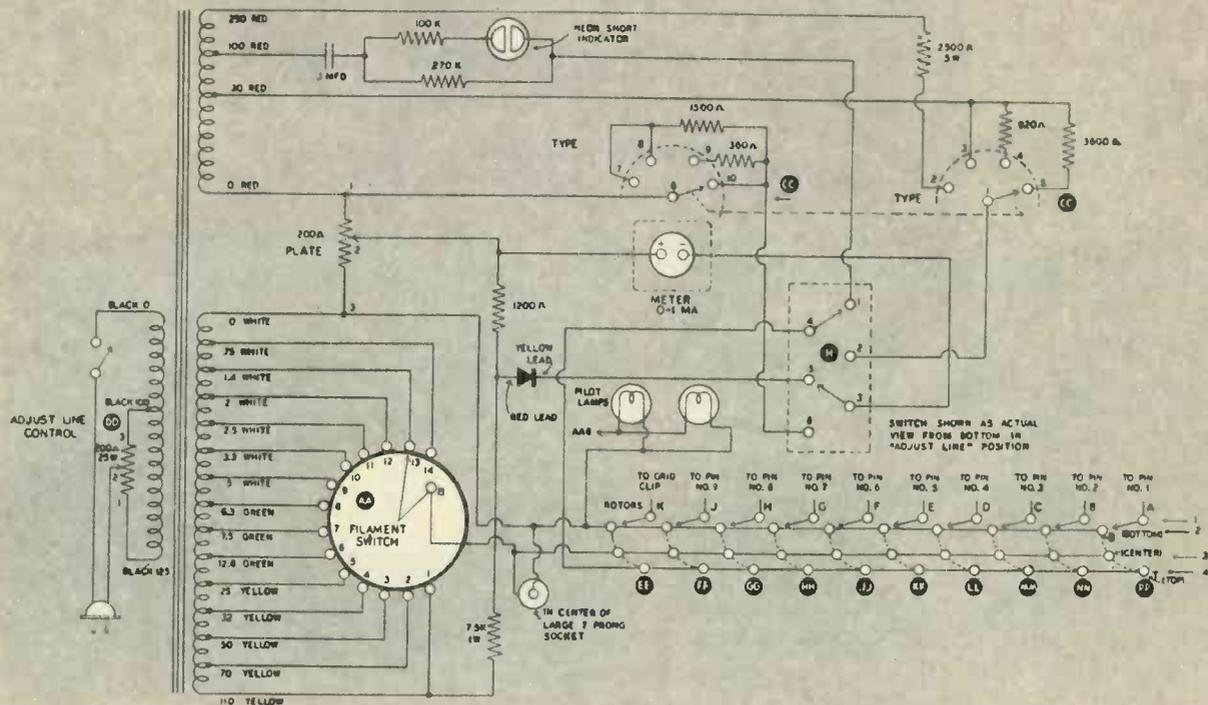
Complete schematic diagram of the Heathkit tube checker. The lever switches are marked A through K. The rectifier, marked "Yellow Lead-Red Lead," is used only to make 0-1 milliampere DC meter read equivalent of the line voltage.
