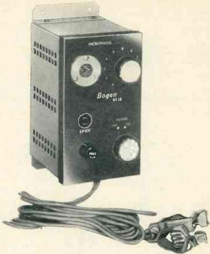
No vibrator is necessary for this compact amplifier, thus eliminating one of the more vulnerable elements in ordinary mobile amplifier installations. Voltages are low, safe.
