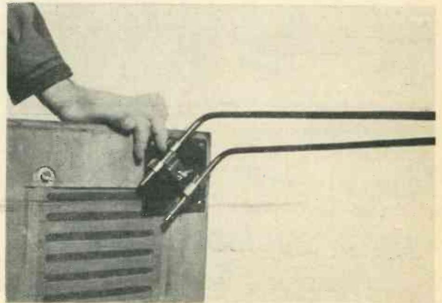
The legs—black iron, in this case—are secured by cross clamps which need but a single wing bolt in the center. They can be attached or removed simply.
