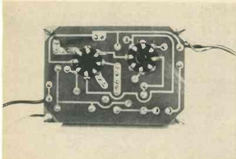
"Wiring" of signal injector involves simply applying solder to component pigtail ends coming through the board.
