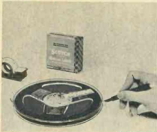
Left and below, written identification of what is on the tape is made on both the tape box and the plastic spool.
