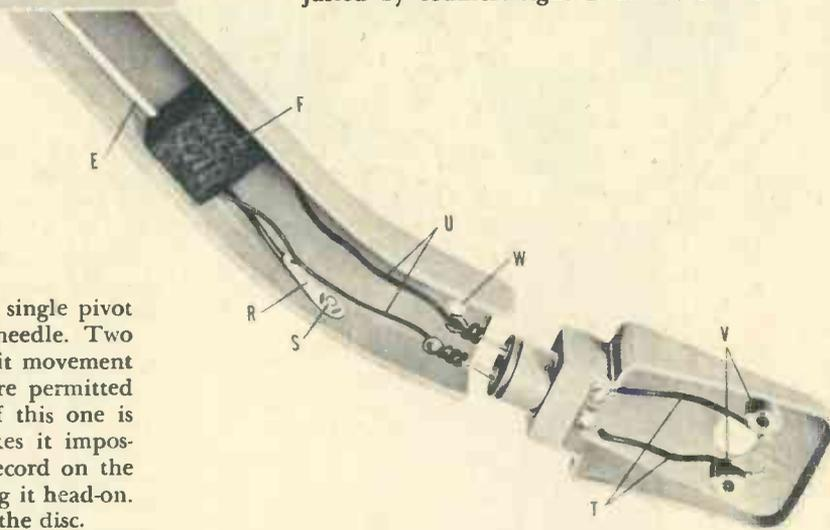
Above, cartridge case is cut away at sides to permit observation of stylus at all times. Knockout hole between mounting holes V allow insertion of control for "turn-around" cartridges. Case is attached to arm by screw through W, electrical connections U are made through pin-jack setup.
