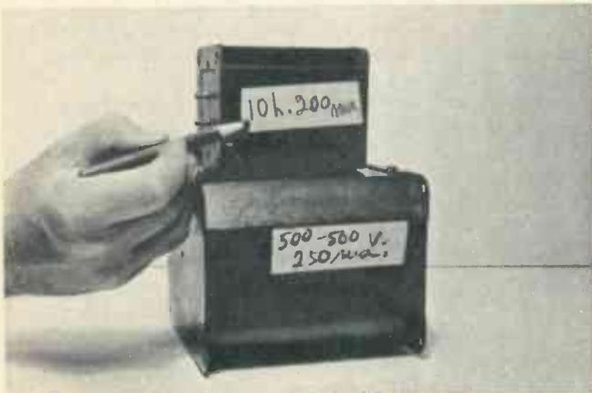
**STICK-ON LABELS:** Lock up technical data for transformers and filter chokes, mark it in grease pencil on masking tape, stick to cases to save bother of consulting dozens of catalogs to identify later on.
