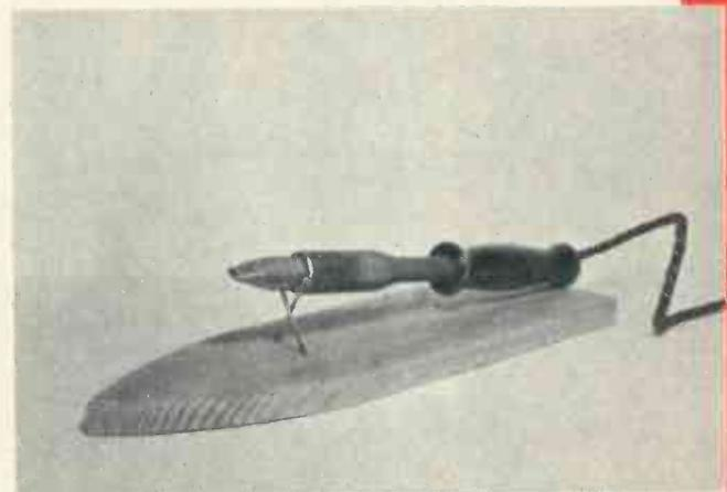
**SOLDERING IRON SUPPORT:** When iron is hot and you need both hands free, this stand is made to order. Merely drive two nails into a scrap board to form an "X." Base here is fence picket.
