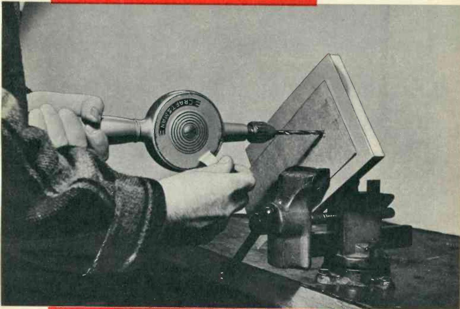
**M**AKING LARGE HOLES in aluminum and steel panels and chassis for numerous electronic components is a constantly recurring problem for experimenters and constructors amateur and professional alike. Round holes from about  $7/16$  inch through  $1\frac{1}{2}$  inches are needed for switches, jacks, volume controls, etc.; square or rectangular openings are needed for transformers, choke coils, etc.
