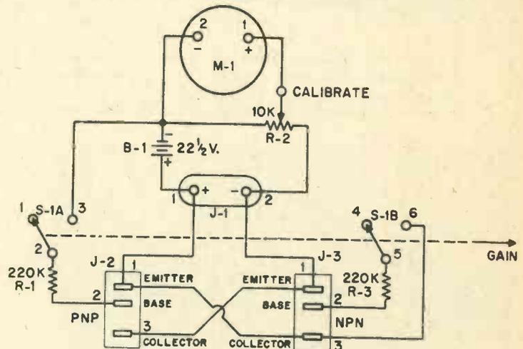
Simplified schematic diagram of the transistor checker. Switches S-1A, S-1B are actually one: LEAKAGE-GAIN.
