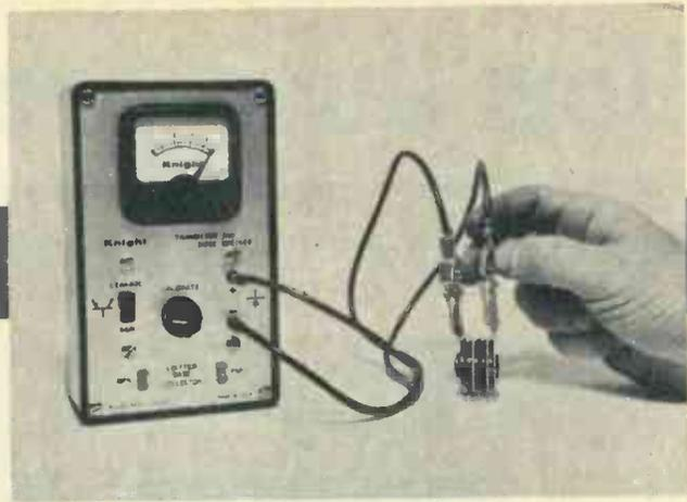
As its name indicates, the checker is used for diode rectifiers as well as transistors. Silicon, other types of diode rectifiers, are connected for test with flexible leads.
