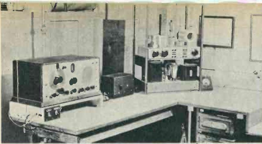
Receiver of this snug, modest ham shack is raised 3 inches above table, and the space beneath it provides convenient storage. Switches on dark panel, lower left, control transmitter. Latter, at right, is built up of uniform-sized aluminum chassis, supported on an open frame of angle iron. Parts are readily accessible.
