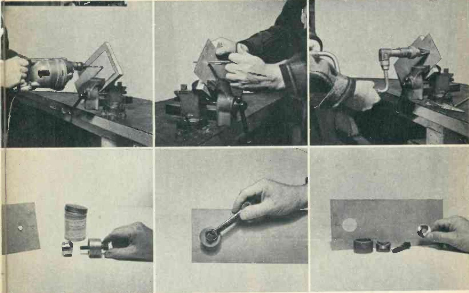
Fastest, cleanest job is done by hardened steel chassis punches like this. Center screw draws cutting section through panel, into hollow body of die.
