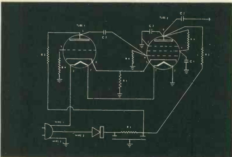
Two-tube circuit, which is AC operated, is basic multi-vibrator oscillator. Output signal is fed to probe through C2.
