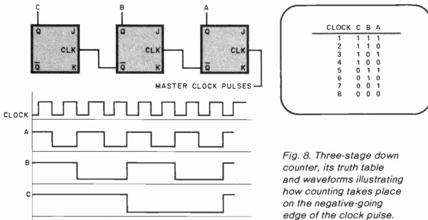
Fig. 8. Three-stage down counter, its truth table and waveforms illustrating how counting takes place on the negative-going edge of the clock pulse.
