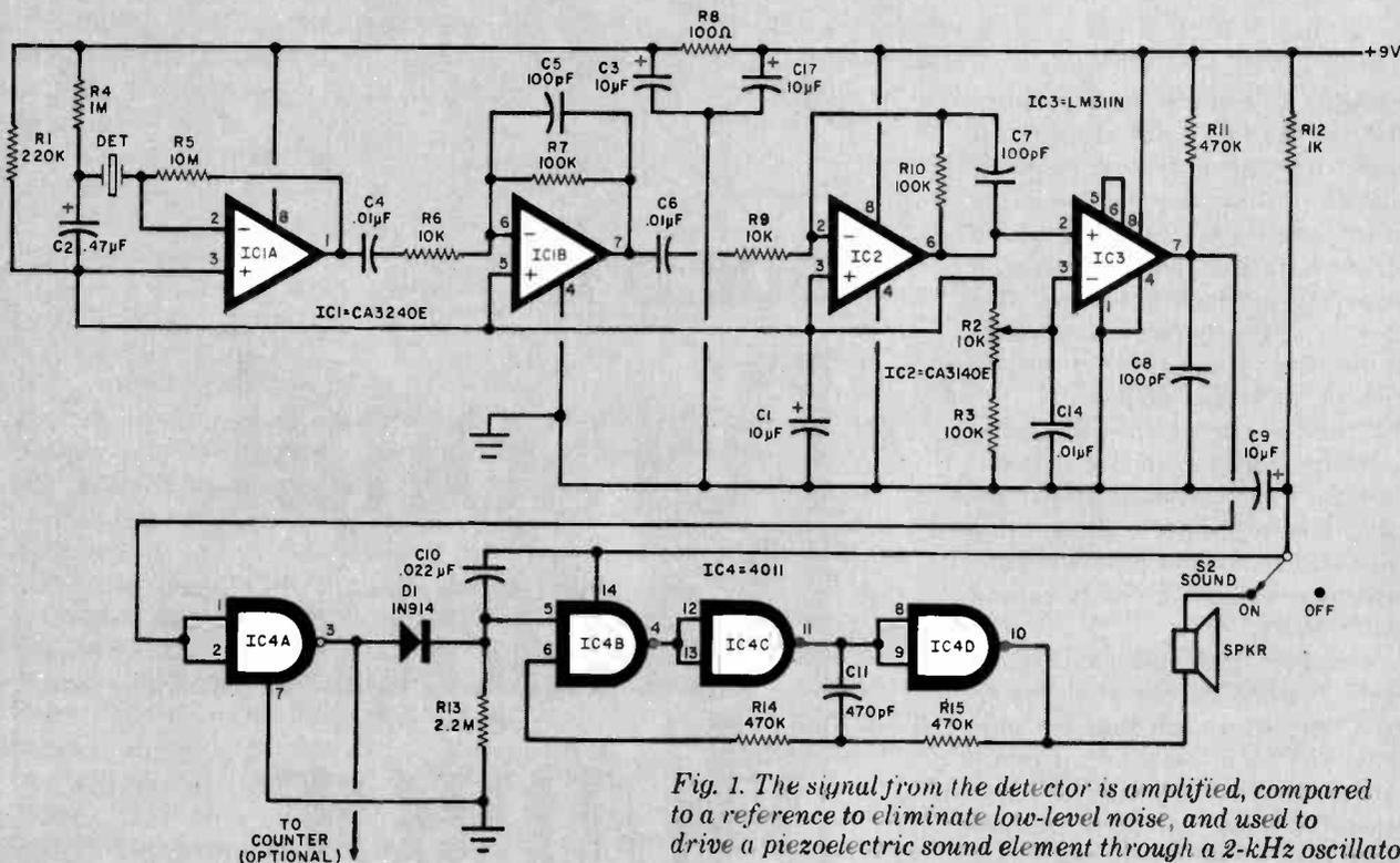
Fig. 1. The signal from the detector is amplified, compared to a reference to eliminate low-level noise, and used to drive a piezoelectric sound element through a 2-kHz oscillator.
