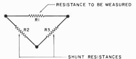
Fig. 2. Generalized model of a circuit containing a resistance to be measured and shunting components.
