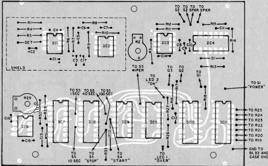
*Fig. 3. Actual-size etching and drilling guides for the two-sided pc board are shown below. Component mounting on the top is at left. Note that the upper portion of the board (containing the audible circuit shown in Fig. 1) can be detached if only that circuit is to be used.*
