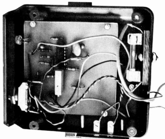
Internal view of the author's prototype shows circuit board in container with LED and switch on front and power leads exiting through back. Terminal strip on side is for leads to the thermistor.
