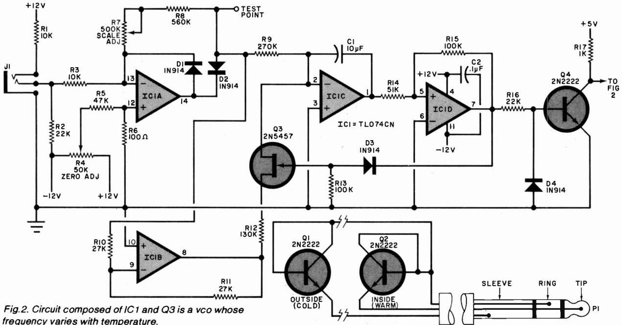
Fig. 2. Circuit composed of IC1 and Q3 is a vco whose frequency varies with temperature.
