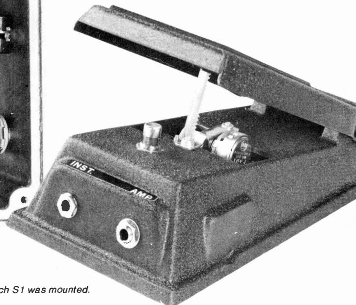
Fig. 5. View of pedal showing how switch *S1* was mounted.
