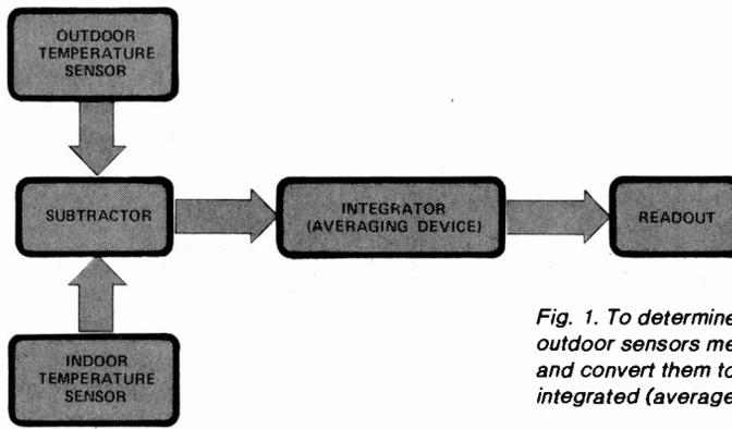
Fig. 1. To determine degree-days, the indoor and outdoor sensors measure temperatures and convert them to voltages, which are subtracted, integrated (averaged) and applied to readout.
