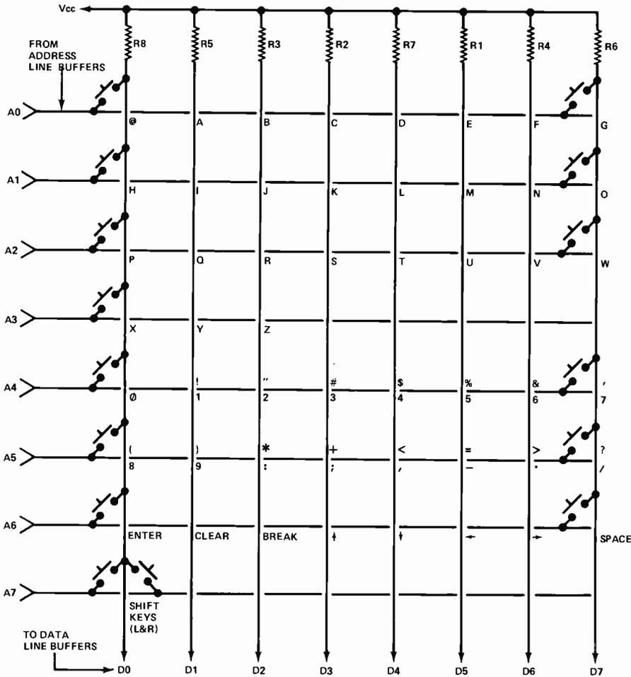
*Schematic shows 8 × 8 matrix layout of the TRS-80 keyboard, which is typical of boards of this type. A keyswitch is located at each intersection of the matrix to generate an output for a specific character.*
