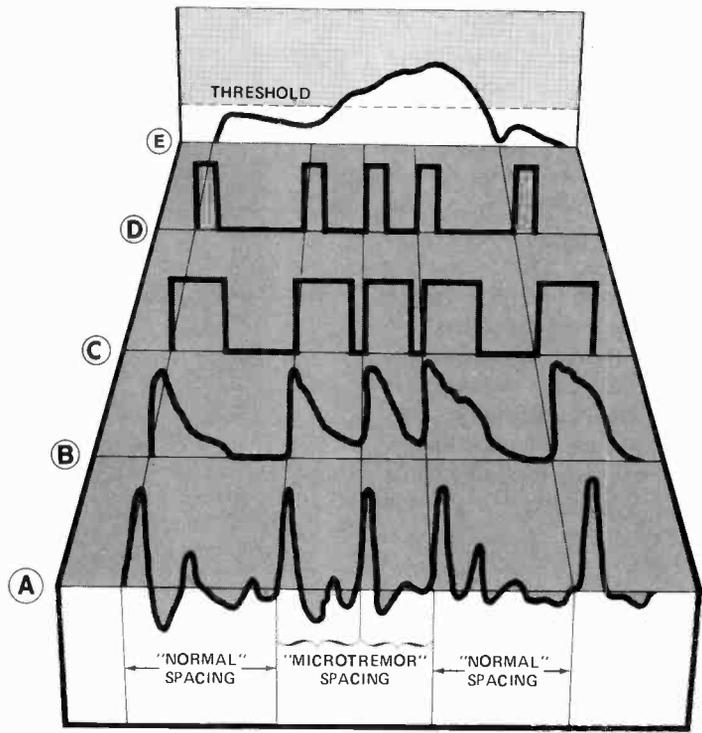
*Fig. 3. Typical waveforms within the analyzer. According to the authors, the "trick" lies in detecting the presence of the narrower microtremor peak spacing within the voice frequencies. Integrated one-shot pulses derived from these signals are used to toggle the readouts.*
