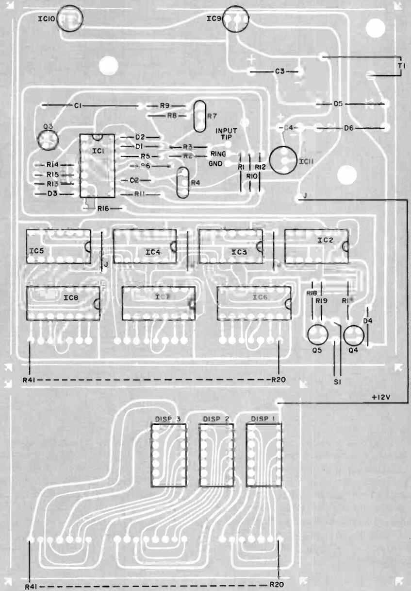
Fig. 5. The large foil pattern (opposite) is for the electronic circuit, while the smaller board below it is for the display. The two boards are interconnected by the current limiting resistors. Installation of these and other components is shown above.
