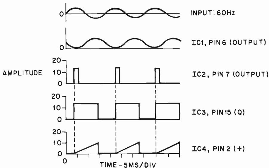
Fig. 3. Representative waveforms to be used in troubleshooting, with  $S1$  on  $X1$ ,  $S2$  open,  $S3$  on  $+$ ,  $S4$  on  $NORMAL$ ,  $R7$  three-quarters  $CCW$  and the timing capacitor selected for  $1\text{ ms/div}$ .
