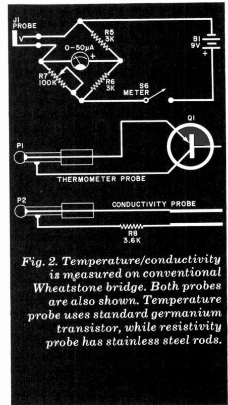
*Fig. 2. Temperature/conductivity is measured on conventional Wheatstone bridge. Both probes are also shown. Temperature probe uses standard germanium transistor, while resistivity probe has stainless steel rods.*
