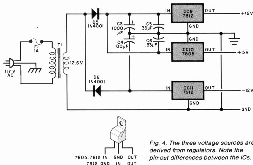
Fig. 4. The three voltage sources are derived from regulators. Note the pin-out differences between the ICs.
