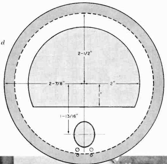
Fig. 5. Use a coping or sabre saw to cut out the form drawn on disc in Fig. 4.
