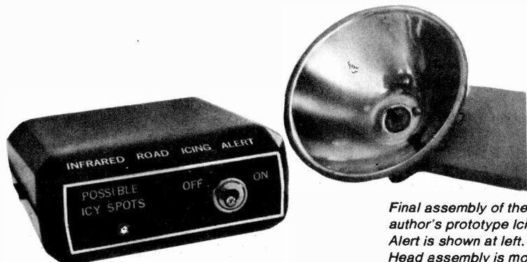
Final assembly of the author's prototype Icing Alert is shown at left. Head assembly is mounted on piece of wood with the thermistor at the focal point.
