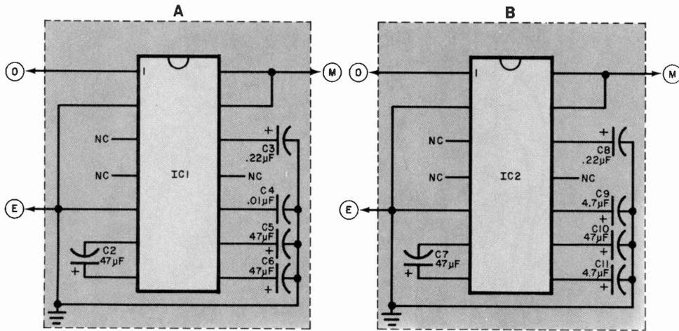
Fig. 11. Wiring diagrams for motion sensor (at far left) and special lightning sensor (left).
