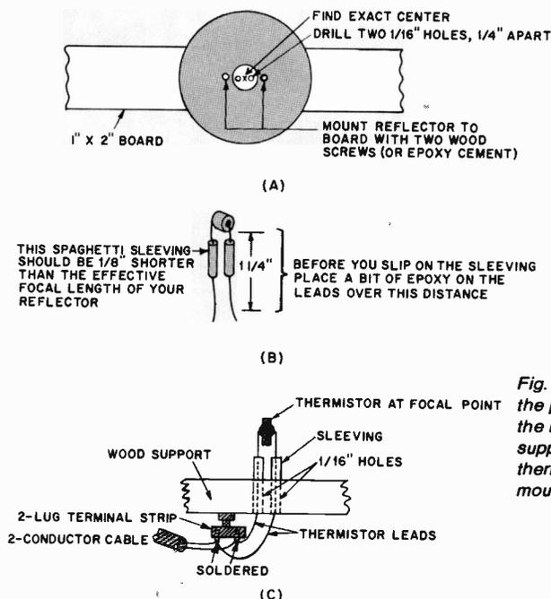
Fig. 3. Diagrams showing the procedures for mounting the reflector on its support (A), preparing the thermistor (B), and mounting the thermistor (C).
