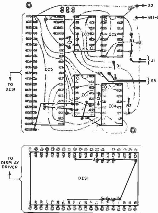
Fig. 3. Component layout for the printed circuit board is at right.
