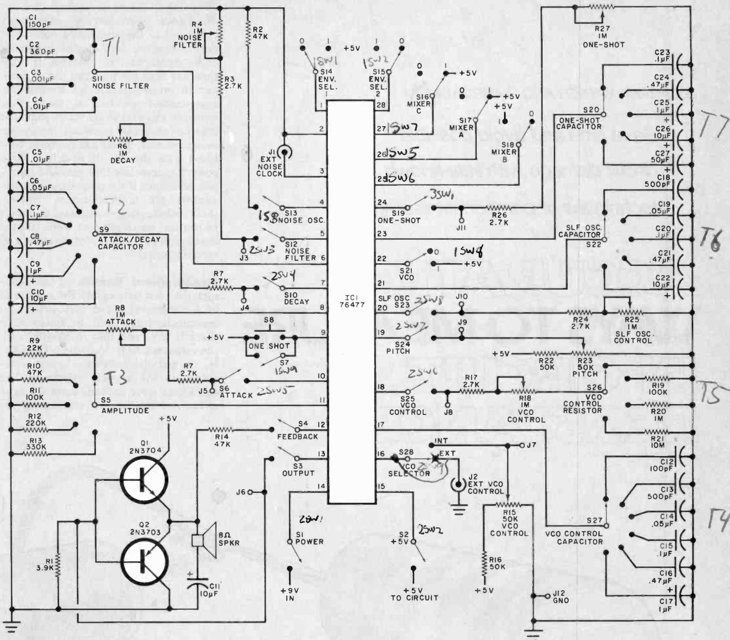
Fig. 3. The circuit for a complete sound-effects generator uses 28 switches, 12 banana (or tip) jacks and eight potentiometers to allow a broad selection of controllable parameters.
