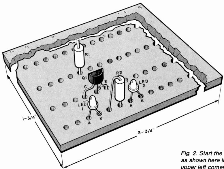
Fig. 2. Start the assembly as shown here in the upper left corner of board.
