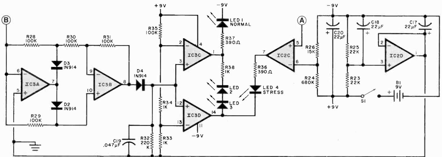
Fig. 5. The 8-to-12-Hz signals are rectified in *IC3A* and *IC3B*, integrated in *C19* and used to turn on a comparator (*IC3C*, *IC3D*) that causes the LED (s) to glow. *IC2C* shuts down the LEDs when there is no 20-Hz signal, while *IC2D* creates a bipolar supply from a single 9-volt battery.
