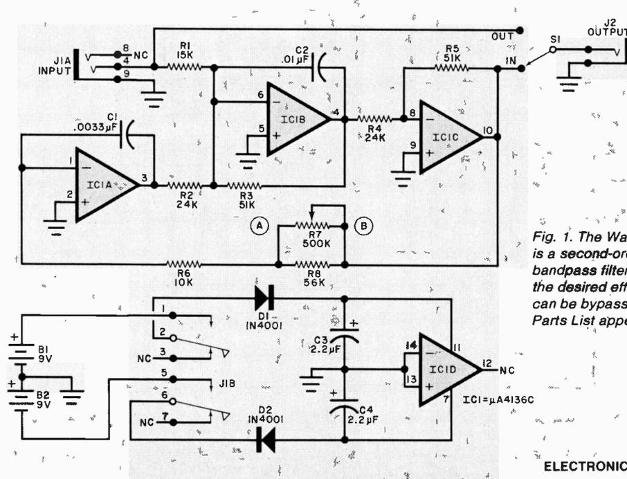
Fig. 1. The Wah-Wah Pedal circuit is a second-order, two-pole active bandpass filter that provides the desired effect. The filter can be bypassed by means of *S1*. Parts List appears on next page.
