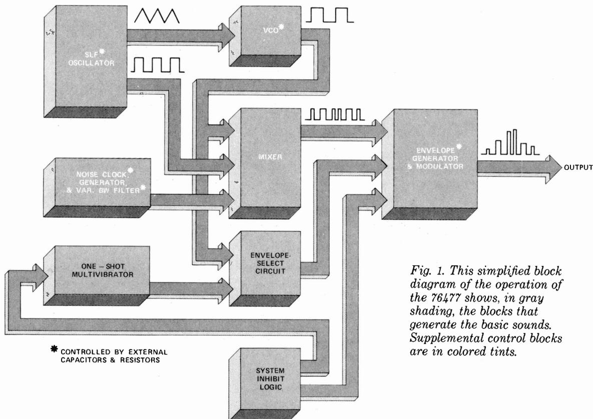
Fig. 1. This simplified block diagram of the operation of the 76477 shows, in gray shading, the blocks that generate the basic sounds. Supplemental control blocks are in colored tints.
