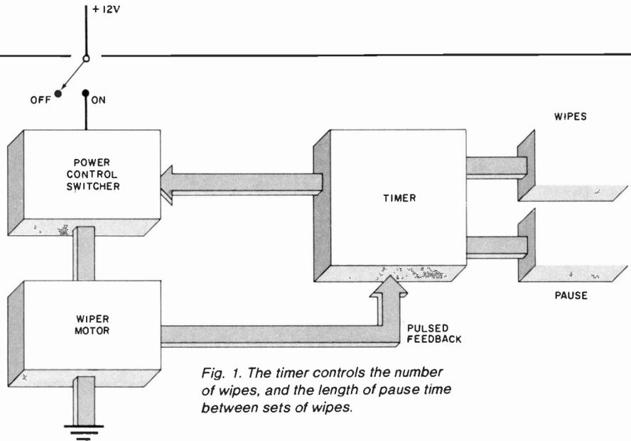
Fig. 1. The timer controls the number of wipes, and the length of pause time between sets of wipes.
