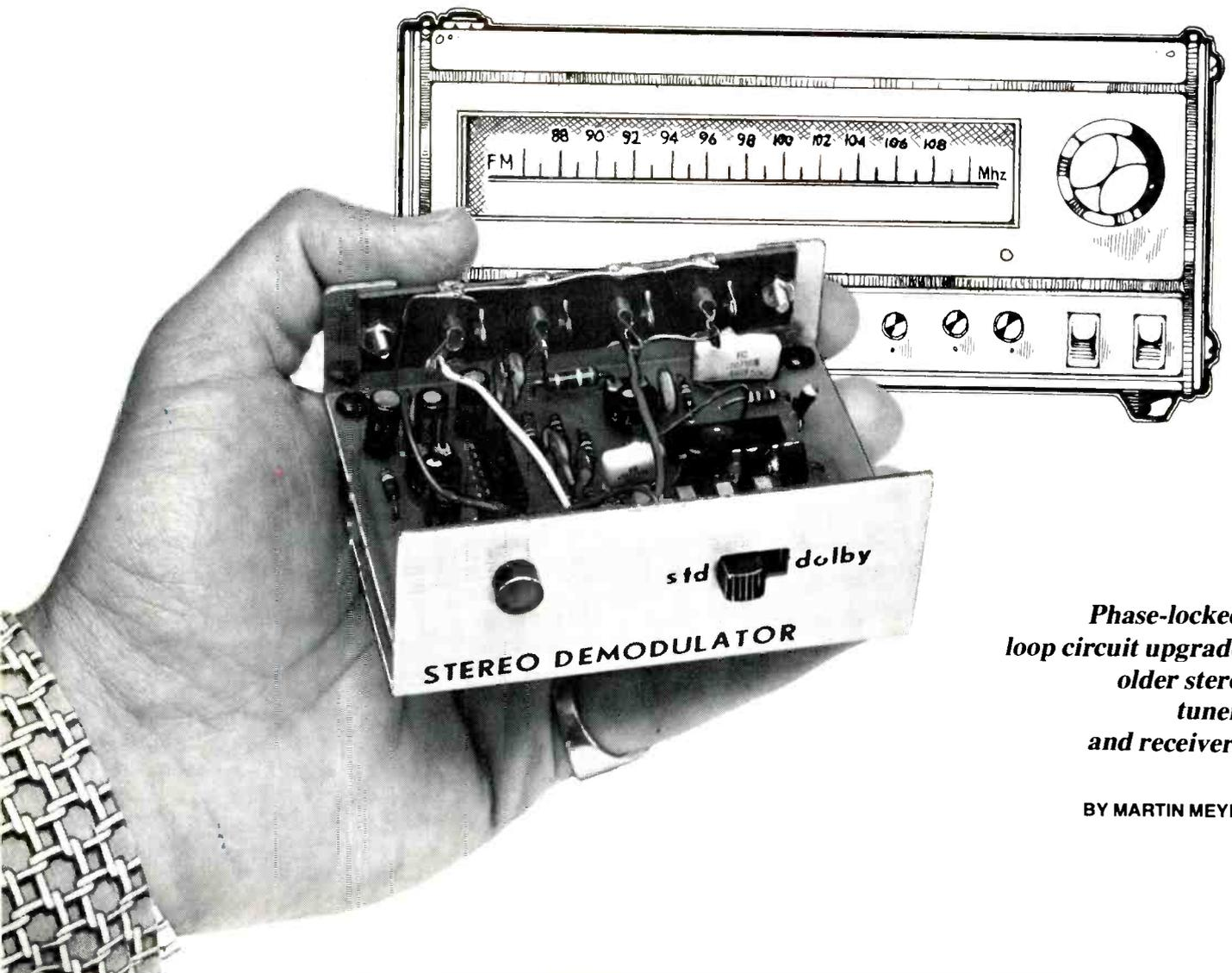
*Phase-locked-loop circuit upgrades older stereo tuners and receivers.*
