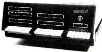
shielded, terminated motherboard; front-panel has address and data breakpoints, slow step, automatic stop, test points and internal diagnostics, binary LED indicators for address and data busses, status byte, programmed output and command status, power supply delivers 25 A @ 8 V, ± 15 V @ 5 A, all lines separately fused; IEEE-standard S-100 bus; supplied less memory, but with 1K PROM (2708) socket on MPU board ..... \$1145
