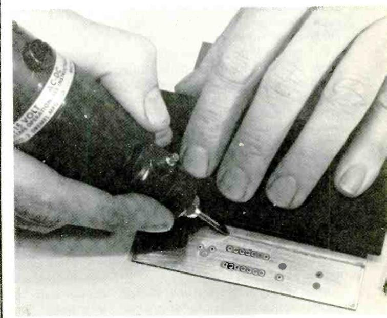
reduce the chance of ground loops that create circuit instabilities. Low-cost solder pin insertion tools permit you to install pins safely and speedily.
