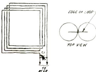
Fig. 1. Loop acts as an LC parallel circuit.
