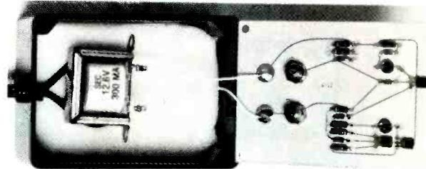
Fig. 2. Pc board can be used as case cover with component mounting as shown at left.
