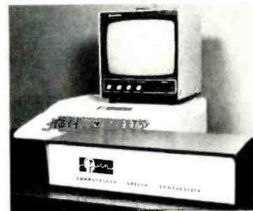
acoustic-phonetic parameters transmitted at 900 bytes/second. Two operating modes: precoded vocabulary for higher speech quality and optional CSR1 phoneme-conversion software for simpler operation. Data tapes and CTEDIT parameter editor included.
