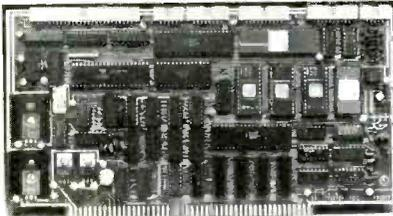
as central processor in an S-100 system. (See Module Boards.)
