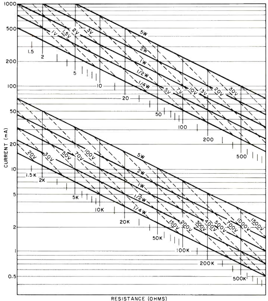
current as well as the minimum resistance required for a given voltage drop to be applied safely across it. In addition, the nomograph tells what the wattage rating for a given resistor should be, given the voltage and current.
