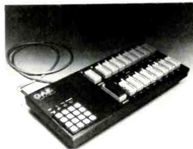
alarm, or poorly erased EPROMs, programs up to 16 PROMs at the same time, verifies all EPROMs in the matrix with the master, allows data to be added to pre-programmed parts (overprogramming). Using personality module for each generic family, the 8048 based programmer and hefty power supply will support a second duplicator for burning 32 PROMs at a time
