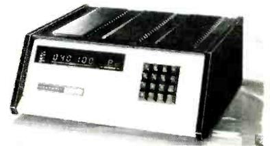
with octal keypad and digital display. With 10-slot cabinet using Heath 50-pin bus; power supply capable of handling up to 32K of memory and two I/O interfaces; programmable speaker and LED status lights. Kit, with wired and tested CPU; BASIC, assembler, editor and debug programs on audio cassette. Requires H8-1 memory board (see Module Boards) to operate. Kit .....
