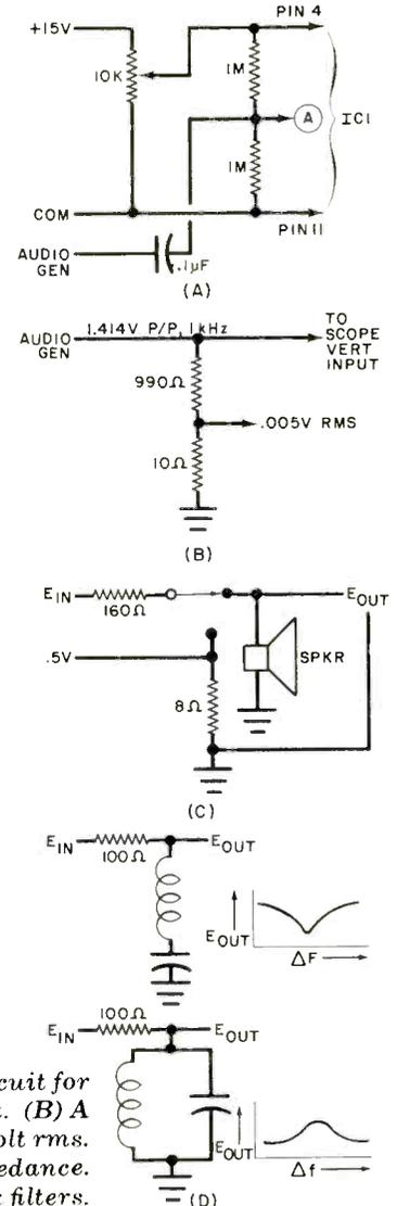
Fig. 2. (A) Test circuit for stage-by-stage checkout. (B) A source of 0.005-volt rms. (C) Measuring speaker impedance. (D) How to check filters.
