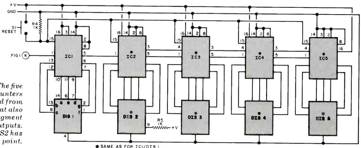
Fig. 2. The five decade counters are formed from IC's that also include 7-segment decoded outputs. Note that DIS2 has the decimal point.
