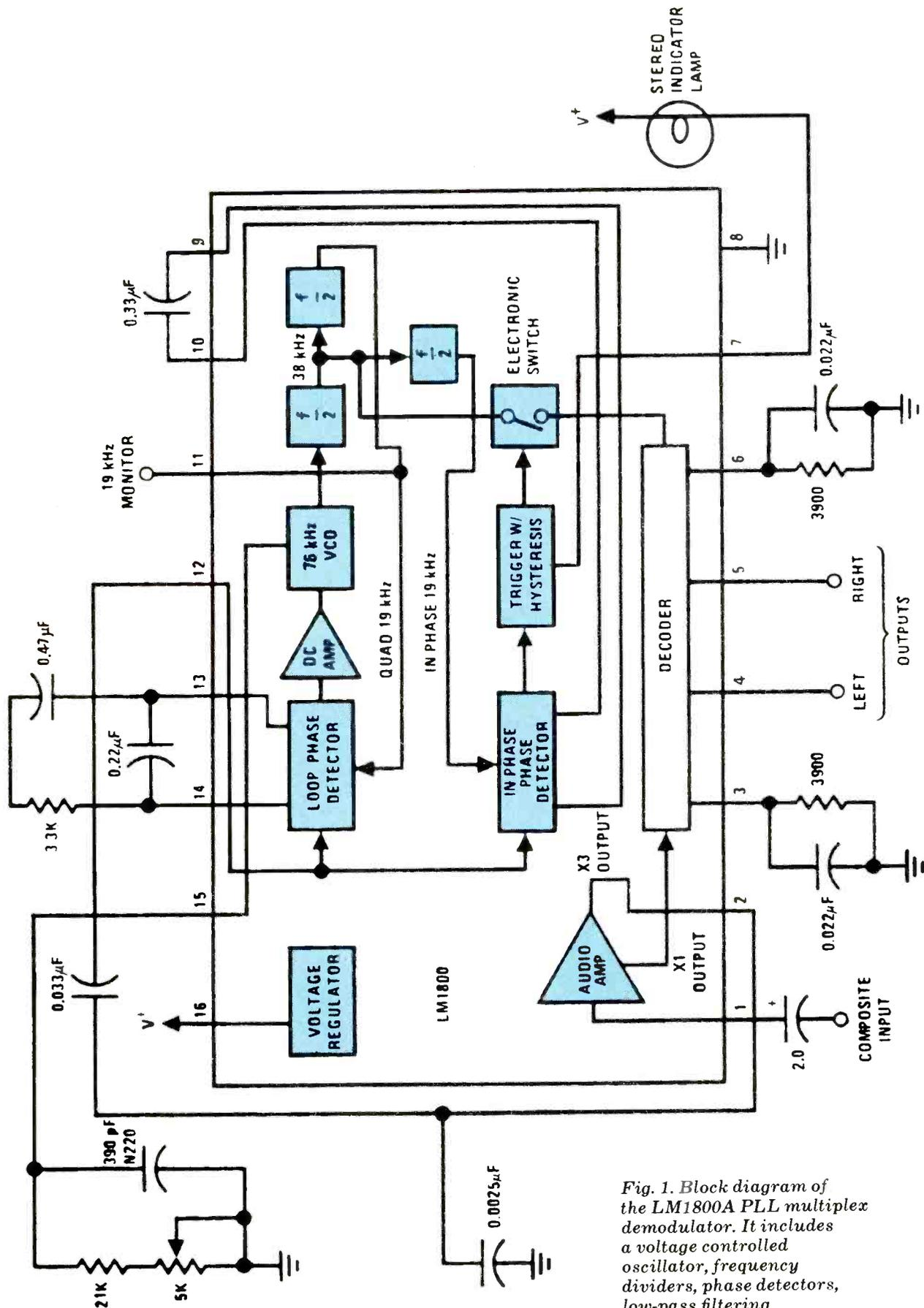
Fig. 1. Block diagram of the LM1800A PLL multiplex demodulator. It includes a voltage controlled oscillator, frequency dividers, phase detectors, low-pass filtering and error amplifier.
