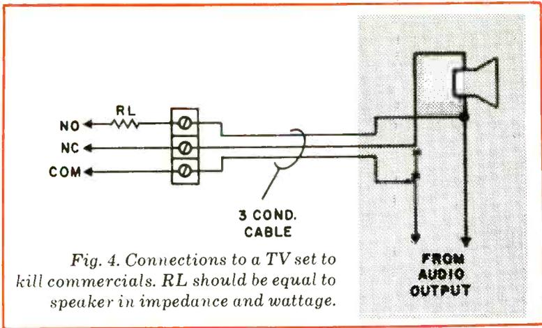
Fig. 4. Connections to a TV set to kill commercials. RL should be equal to speaker in impedance and wattage.
