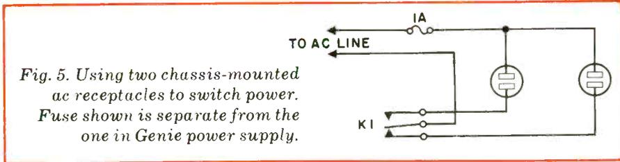
Fig. 5. Using two chassis-mounted ac receptacles to switch power. Fuse shown is separate from the one in Genie power supply.
