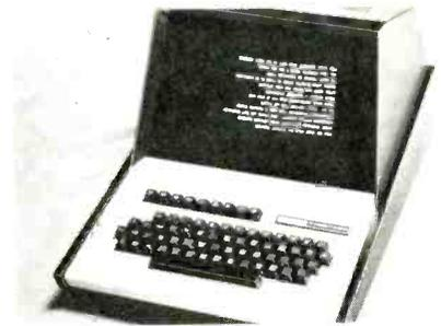
acters; cursor control; batch transmit, plot mode; 110-9600 baud; serial RS-232, 20 mA, and TTL interfaces. Kit ..... \$479
