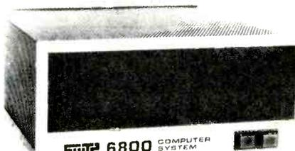
with 4K bytes of eight-bit static RAM; serial 20-mA TTY/RS-232 interface card; power supply; crystal-
