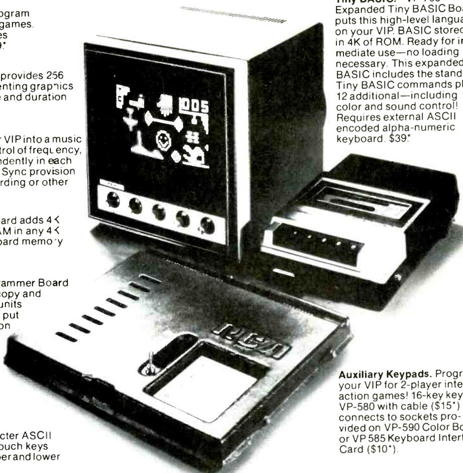
**Auxiliary Keypads.** Program your VIP for 2-player interaction games! 16-key keypad VP-580 with cable (\$15\*) connects to sockets provided on VP-590 Color Board or VP 585 Keyboard Interface Card (\$10\*).
