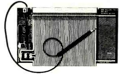
rent-measurement and for fusing of board under test; edge-connectors with formed leads for easy scope probe attachment; all connector lines labelled. S-100 version also has TTL logic probe indicating low- and high-level logic and pulses on seven-segment LED display; pulse-catcher LED whose brightness corresponds to pulse-stream duty cycle; "kluge board" section with holes on 0.1-in grid for user circuits.
