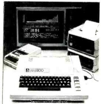
video as well as r-f output; power indicator/low-voltage light; two externally accessible cartridge slots for rapid program loading, four internal for user-replaceable memory cartridges; serial I/O; includes 410 cassette unit; 8K RAM, expandable to 48K, 8K internal ROM plus 8K BASIC in ROM cartridge
