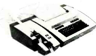
character burst buffer, caps lock, control keys; friction feed prints to 72 or 80 char/line at 10 char/in, six li/in, on std. 8 1/2-in roll paper; pin feed also prints to 132 char/line at 13 char/in, on 12-in paper, with up to five carbons; nine-wired matrix print-head; prints full 94-char. ASCII upper/lower-case set, plus parity error symbol; paper alarm; last character visible.
