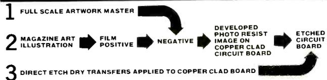
Copy circuits right from a magazine using special photo film. No camera or darkroom used. Page is not destroyed in process.
