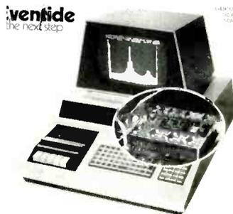
nal level. Mode 1s for Pet, Radio Shack TRS-80, and Apple II; vertical resolution varies with computer (e.g., 144 vertical elements for PET, for 7-mV resolution with 1 V input signal); input impedance 10k, unbal.; programmable in BASIC; modifiable to display 32 channels of absolute level indication, for multi-channel audio use; accommodates 2K ROM ..... \$595
