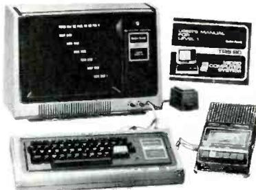
Level 1 BASIC with string variables, video graphics and cassette save and load; 4K RAM; internally expandable to 12K ROM plus 16K RAM, total memory capability 62K; includes cassette I/O and video output interfaces; TRS-80 expansion bus for future peripherals; has cursor control, automatic scrolling and rebout \$400
