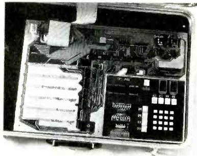
RAM, 8K EPROM; console board includes hex keypad and display, plus indicators, six I/O slots
