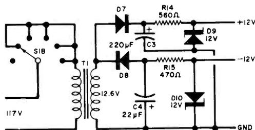
Fig. 2. Power supply delivers sufficient current for meter.
