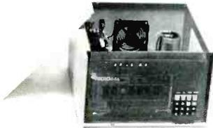
to 64K; 25-A power supply; ROM monitor, editor, and I/O; TTY/RS-232 and Kansas-City-standard cassette interfaces. In fan-cooled cabinet with 13-slot motherboard (also accepts Motorola EXORCisor cards). Available with extra I/O and bus connections at front panel. M68b. Wired ..... \$1915
