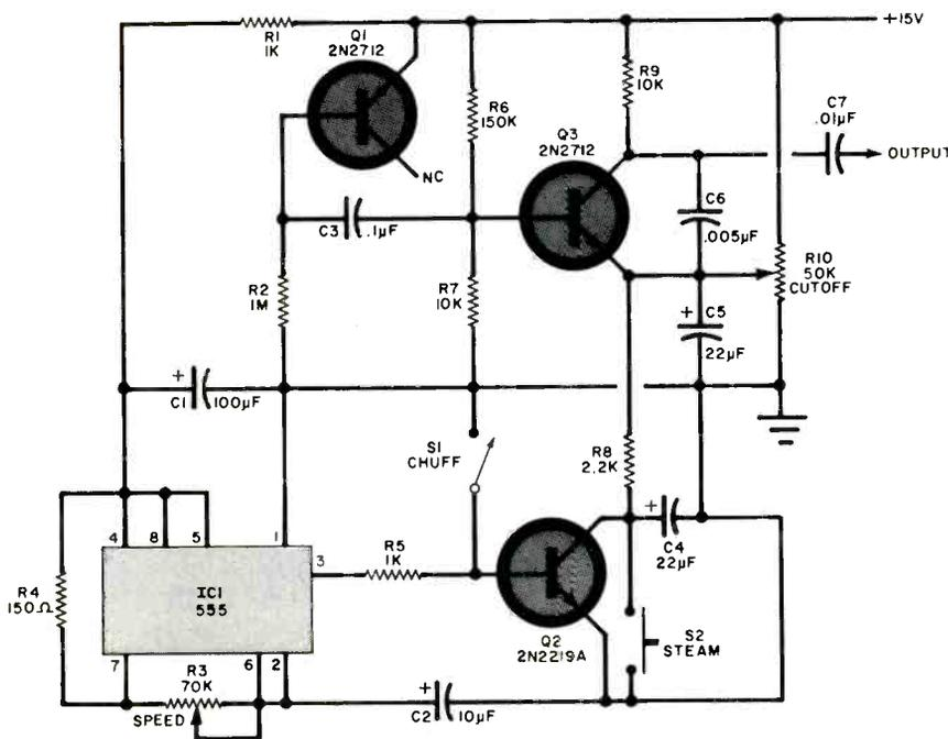
Fig. 2. Steam sound comes from white-noise generator *Q1*.
