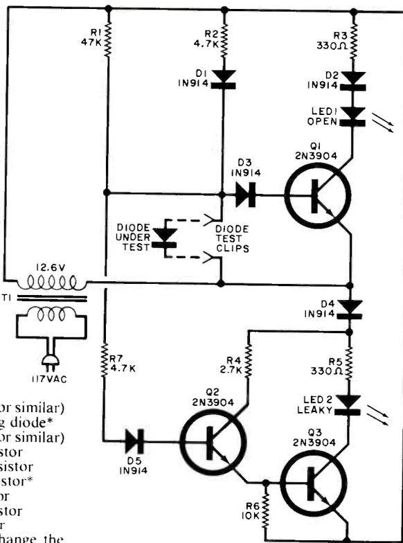
tional 12-volt transformer, no dc supply is required and all switching is performed automatically at 60 Hz.
