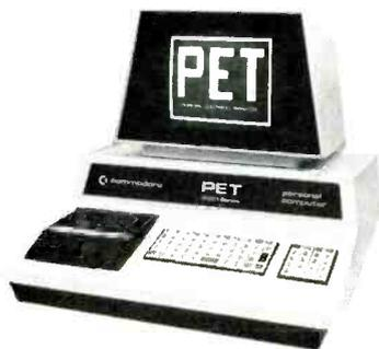
play for graphics, 40-character X 25-line alphanumeric or both; 8K RAM memory, expandable to 32K; 12K ROM including 8K BASIC interpreter and 4K operating system, built-in audio-cassette recorder (file management system in BASIC); interfaces for additional recorder and IEEE-488 instrument interface bus. Wired.
