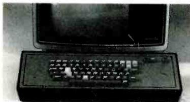
17K PROM with sockets for additional firmware, supplied with extended disk BASIC in ROM, file control system, and terminal software designed for up to 512 ports; 128 X 128 pixel graphics; vector plotting; upper-case alphanumerics plus 64 graphic characters; RS-232 interface; terminal-mode software supplied; disk capacity 51.2K/disk side (formatted); both sides of disk usable by flipping disk over. Wired.
