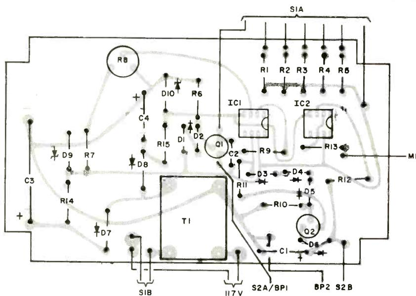
basic accuracy of the meter movement used and the accuracy of resistors  $R1$  through  $R5$ . In most cases, the meter accuracy will be 3%, and experience has shown that, with 5% tolerance resistors, the overall accuracy is about 3%. Although this may sound strange, it is due to the fact that most 5% resistors made by the same company tend to be off tolerance by the same percentage, thus reducing the effective percent error between the resistors. Using 10% resistors yields about 6% accuracy.
