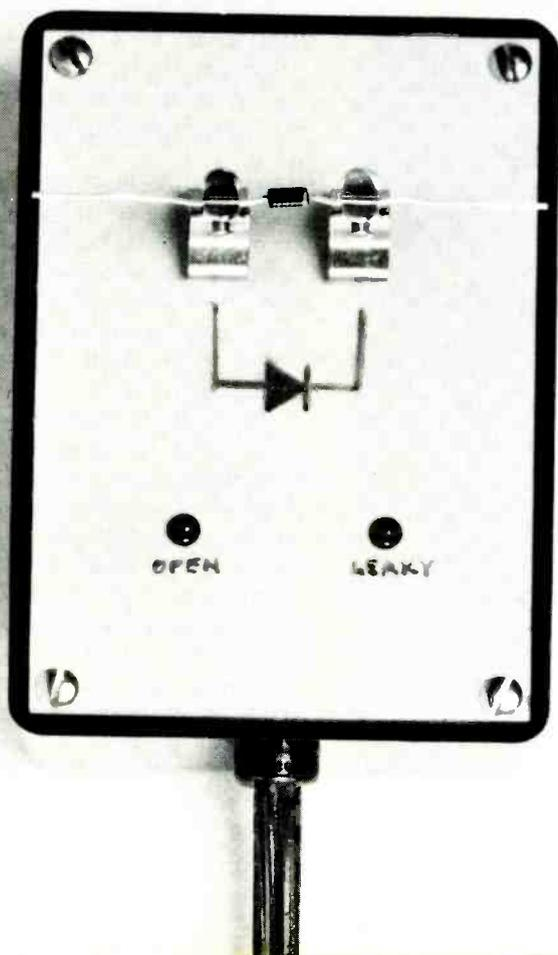
**M**OST EXPERIMENTERS think that using an ohmmeter is the best way to test a semiconductor diode. However, some ohmmeters supply too much current to the device, causing an "open" where one does not really exist. Other meters indicate values of forward and reverse resistance, which hopefully give an indication of the diode's condition.
