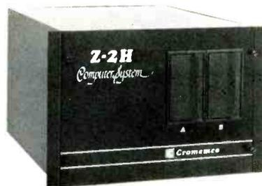
slot motherboard (5 slots occupied); 64K RAM, expandable to 512K; PRI printer interface; includes CDOS for hard and floppy disks. Wired .....\$9995
