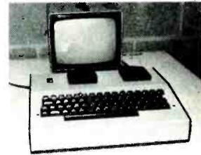
16-line display; 110-9600 baud; half or full duplex; auto carriage return/line feed; automatic rollup; available with built-in acoustic coupler.
