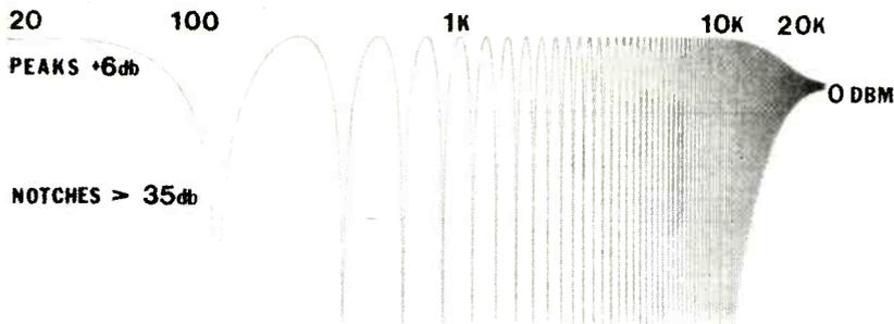
Fig. 1. Frequency between notches on a comb filter is adjusted by varying the clock frequency.
