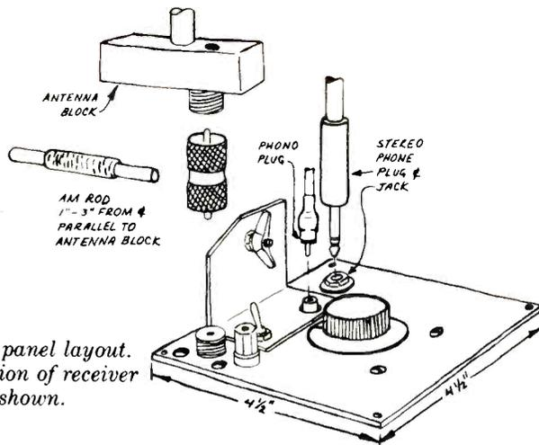
Fig. 4. Control panel layout. Proper orientation of receiver rod antenna is shown.
