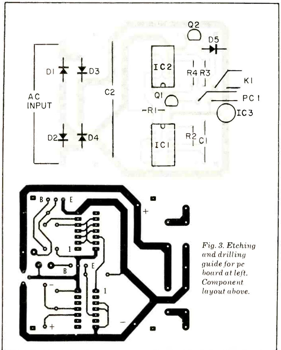
Fig. 3. Etching and drilling guide for pc board at left. Component layout above.
