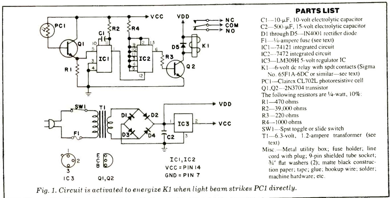
Fig. 1. Circuit is activated to energize K1 when light beam strikes PC1 directly.
