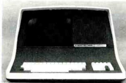
keyboard plus 18-key numeric pad; cursor addressing; automatic repeat on all keys; shiftlock, backspace; graphics mode; programmable white-on-black or reverse display; self-test mode; editing features include char and line insert/delete, full/partial block transmit, line-end terminators, protected fields; generates all 128 ASCII characters; blinking, reverse and half-intensity; 12-in CRT; RS-232 standard, 20 mA avail.; aux. printer port with local print mode; export models available .....\$995
