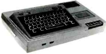
output to conventional TV; power supply. Color output on TV channel 3, r-f switchbox included; audio software and hardware includes three-octave music synthesizer, tape generation. Cassette interfaces up to 2000 byte/sec, can output sound from tape. Keyboard 53-key, typewriter-layout. Includes joystick X-Y controls. Software available includes BASIC, calculator, data management, mailing list, account ledger, music, educational and games. With 2 programs ..... \$500
