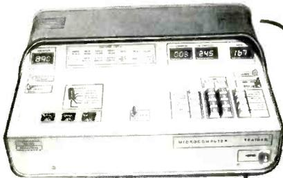
ports; displays in octal for hi and lo address, data and counter; octal keypad; function keys as switches; 256 byte executive program in EPROM. \$900
