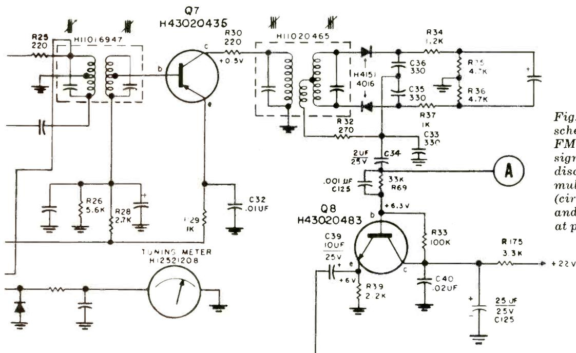
Fig. 4. Partial schematic of typical FM receiver. Composite signal is obtained by disconnecting existing multiplex decoder (circuit below *C34*) and tapping signal at point A.
