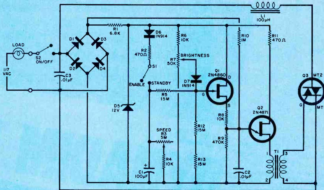
Fig. 1. Unlike a conventional light dimmer, the triac (Q3) is gated later and later in the power-line cycle as C1 discharges. Dimming time is controlled by varying discharge time to C1
