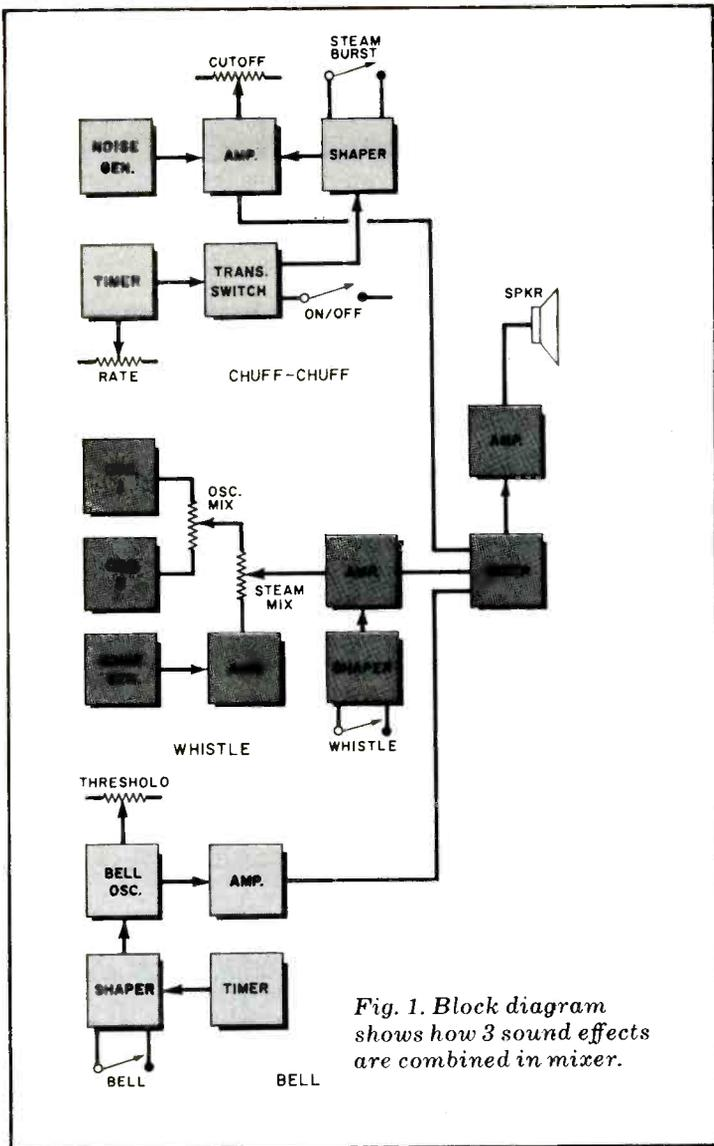
Fig. 1. Block diagram shows how 3 sound effects are combined in mixer.
