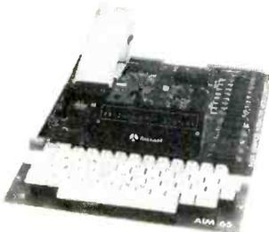
dot matrix printer, separate 54-key terminal-style keyboard. Includes: dual cassette and TTY interfaces; 8K ROM with text editor, monitor and debug sockets for 16K ROM, 1K or 4K RAM; two bi-directional 8-bit ports; expansion and I/O connectors compatible with KIM-1. Wired, 1K/4K ..... \$375/\$450
