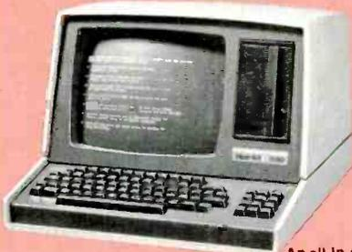
An all-in-one computer system, complete with built-in floppy disk storage
