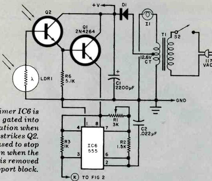
Fig. 1. Timer IC6 is gated into oscillation when light strikes Q2. LDR1 is used to stop operation when the camera is removed from support block.
