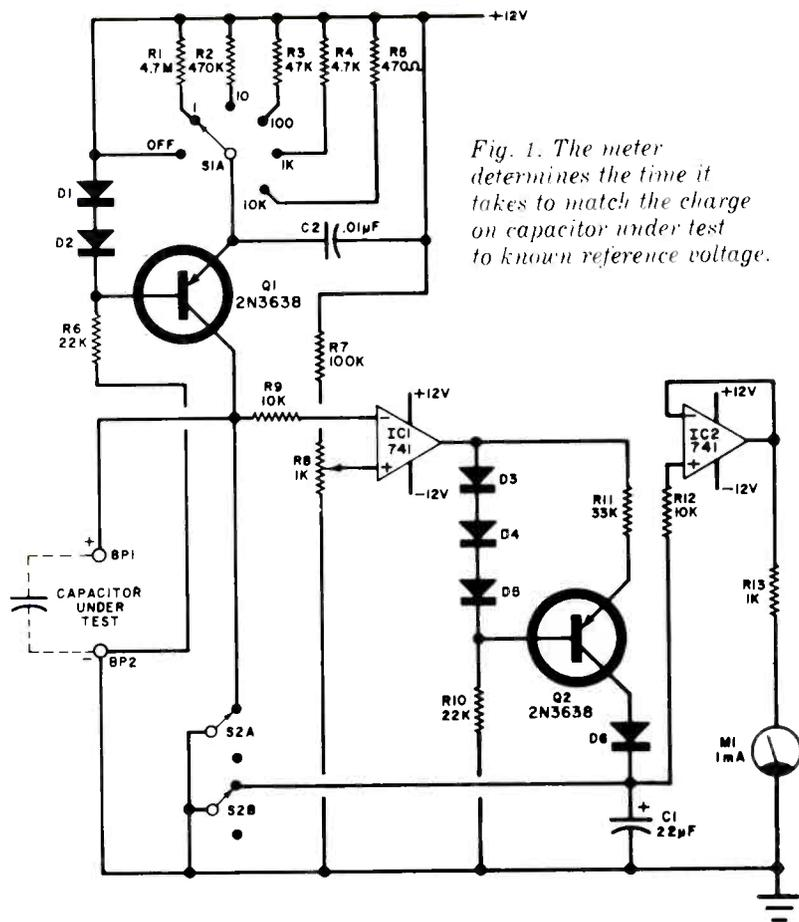
Fig. 1. The meter determines the time it takes to match the charge on capacitor under test to known reference voltage.
