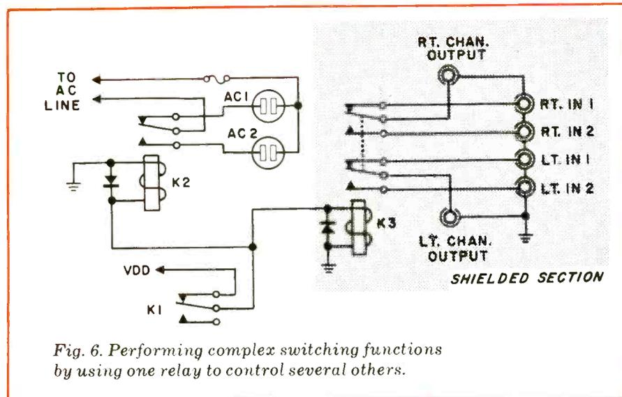
Fig. 6. Performing complex switching functions by using one relay to control several others.
