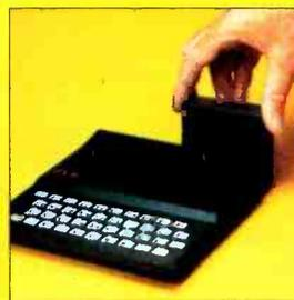
**16K MEMORY MODULE:** Like any powerful, full fledged computer, the ZX81 is expandable. Sinclair's 16K memory module plugs right onto the back of your ZX81 (or ZX80, with or without 8K BASIC). Cost is \$99.95, plus shipping and handling.
