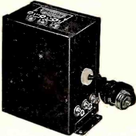
ABOVE is shown Thordarson power foundation unit for B-elimination and power amplification. It contains a power supply transformer, two filter choke coils, a center tapped filament supply, and two buffer condensers all in one compound filled case. In two types; R-171 for Raytheon tube BH and power amplifying tube UX 171, and type R-210 for UX 216-B rectifying tube and UX 210 power amplifying tube.
