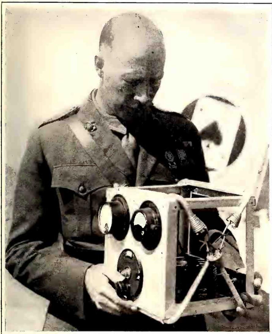
Smaller than a typewriter and weighing only 5 1-2 pounds, with a sending radius of 300 miles, a tiny transmitter has been built by United States Marine Corps aviators and installed in marine airplanes for "talking" to other pilots and to ground stations. In 50 separate tests, the little sender worked "perfectly" 47 times, and aviators said the three failures were due to factors outside the transmitter.
