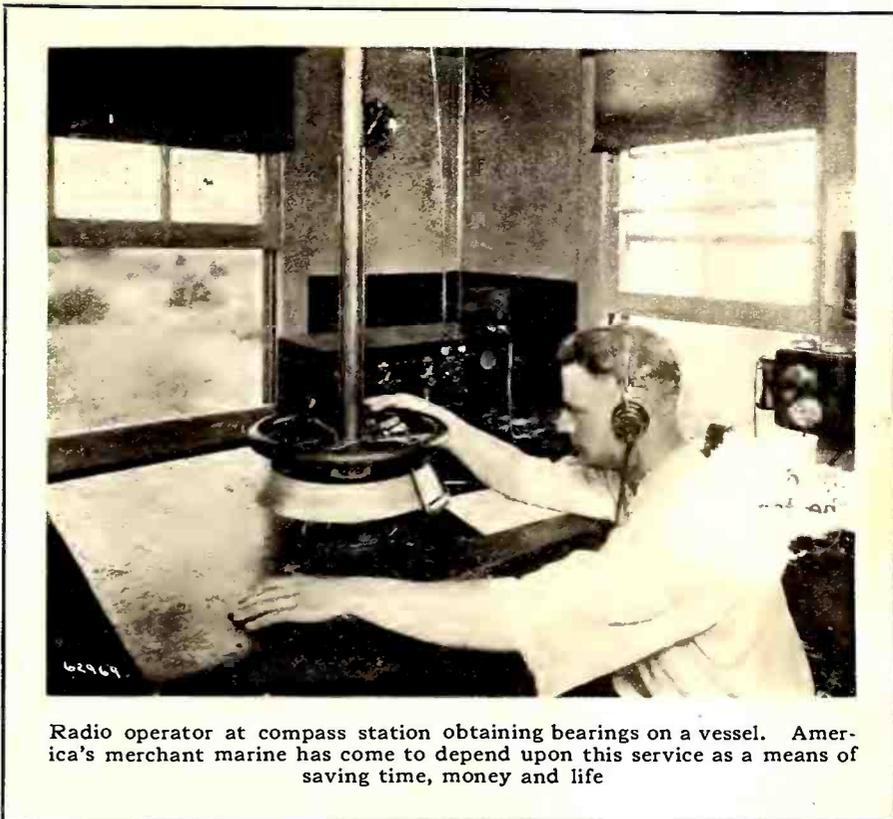
Radio operator at compass station obtaining bearings on a vessel. America's merchant marine has come to depend upon this service as a means of saving time, money and life
