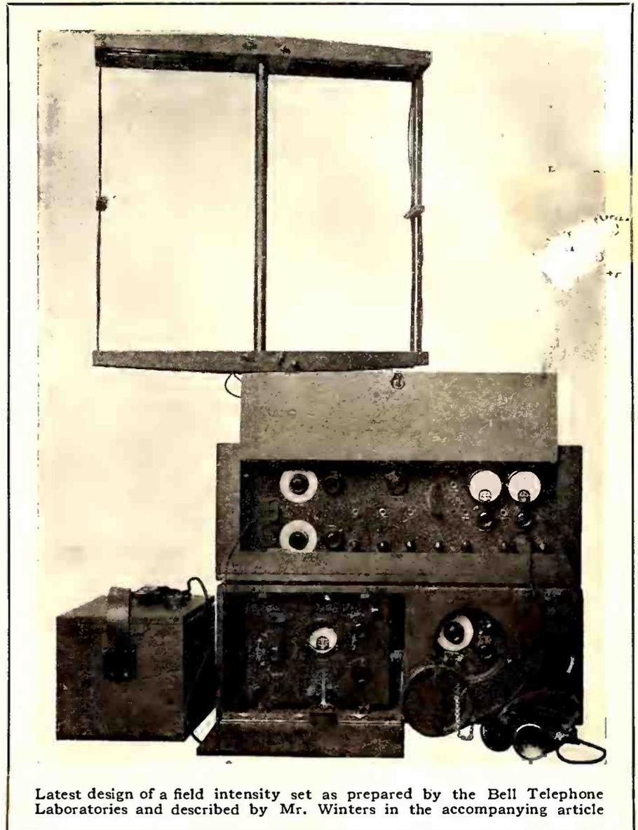
Latest design of a field intensity set as prepared by the Bell Telephone Laboratories and described by Mr. Winters in the accompanying article
