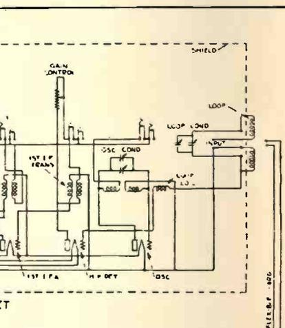
Schematic circuit of the field intensity measurement set developed by the Bell Laboratories
