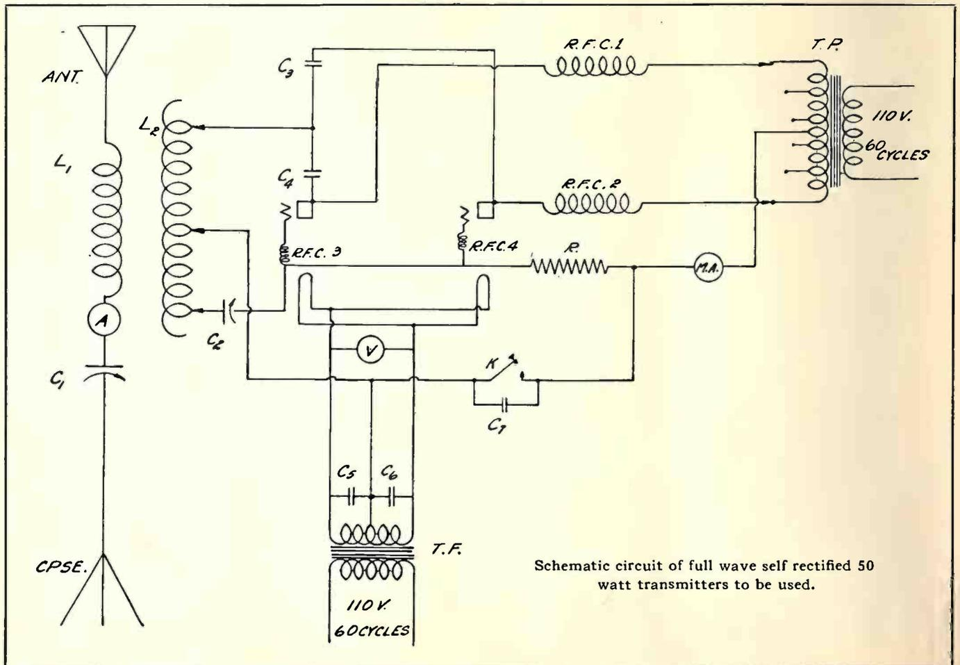
Schematic circuit of full wave self rectified 50 watt transmitters to be used.
