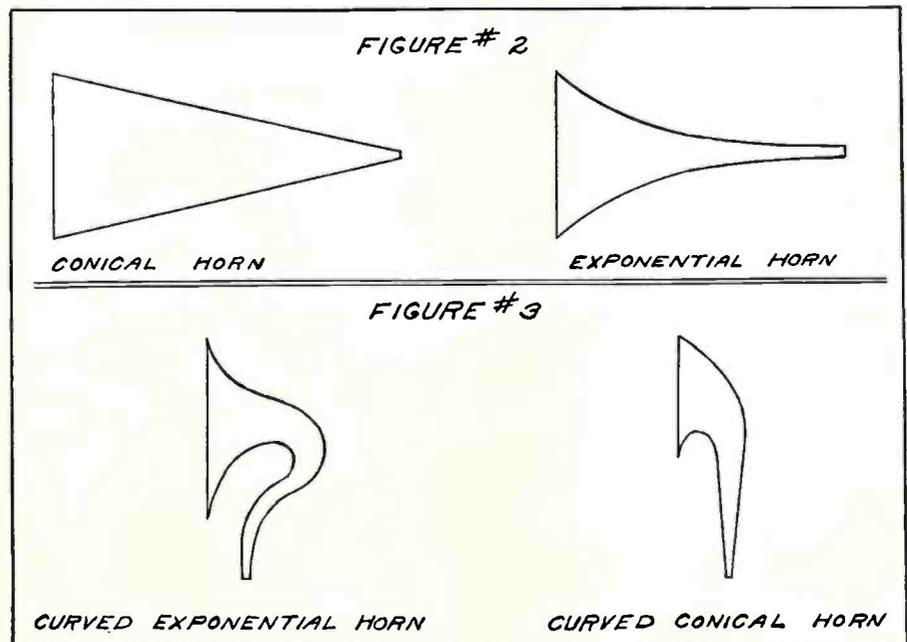
ever, alter its characteristics in any way other than to slightly improve the tone due to decreased sound reflection at this point. These types of horns may be curved into any conceivable shape without altering their general behavior provided that the turns are not too sharp. Figure No. 3 shows the two most common types of curved horns.
