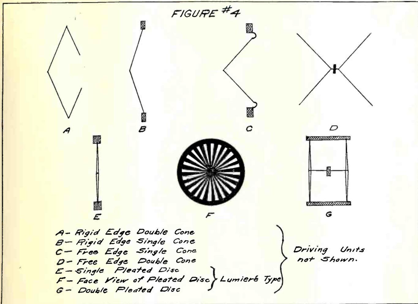
general ways. Sometimes the edge of the cone is flexibly supported by circumferential rubber or kid leather strips; sometimes it is loosely held by soft felt packing around the periphery; and in one or two makes, it is absolutely free, all support of the cone being accomplished by the driving pin, which is made proportionately stronger to bear the additional strain imposed upon it.
