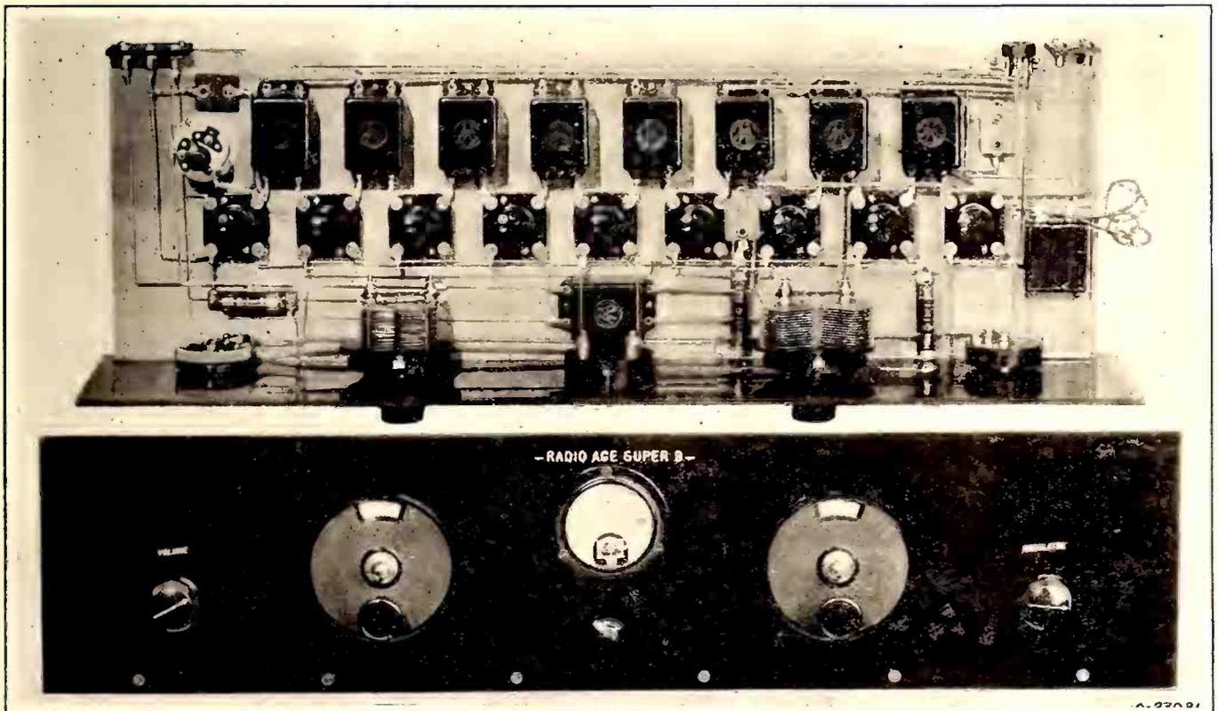
In the upper picture is shown the baseboard layout of the Radio Age Super 9. Beginning at the left of the baseboard the transformers used are as follows: H210, H210, H215, H210, H215, F320, L425, F320. The transformer shown between the two Remler condensers is an L430 RF transformer. The grid of the sixth and seventh transformer is not bridged directly to the tube socket. See the schematic for the actual electrical connections
