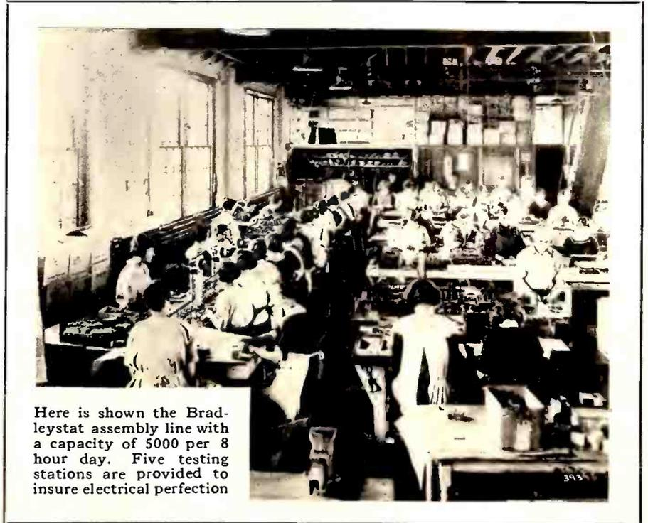
Here is shown the Bradleystat assembly line with a capacity of 5000 per 8 hour day. Five testing stations are provided to insure electrical perfection
