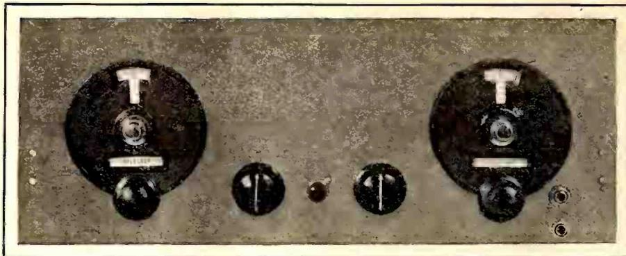
Figure 3 shows the front panel view of the seven tube portable described in this article. The number of controls has been cut to a minimum
