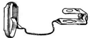
Showing contact spring and terminal with flexible connecting link, which is for current, not spring tension. The superiority of the spring contact is at once evident. It is positive but causes no undue side strain. The tube slips in place without forcing and is removed easily without sudden and unexpected release.
