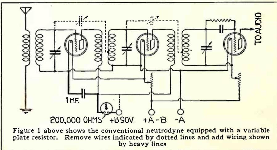
Figure 1 above shows the conventional neutrodyne equipped with a variable plate resistor. Remove wires indicated by dotted lines and add wiring shown by heavy lines
