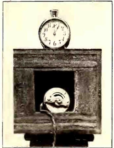
Many novel means of identifying radio stations have been hit upon but none so popular and so completely unique as the clock used by Havana to keep its wave channel alive during the program interludes
