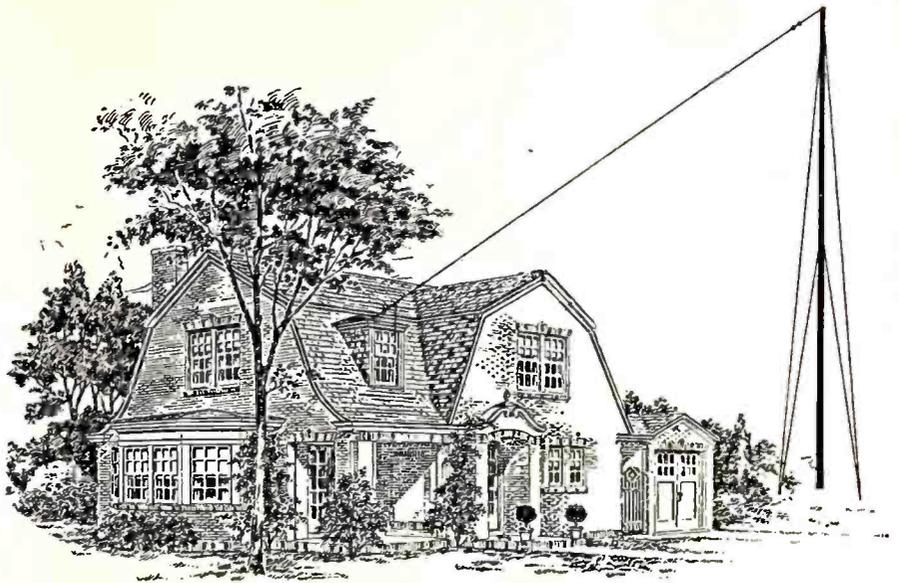
Fig. 4. Straight wire antenna for extreme simplicity
