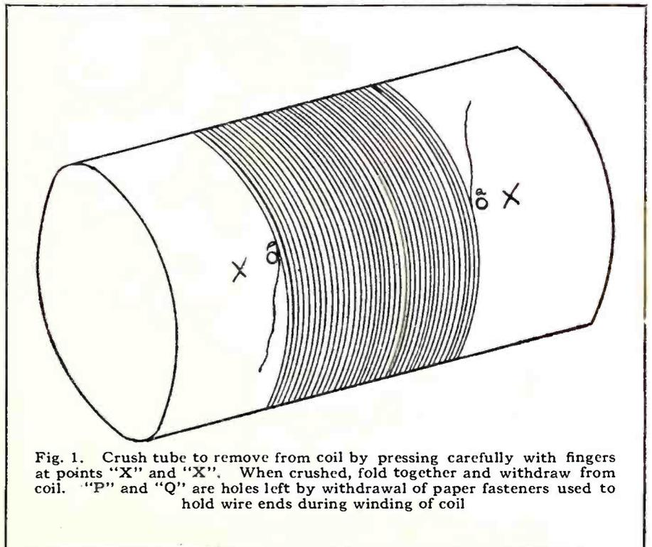
Fig. 1. Crush tube to remove from coil by pressing carefully with fingers at points "X" and "X". When crushed, fold together and withdraw from coil. "P" and "Q" are holes left by withdrawal of paper fasteners used to hold wire ends during winding of coil
