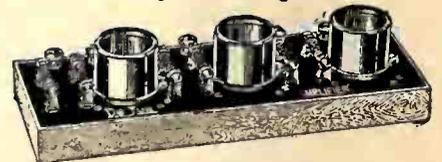
The De Jur Amplifier is a compact rigidly constructed unit to be substituted for the audio transformers thereby changing a transformer-coupled to a resistance-coupled receiver. The panel is of Bakelite and is mounted in a mahogany case which fits into the audio side of any type set.
