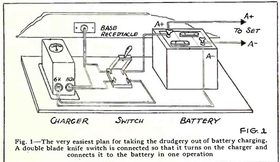
Fig. 1—The very easiest plan for taking the drudgery out of battery charging. A double blade knife switch is connected so that it turns on the charger and connects it to the battery in one operation
