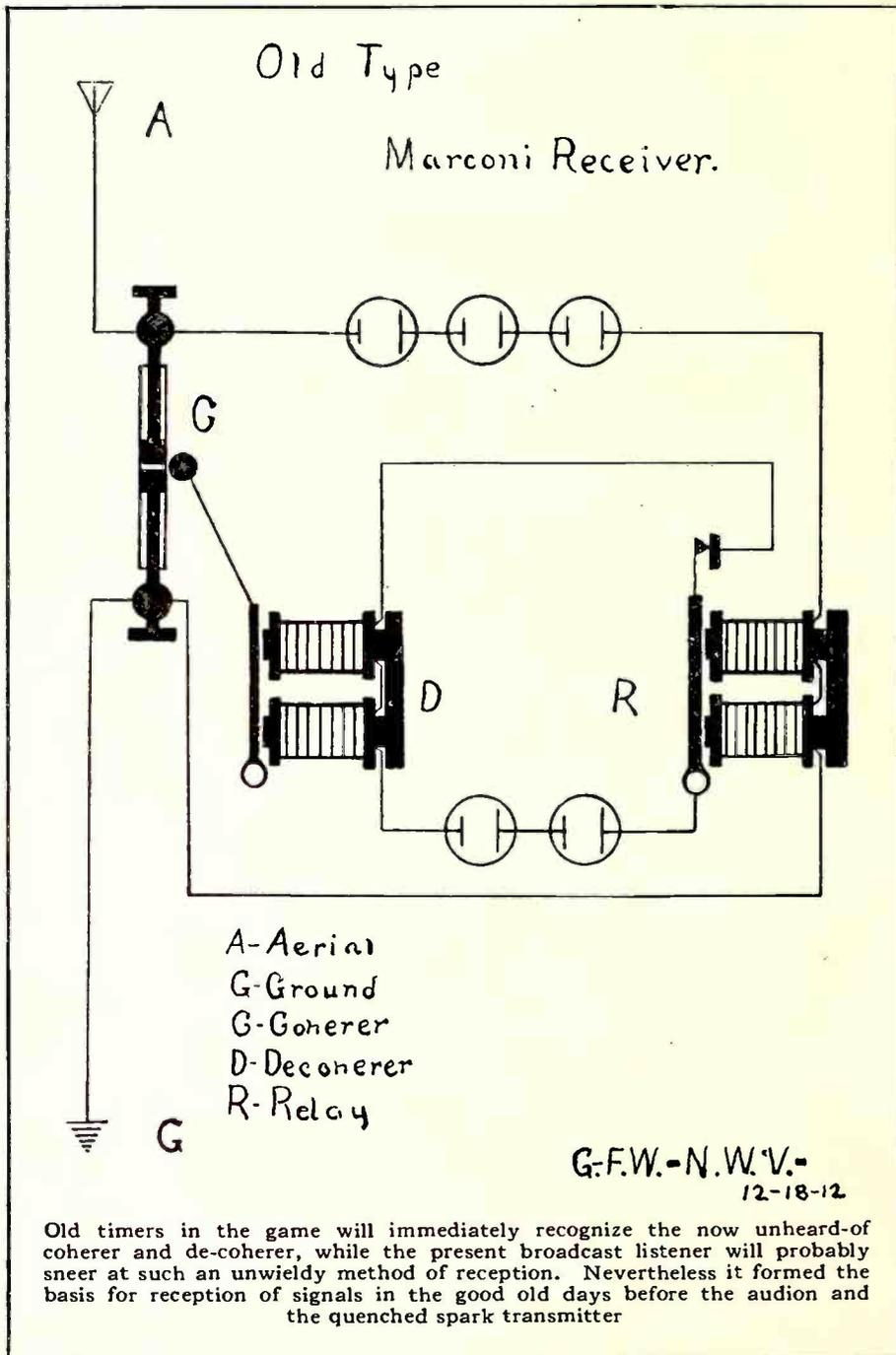
Old timers in the game will immediately recognize the now unheard-of coherer and de-coherer, while the present broadcast listener will probably sneer at such an unwieldy method of reception. Nevertheless it formed the basis for reception of signals in the good old days before the audion and the quenched spark transmitter
