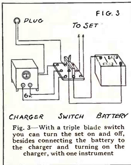
Fig. 3—With a triple blade switch you can turn the set on and off, besides connecting the battery to the charger and turning on the charger, with one instrument
