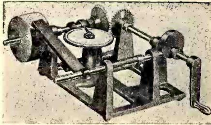
With this device, which is within the reach of any experimenter, three different widths of honeycomb coils may be wound. A turn counter is also provided to facilitate counting the windings. Half, three quarters and one inch are the widths provided for by means of removable eccentrics. The diameter of the coils may be altered by placing different sized spools on the winding spindle.
