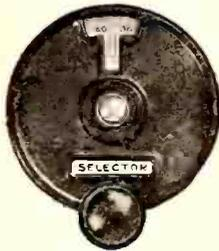
Composed of black bakelite dial housing enclosing reversible, celluloid-finished indicator plate marked off to half-degree divisions. Ratio: 14.5 to 1. Absolutely without backlash due to automatic friction take-up. Fits any condenser—left or right—half or full turn movement. Price.....\$2.50
