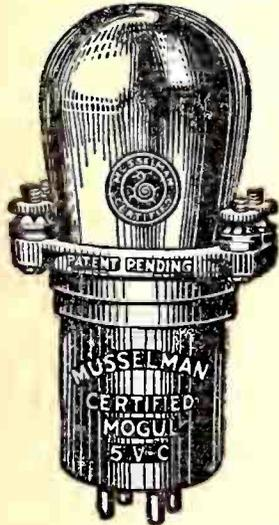
An interesting feature of the new Mogul 5V-C power amplifier tube put out by the Van Horne Co., and certified by Musselman, is an adapted base, in addition to the conventional tube base, on which are mounted four terminals for inclusion of higher B and C voltages than found in the normal sets without having to alter the wiring.
