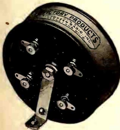
VICTOREEN intermediate transformers, handled by the George W. Walker Co., have a sharp resonance curve. This resonance feature of the coil permits use of an aperiodic primary, prevents interstage oscillation, makes the set more stable and permits the use of a potentiometer as a volume control.
