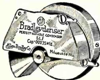
The one hole mounting makes installation easy. The plates are of brass and soldered to provide highest conductivity. Rotor plates are grounded.
