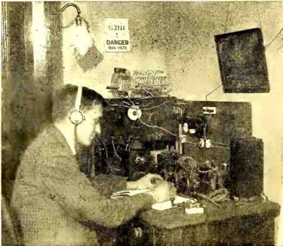
Fig. 1. The picture above shows Herbert Hiley, of the British station G21 H, situated at Keighley, Yorkshire, who has been successful in establishing communication with M. Fresni, Rua Aswaldo Cruz, Nieteroky, Brazil, a distance of 5400 miles with a wavelength of 42 meters and 15 walls in the antenna, the circuit used being a Hartley loose coupled. Mr. Hiley is shown logging a station. The photograph is by courtesy of G. Crowther, 28 Cark Road, Keighley, England.
