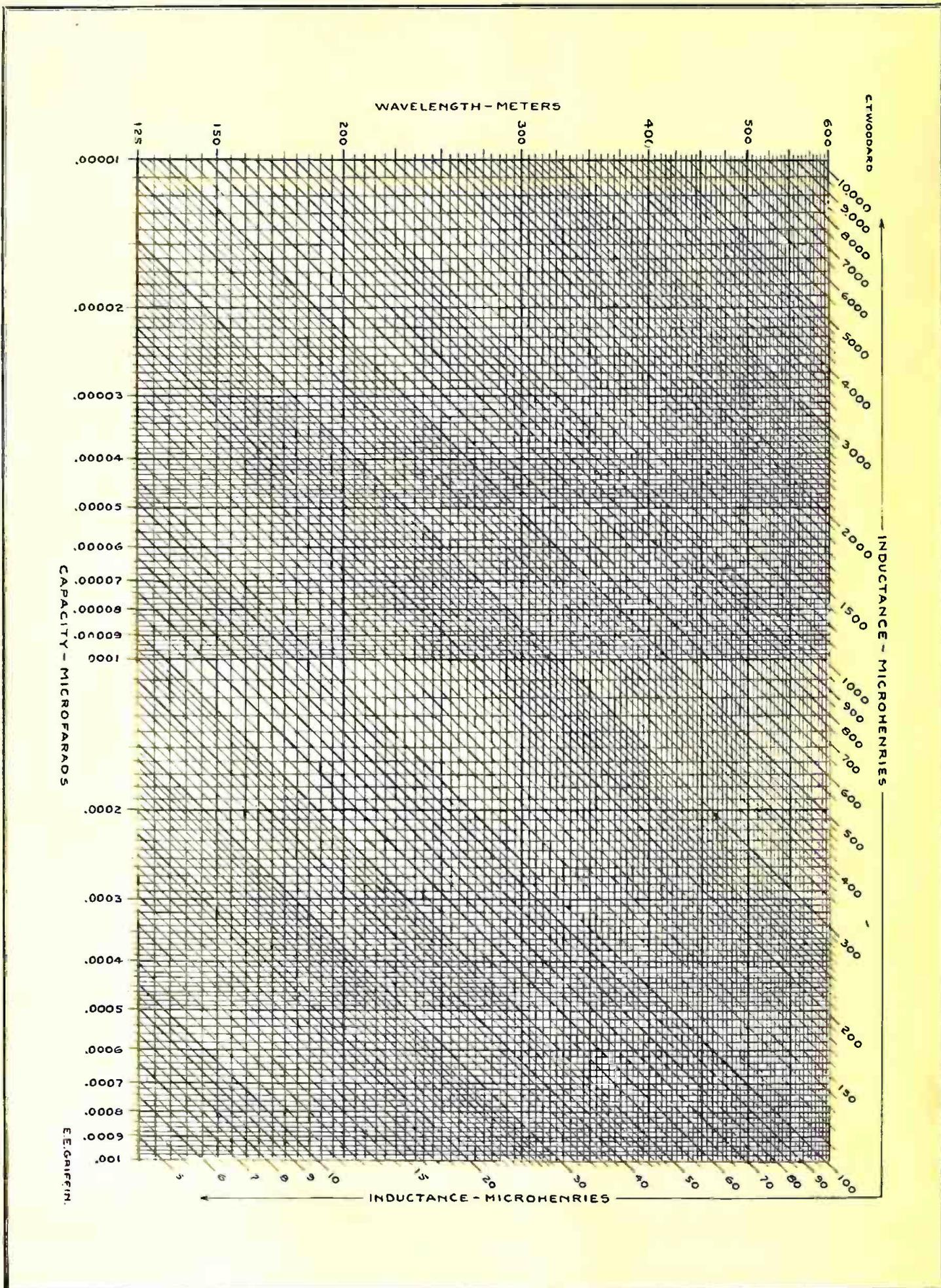
Here is the chart explained in the article on the preceding page, by which applications of the wavelength formula as applied to broadcast work may be solved with little trouble. In reading the scales, it will be advisable to interpolate between captioned lines, since the various lines in between are necessarily of varying spacing.
