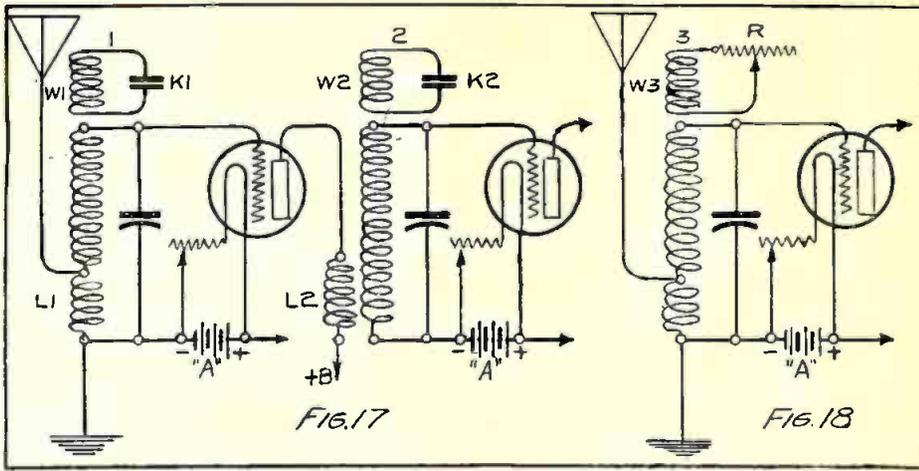
oscillations if they are not too severe, but at the same time we lose sensitivity and volume. Such resistances will vary from 5,000 to 20,000 ohms and are of the grid leak type. By connecting a small fixed condenser (K) across the resistance (R2) in the grid return we can sometimes work a decided improvement in the sensitivity. Here we have the usual coupler with the primary (L1) and secondary (L2) tuned by the variable condenser (C). This may be applied to the first or second stage or to both.
