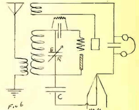
Fig. 6. The above circuit shows us the A. C. tube at its highest efficiency; it furnishes A battery current for the electronic emission and also furnishes its own B potential through the connection between the plate of the tube and the center of the 110 volt filament.
