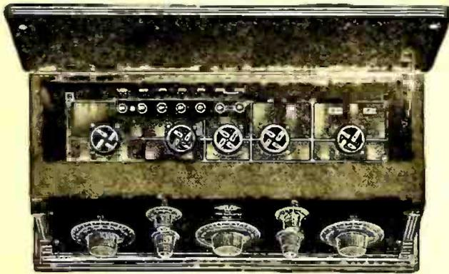
**I**N TESTING the Melco Supreme receiver we experienced a few new things, both in circuit design and use of radio apparatus. The Melco Supreme receiver is a tuned radio-frequency receiver using five tubes, and follows the usual design in such a circuit. The differences that exist are not in any way radical but they represent refinements in parts of the circuit that are important.
