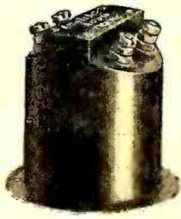
Test No. 81. Submitted by the Anylite Electric Co., at Ft. Wayne, Ind. The sample consists of an audio frequency transformer, well built and shielded, designed for use in any audio amplifier where clearness of speech and volume is desired. Tested and approved by RADIO AGE Institute.
