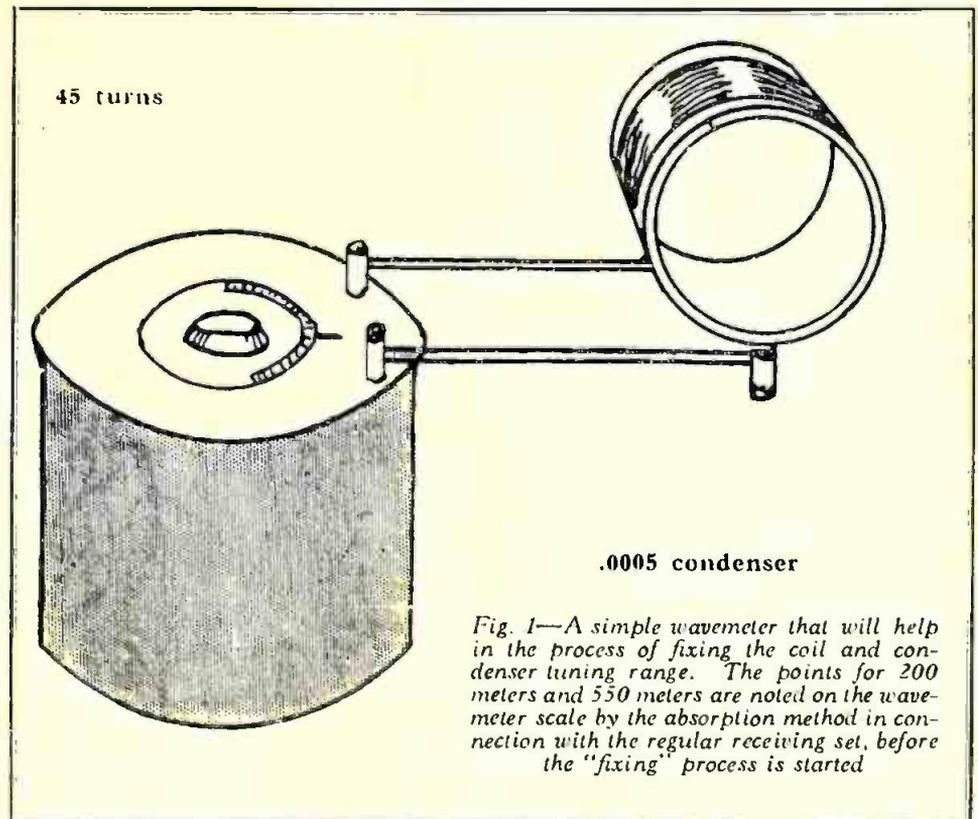
and that fewer turns of wire will be needed to place the lowest wavelength at the desired point—200 meters for broadcast reception. The effect of the tuning condenser is thus decreased; that is, a larger condenser is necessary to cover the broadcast band.
