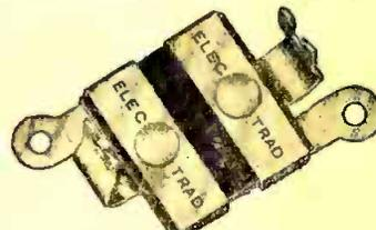
Test No. 83 submitted by the Electrad, Inc., 428 Broadway, New York. Sample consists of a grid condenser type G-S equipped with punched connecting lugs by means of which the condenser may be mounted directly to the socket. There are two prongs for the use of a cartridge resistance of a grid leak. The capacity of each condenser is stamped on the prongs. Tested and approved by the RADIO AGE Institute.
