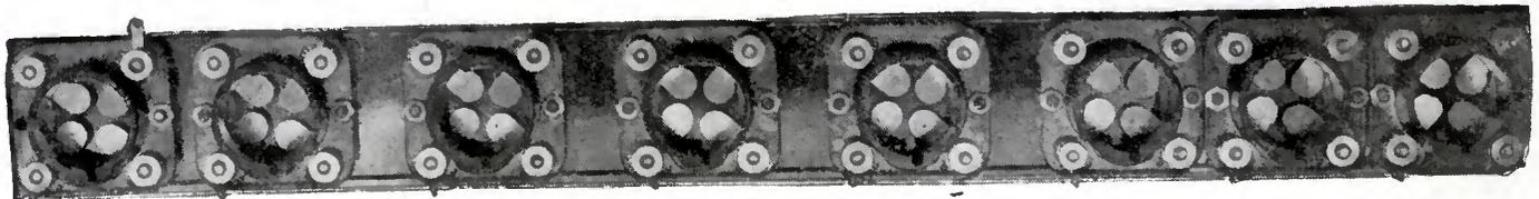
The socket strip for the simplified portable super-heterodyne, showing one filament lead and method of binding lugs for other filament lead.
