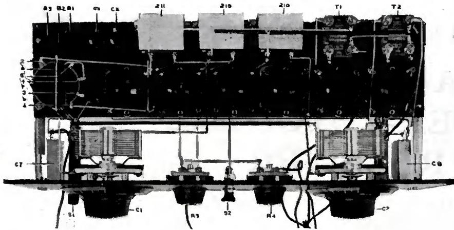
Fig. 2. Interior view of the super-autodyne. The instrument designations will be found in the text. The sockets, from left to right, are: V1, autodyne; V2, 1st R. F.; V3, 2nd R. F.; V4, 2nd Det.; V5, 1st A. F.; V6, 2nd A. F.; Socket shelves may also be procured for UV199 or C299 tubes.
