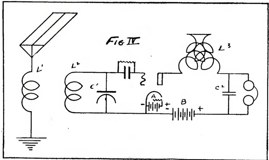
An inductively coupled Armstrong regenerative. Coils L1 and L2 are wound by the contributor, while L3 is an ordinary plate variometer. He gets good results on it, as he should with a loose coupled regenerative set.
