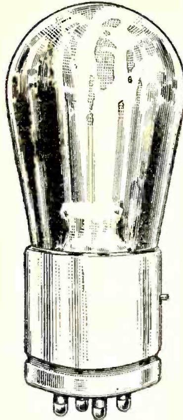
**J**UST what part the vacuum tube plays in the working of a receiving set is well known to all radio enthusiasts; at least, they know that if it is to be used as a detector tube, it must be placed in one part of the circuit and if it is to be used as an amplifier tube, it is used in a different part of the circuit.
