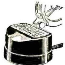
Test No. 25. PHONOGRAPHIC RELAYING DEVICE. Better known as the Dulce - Tone Phonographic Loud speaking Device. Made by the Teagle Company of Cleveland, Ohio. The Model V tested by the laboratory was found to be a good unit for transferring the electrical energy to sound energy at the same time making use of the acoustic qualities of the phonograph. Music after adjustments was faithfully reproduced. Tested and approved by RADIO AGE Institute.
