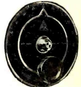
The new Apex Vernier Dial embodies some unusual and original ideas in its design. It consists of two plates, a stationary indicator and a calibrated rotary element, which rotate with a ten to one ratio.
