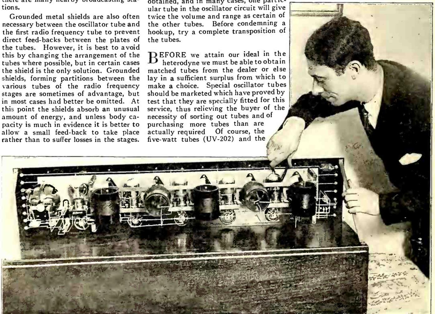
A rear view of a novel neutrodyne receiver constructed by a well known Eastern amateur radio builder, which shows some unusual feats of engineering skill. Note the method of off-setting magnetic coupling between the neutroformers, and the simplified arrangement of the receiver as a whole. The panel is shielded carefully from stray capacity effects, which may be introduced while operating.
