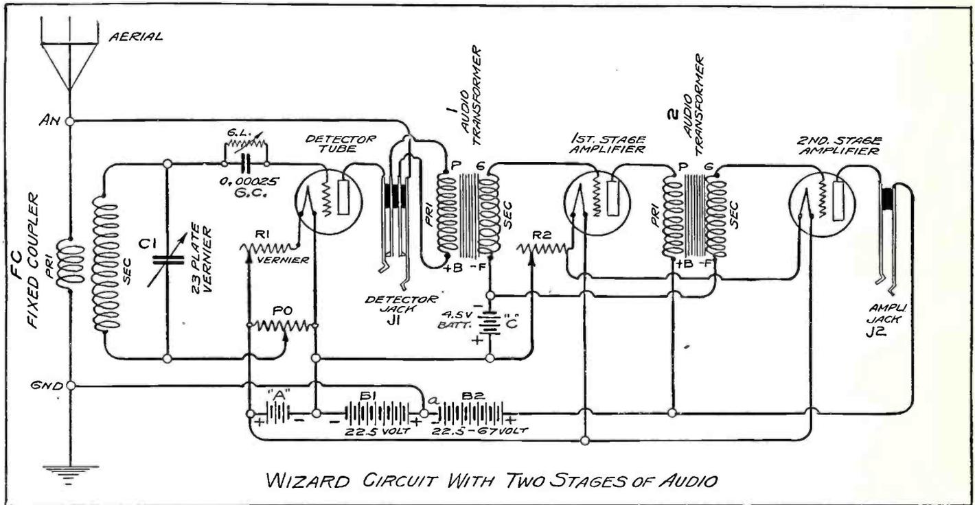
formers only the primary and secondary are marked, as often transformers are not critical to the location of the grid connection (G). With other transformers particular care should be taken to connect the post (G) of the transformer to the grid post of the socket.
