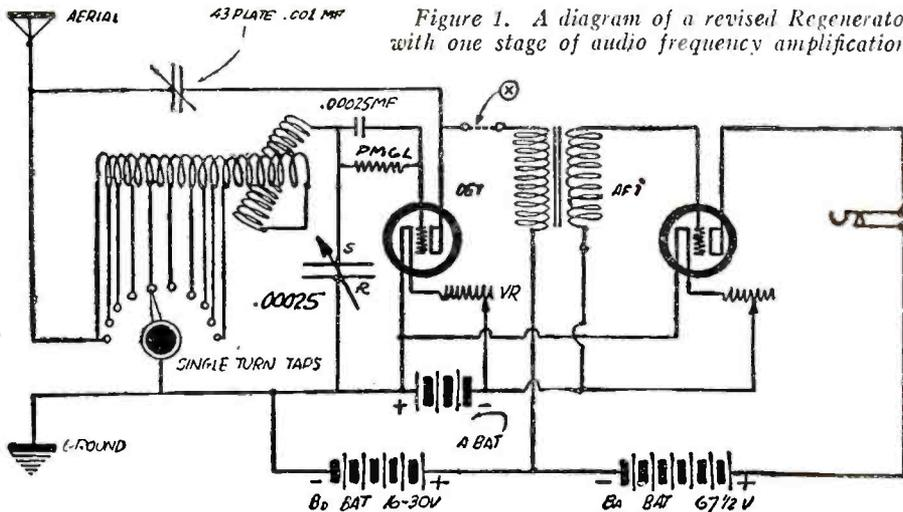
Figure 1. A diagram of a revised Regenerator with one stage of audio frequency amplification.
