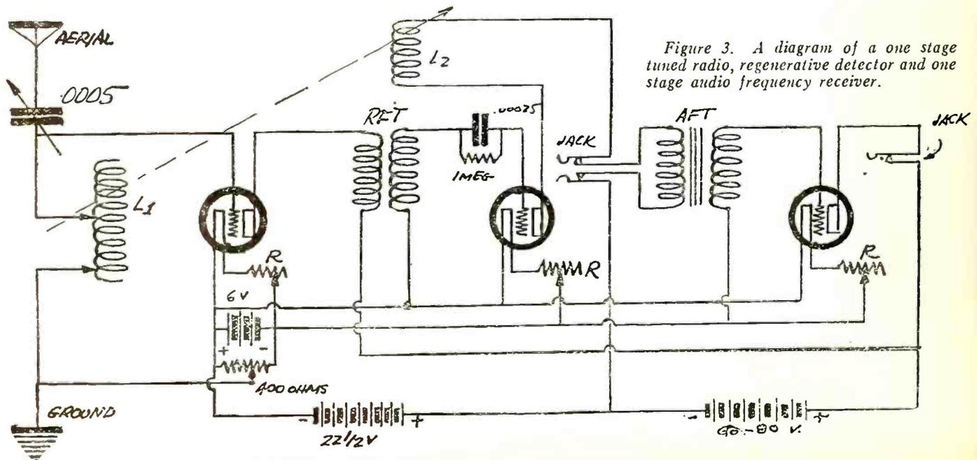
Figure 3. A diagram of a one stage tuned radio, regenerative detector and one stage audio frequency receiver.
