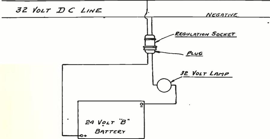
DETERMINE POLARITY OF LINE BY PLACING CHARGING LEADS IN A GLASS OF WATER & BUBBLES WILL ARISE FROM NEG LEAD IT IS VERY IMPORTANT THAT THE NEG. OF THE BATTERY CONNECTS TO THE NEG. OF THE CHARGING LINE & THE POSITIVE OF THE BATTERY TO THE POS. OF THE CHARGING LINE.
