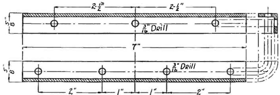
Figure 5. The bracket supporting the shelf is drilled in the manner shown here-with for the best mounting arrangement.
