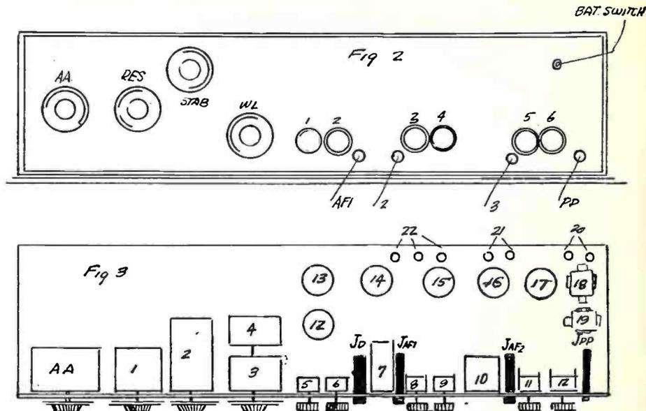
Figure 1b. The layout of the Superdyne receiver.
