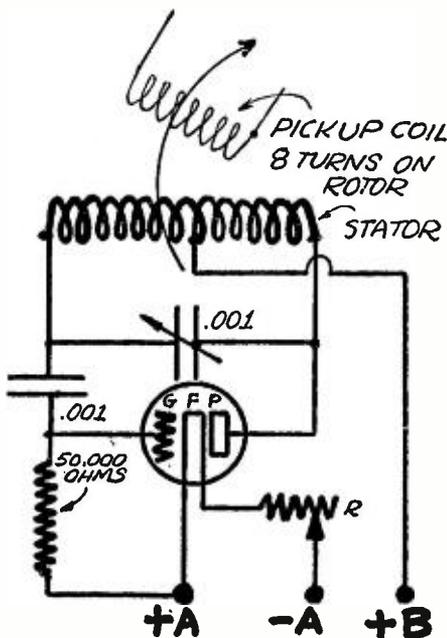
Figure 2. A diagram of the Hartley Oscillator.
