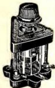
The new Freshman double-adjustable crystal detector has several distinctive features. It has a knob which can be brought through to the panel and when turned varies the crystal contact with the loop-whisker, thus permitting the operator to find sensitive spots
