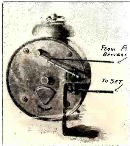
Station KYW, Chicago, broadcasts news bulletins at half-hour intervals throughout the day and night. Paul C. Kahn, 3222 Carroll Ave., Chicago, has invented an alarm clock device that automatically "brings in" the station. The clock is timed with the station time and the alarm is set for the half hour. When the alarm sounds the lever attached to the alarm wind comes down and completes the circuit. When the announcer signs off the clock is again set for the next period.
