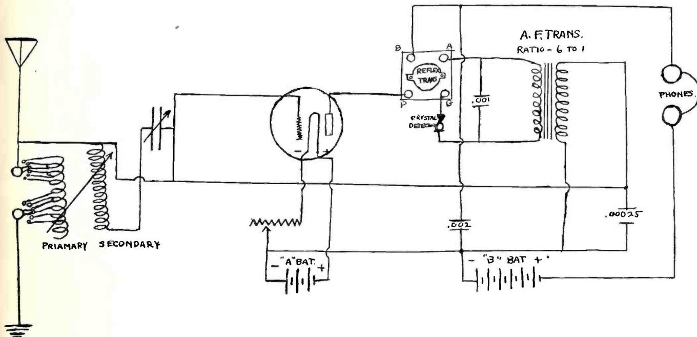
Figure 2—Circuit diagram of the simple reflex receiver.
