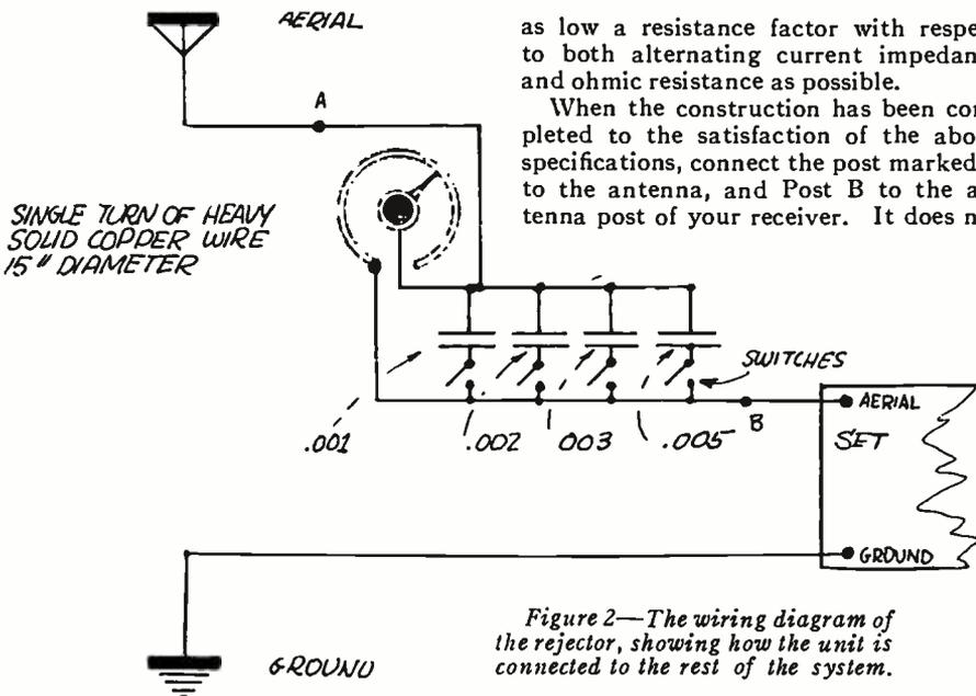
Figure 2—The wiring diagram of the retractor, showing how the unit is connected to the rest of the system.
