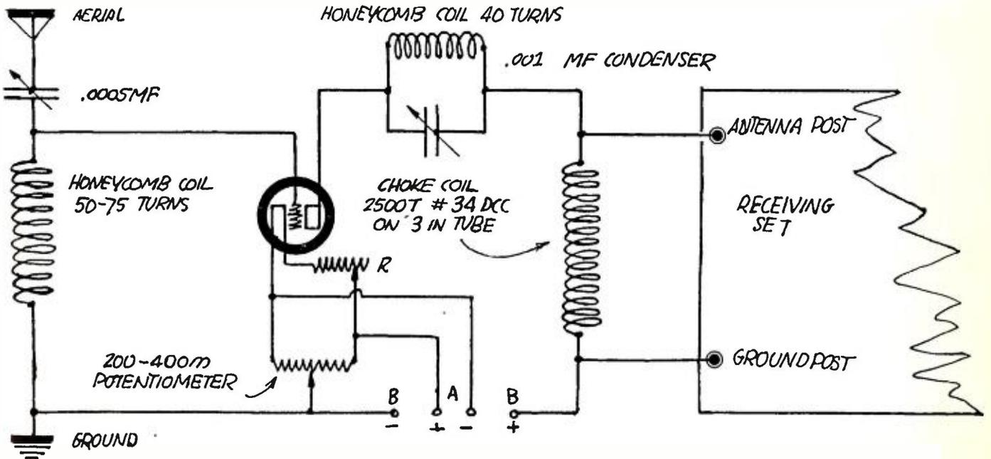
Figure 3—The tube type of rejector is one of unusual merit, and fans who are looking for an elaborate but sure-fire eliminator should try the one described herewith.
