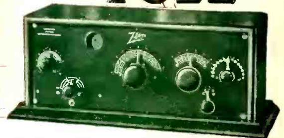
**Model 4R**—The new Zenith 4R "Long-Distance" Receiver-Amplifier comprises a complete three-circuit regenerative receiver of the feed-back type. It employs the Zenith regenerative circuit in combination with an *audion detector* and *three-stage* audio-frequency amplifier, all in one cabinet.
