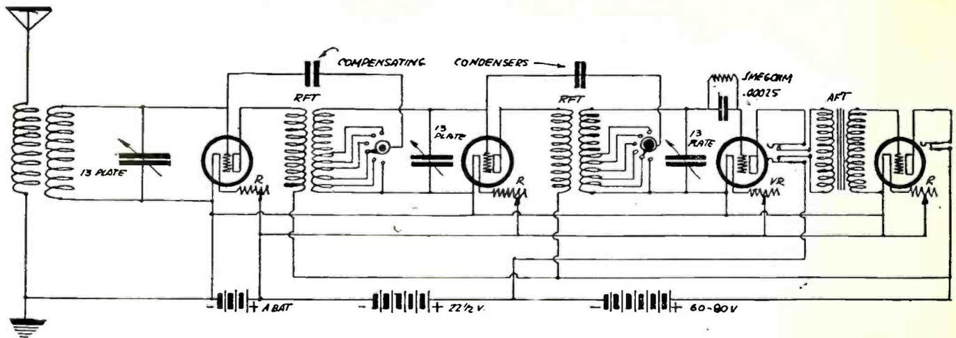
Figure 3. Complete circuit diagram of the Neurodyne set.
