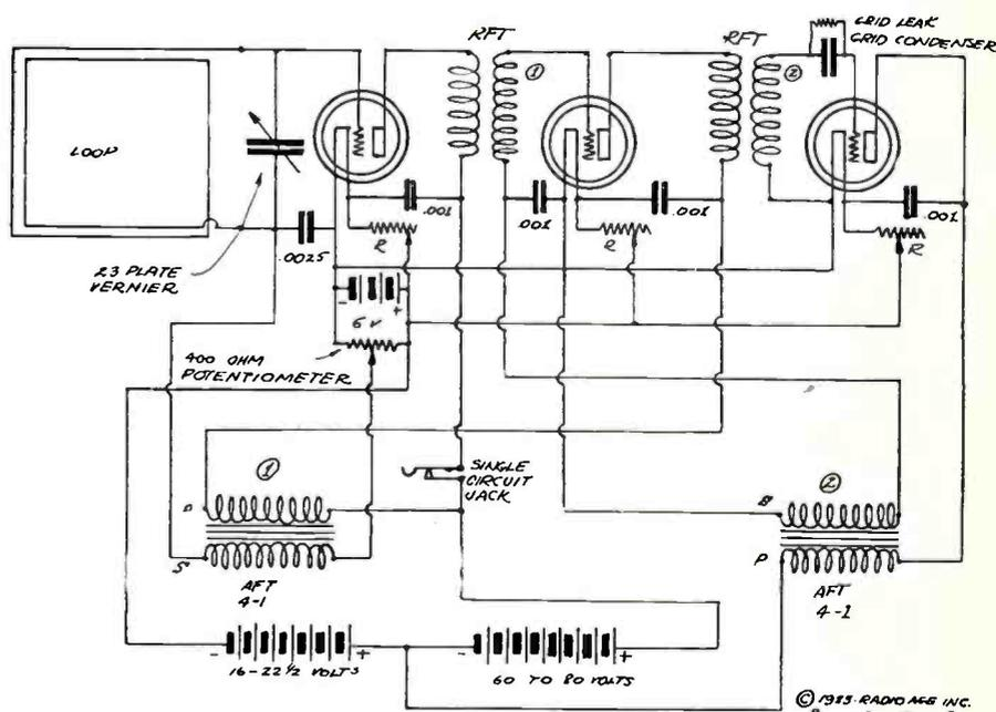
Figure 2. The finished hookup of the Grimes Circuit.
