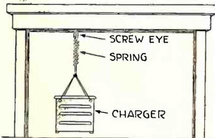
Secure a strong wire to each of the four corners of the charger case. These can be attached by running them through the ventilating holes. All four wires are joined and fastened to a door spring. The charger is then hung from a large screw eye under the table, it need not clear the floor by more than an inch or so. See illustration.—J. C. Heberger.
