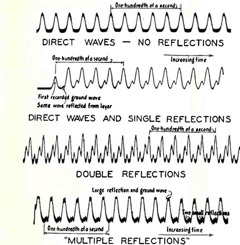
The Highest Hump in Each of These Cases Is Made by Waves Along the Shortest Path; the Smaller Humps and some of the Irregularities Are Caused by Reflections
