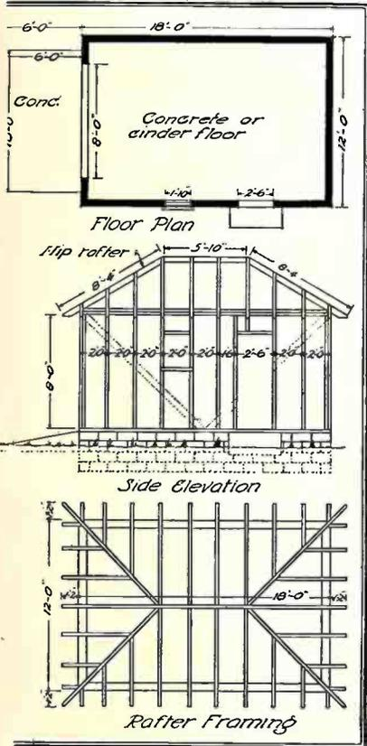
ing, divide into six foot sections with lath on edge between. Later these lath are to be removed and hot asphalt poured in for expansion joints. Of course the ground must be well tamped down before the floor is placed, particularly if you have added any fill.
