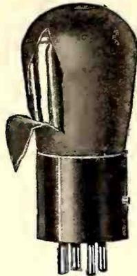
Above is shown the new Strongson self shielded copper plated tube recently marketed by the Moulded Products Corporation. A section of the copper coating is shown laid back. This tube was designed for use in radio sets where tube coupling effects are bothersome. The shielding is connected to the negative terminal of the socket so the tube's coating remains at ground potential.
