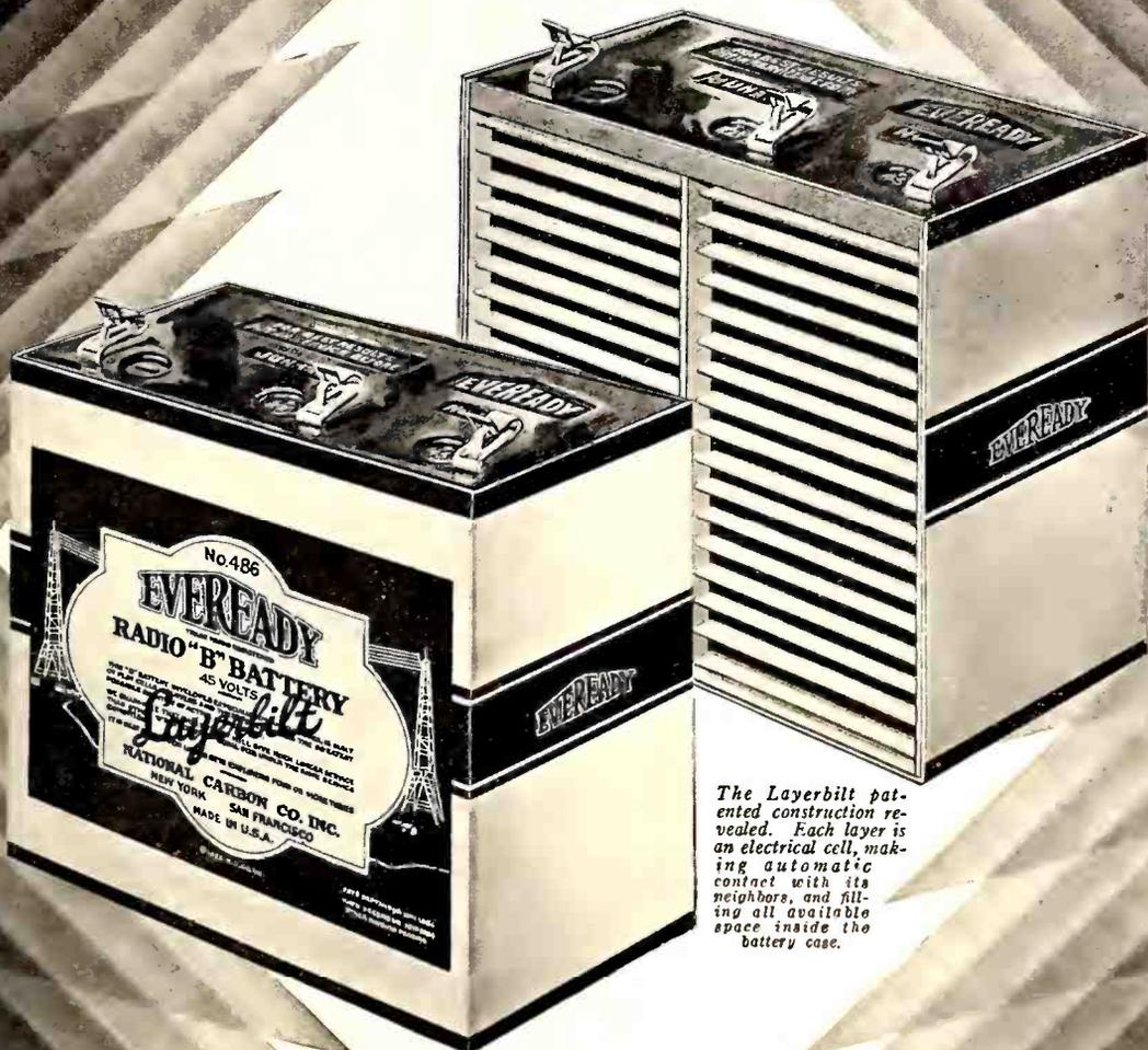
The Layerbilt patented construction revealed. Each layer is an electrical cell, making automatic contact with its neighbors, and filling all available space inside the battery case.
