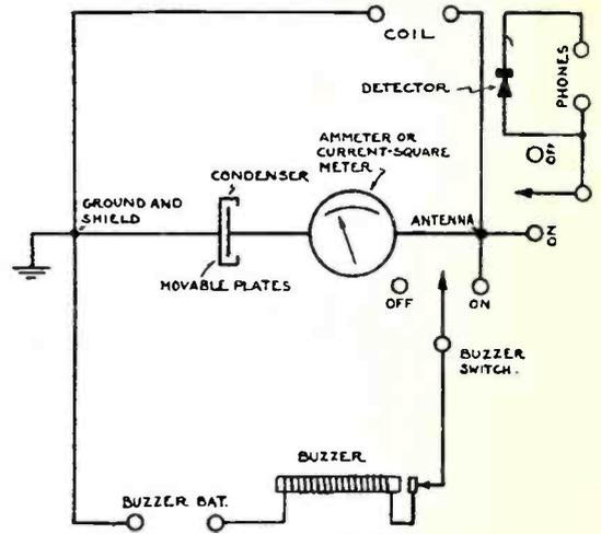
FIG. 2. WAVEMETER CIRCUIT.
