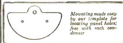
Mounting made easy by our template for locating panel holes; free with each condenser
