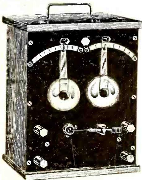
There are two tuning levers on the front. After locating the most sensitive point of the Galena the two levers are moved back and forth until the best result is obtained.
