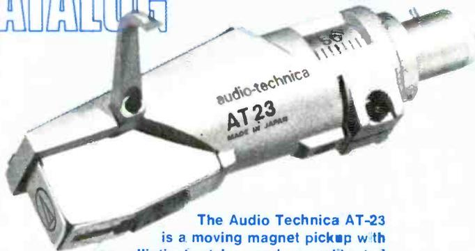
The Audio Technica AT-23 is a moving magnet pickup with an elliptical stylus and a calibrated adjustable overhang with built-in gauge. It has a recommended VTF of 0.9 to 1.7 grams. \$225. Circle 115.
