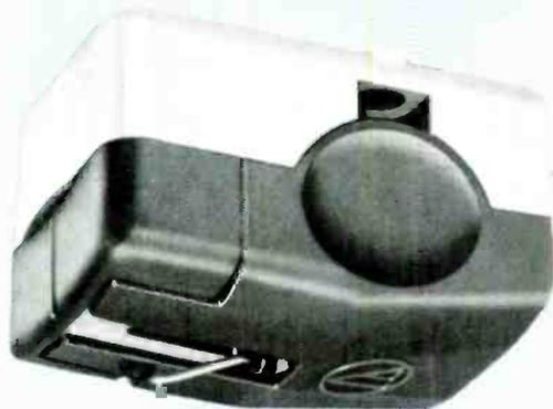
Signet's moving magnet TK3E features a unique flip-down integral stylus guard. The elliptical stylus has a VTF of from 1 to 1¼ grams. Loading capacitance is 270 pF. \$55. Circle number 118.
