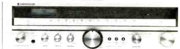
This Kenwood KR-3010 receiver is a good example of a low to medium priced receiver with full features to make it the central component of an economical system. It has an output of 27 watts RMS per channel with no more than 0.05% total harmonic distortion. It has outputs for two sets of speakers and two tone controls. \$280. Circle 75 for info.
