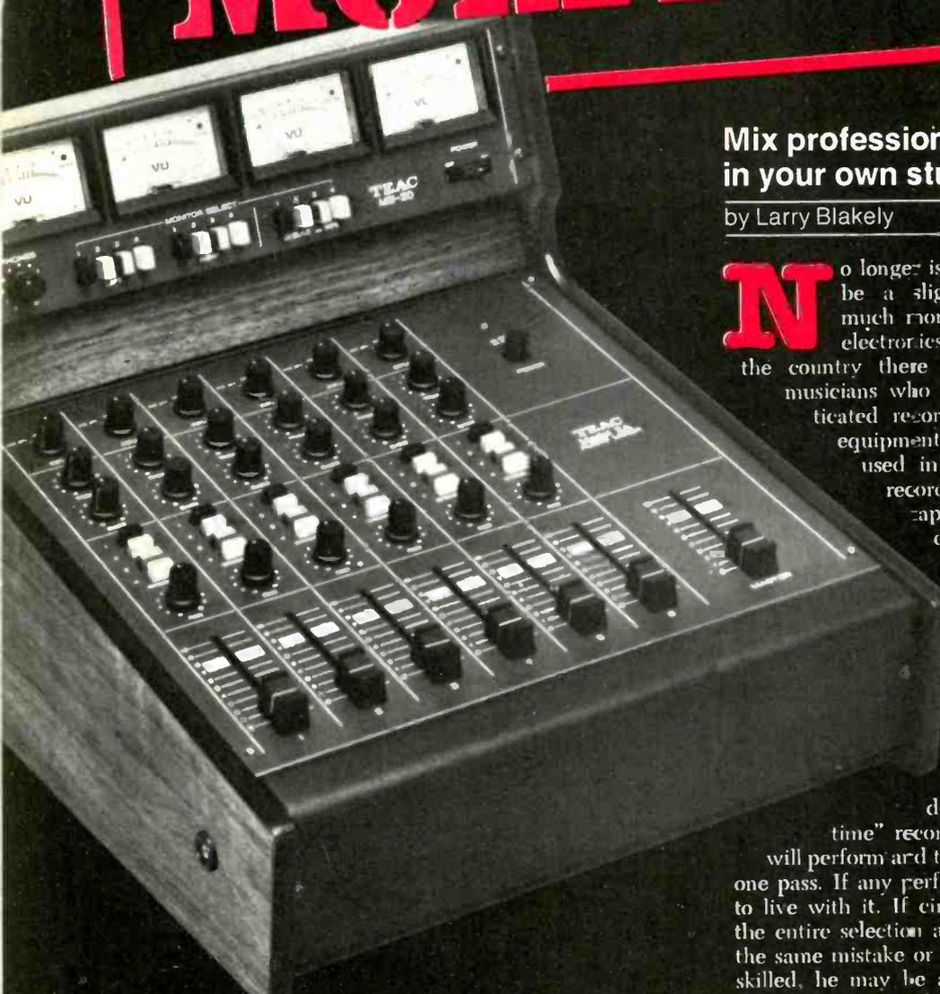
The TEAC model 2A is a six-input, four-output mixer. Each input has switchable mic/line level inputs,  $\pm 12$  dB bass and treble controls, color-coded output selection switches, and slide fader. The unit shown includes the MB-20 meter bridge which monitors the input level sensitivity and the level of the output signal. The mixer has a master output level control and a pan control that lets you move the image from left to right. Model 2A sells for \$475 and MB-20 for \$250. Circle 121.
