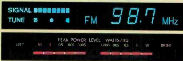
Sansui's patented Digitally Quartz-Locked Circuit uses a precise quartz crystal time base to keep your station locked in, even through many hours of listening or if you turn the receiver off and back on again.
