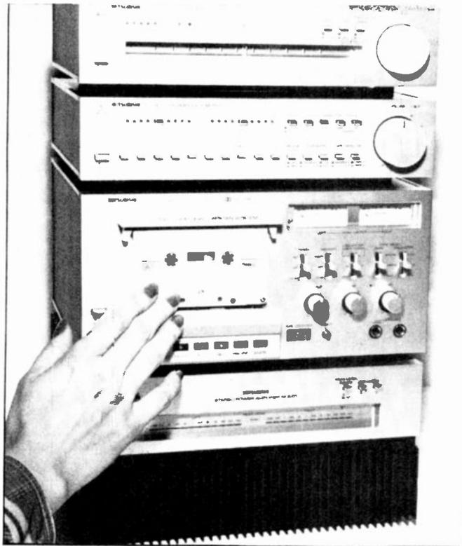
The Mitsubishi micro component system includes: the M-A01 power amp with 70 watts per channel RMS and 0.01% THD (\$500), the M-FO1 quartz-lock tuner (\$340), the M-PO1 preamplifier with a moving-coil head pre-amp (\$370), and the M-TO1 cassette deck with microswitches to control the mechanical parts (\$560). The stack is only 16 1/4 inches high, 10 3/4 inches wide, weighs 54 lbs. Circle 78.
