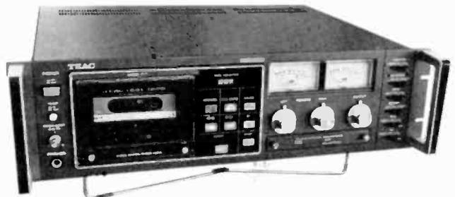
TEAC's C-1 cassette deck may be modified to record and play metal particle tape at a cost of \$150, freight charges included. Modification takes 2 to 3 weeks. The C-1 also offers pitch control, bias optimization modules, optional dbx module. \$1300. Circle Reader Service No. 10 for details.
