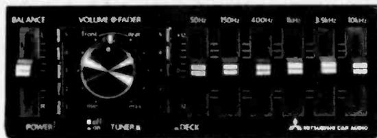
Mitsubishi's CV-23 equalizer/booster is a 6-position unit including volume/front-rear fader knob and left/right balance slide control. \$180. Circle No. 140.
