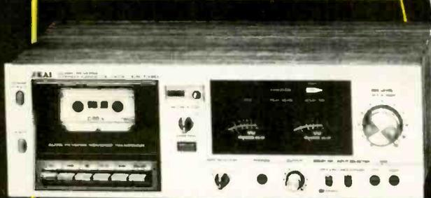
Akai's CS-732D is an automatic reversing cassette deck which also offers Dolby noise reduction, four-position tape selector, and a photosensor "Quick Reverse" which provides instantaneous change of tape direction. \$400. Circle No. 62.
