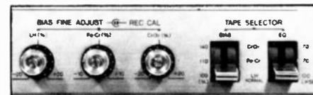
The Dolby and bias calibration controls are coaxial for each tape type. The screwdriver adjustment in the center of each bias adjustment is the Dolby calibration. The bias adjustment is made along with the bias and equalization switches located just to the right of the bias controls.
