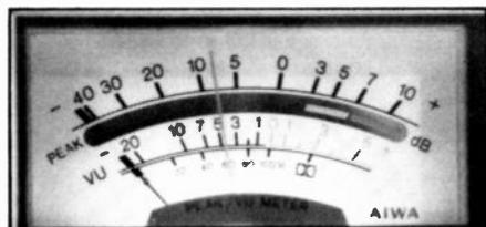
The dual-pointer record-level meters simultaneously indicate the VU and peak signal levels. The peak pointers can also be switched to "hold" a reading after the signal stops, as indicated in this photo. Note the VU pointer is on zero while the peak pointer reads approximately -8 dB.
