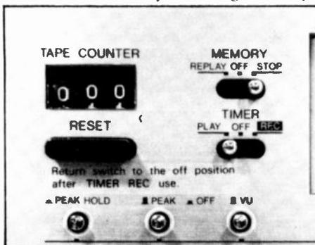
Meter functions are determined by the switches labeled VU, PEAK, and PEAK HOLD. The memory counter and timer switches directly above the meter switches provide automatic repeat play after rewind, as well as powerline control to play/record from a capstan-disengaged preset.
