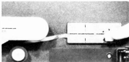
An Editall type splicing block with a built-in guillotine cutter is built into the deck directly after the capstan.
