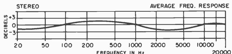
**Performance:** The frequency response measured  $+2/-3$  dB from 20 to 16,000 Hz, with one channel having a steady rise from the midband to 20,000 Hz. Channel balance was within 2 dB from 20 to 10,000 Hz; increasing to 5 dB at 20,000 Hz. The worst-case stereo separation measured 17 dB at 1000 Hz; 10 dB at 15,000 Hz. ▲
