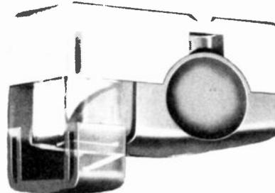
est diamond stylus with the smallest cantilever of any production cartridge known. For example, the cantilever of the TK7SU is just 0.5 mm in diameter at the large end of the hollow tube, tapering to just accommodate the 0.11 mm diamond at the tip. The square-shank stylus can be precisely oriented
