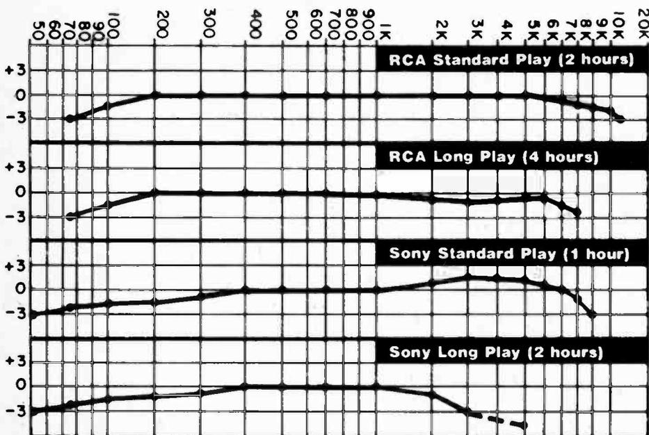
The RCA machine's frequency response at the 2-hour-tape speed was +0/-3 dB from 75 to 10,500 Hz. The 4-hour-tape speed yielded a response of +0/-3 dB from 80 to 8000 Hz. The frequency response of the Sony VCR at the tape speed used to make 1-hour tapes (4 cm/sec.) was 75 to 9000 Hz +1/-3 dB, down 5 dB at 50 and 1000 Hz. At the 2-hour tape speed, the response was down 3 dB at 4000 Hz.
