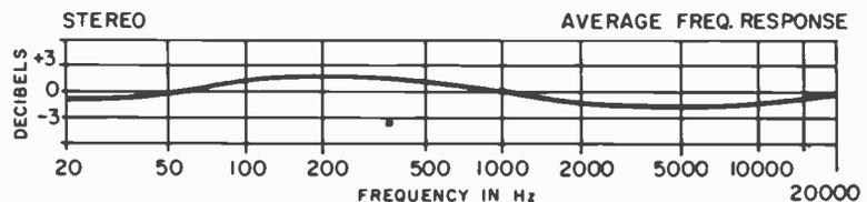
**Performance:** The frequency response measured within  $\pm 2$  dB with an unusually flat upper high end. Channel balance was within 0.25 dB to 18,000 Hz, rising to 1.5 dB at 20,000 Hz. The worst-case stereo separation was 26 dB at 1000 Hz; 23 dB at 15,000 Hz. ▲
