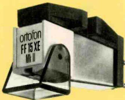
Ortofon FF15XE Mk II magnetic phono pickup utilizes an elliptical stylus and has a recommended tracking force of 2 grams. Its recommended load capacitance is 400 pF. \$40. Circle R. S. No. 115.
