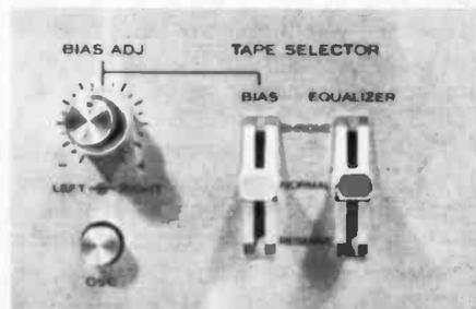
Pressing the OSC button automatically disconnects the input signal and applies the bias test tones alternately to the tape. Left and right bias level are individually adjusted through concentric controls.
