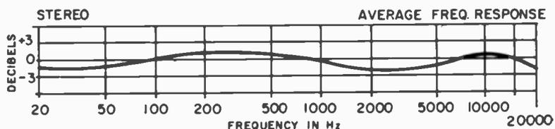
**Performance:** The frequency response measured within  $\pm 2$  dB from 20 to 20,000 Hz. Channel balance was better than 1 dB. The worst-case stereo separation measured 26 dB at 1000 Hz; 21 dB at 15,000 Hz.
