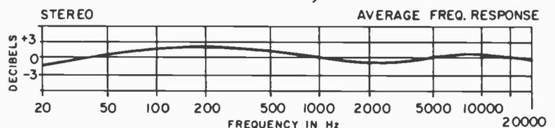
**Performance:** The frequency response measured within +1.5/-1 dB from 20 to 20,000 Hz. Channel balance was within 1 dB from 20 to 20,000 Hz. The worst-case stereo separation measured 23 dB at 1000 Hz; 20 dB at 15,000 Hz. ▲
