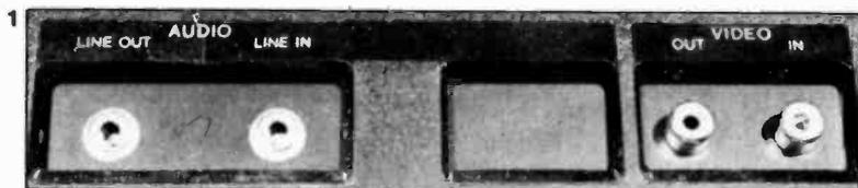
(1) On the Sony machine, the audio and video connections are automatically switched over only when the appropriate patch cords are plugged in. The idea is fail-safe and a delight to use. (2) RCA's VHS machine has the modulator completely built in and the user selects either channel 3 or 4 for operation. No viewing area has stations assigned to both stations. Always check with your dealer to make sure that the machine you buy will work in your home.
