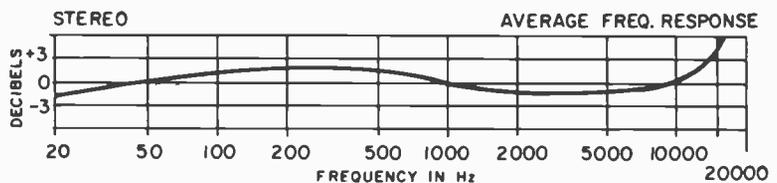
**Performance:** The frequency response measured within  $\pm 2$  dB from 20 to 14,000 Hz, rising to +6–7 dB at 20,000 Hz. Channel balance was within 1 dB. The worst-case stereo separation measured better than 30 dB at 1000 Hz, 18 dB at 15,000 Hz. The overall sound quality is slightly edgy in the upper highs because of the rising response. The rise can be reduced by adding capacity through shielded patch cord extensions. ▲
