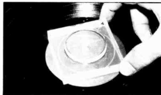
When the turntable is assembled, with its locking screws released, check for 360° balance with a gauge like the Audio Kare AK-5, or a floating platter, adjust the support screws; adjust the feet, using tape shims, if necessary.
