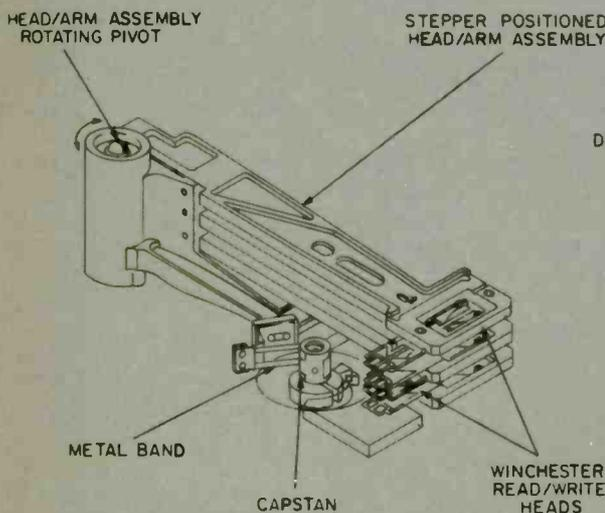
Fig. 3. Read/write functions are performed by the sensors at the end of the radial arm, a diagram of which is shown above.
