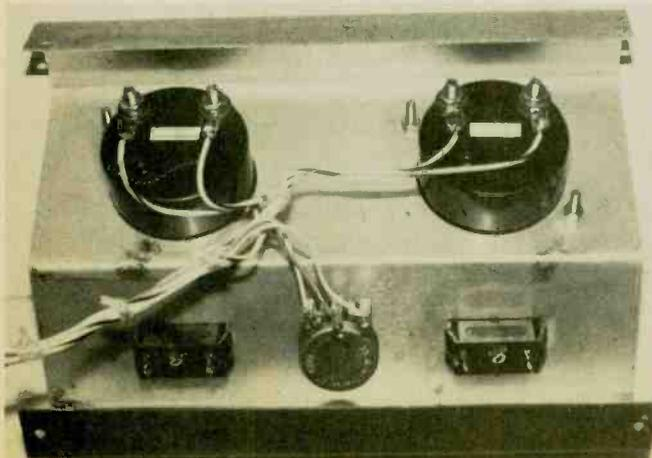
Looking down at the Solar Cell Tester. Chassis, meters, switches, and the calibration control can be seen. If you look carefully, you will notice the wire shunt (R<sub>m</sub>) across the panel meter on left.
