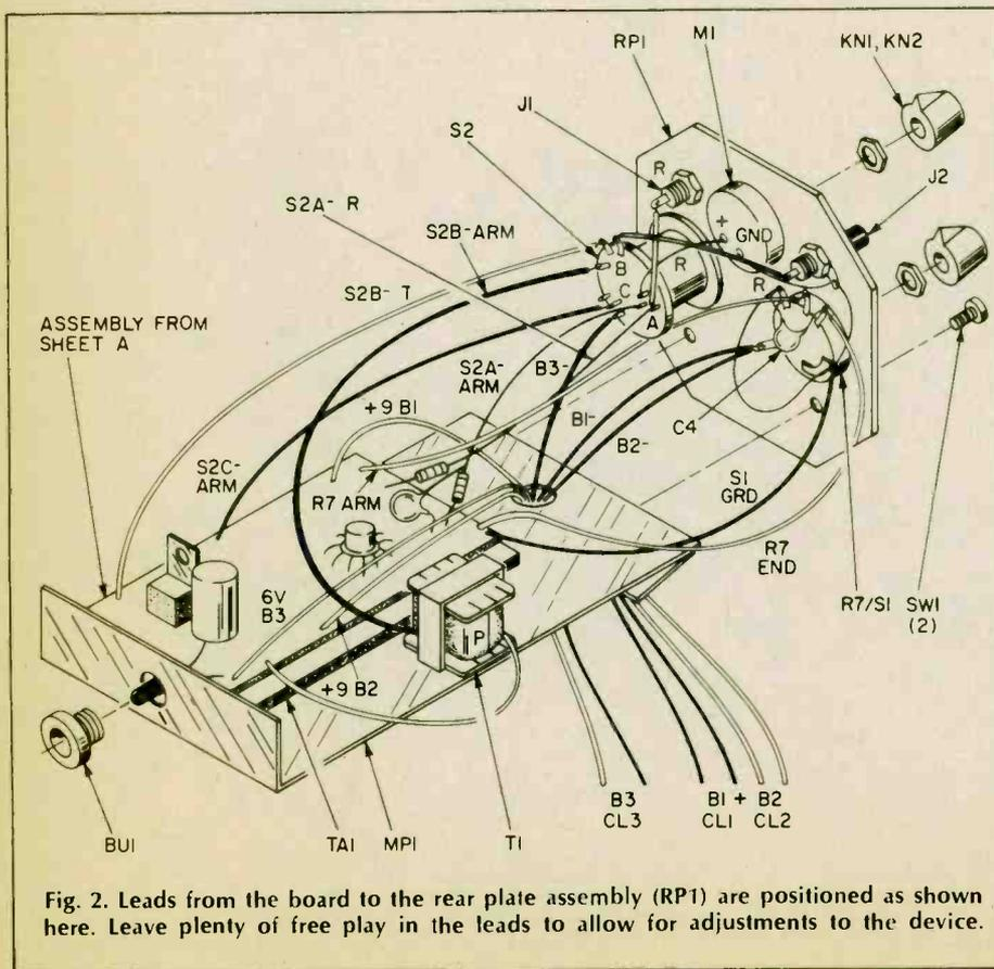
Fig. 2. Leads from the board to the rear plate assembly (RP1) are positioned as shown here. Leave plenty of free play in the leads to allow for adjustments to the device.
