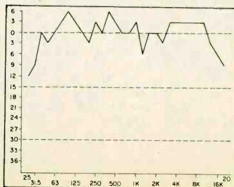
Fig. 10. Floor mounting improves the bass portion, with a moderate boost at mid band.
