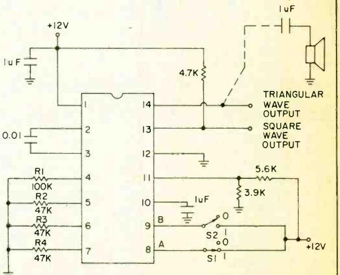
Figure 2. Schematic of frequency control arrangement is at left. The frequency-determining capacitor is connected as shown.
