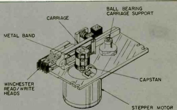
Fig. 2. The stepper motor turns the disk drive capstan; it receives its instructions from the controller board interface.
