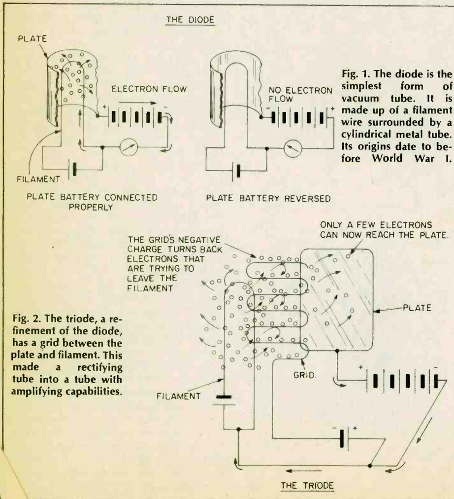
Fig. 1. The diode is the simplest form of vacuum tube. It is made up of a filament wire surrounded by a cylindrical metal tube. Its origins date to before World War I.
