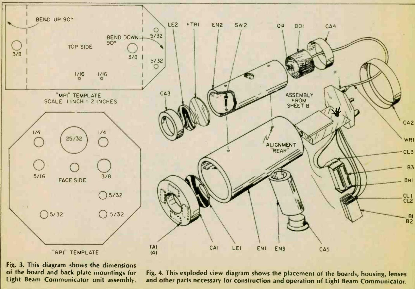
Fig. 3. This diagram shows the dimensions of the board and back plate mountings for Light Beam Communicator unit assembly.
