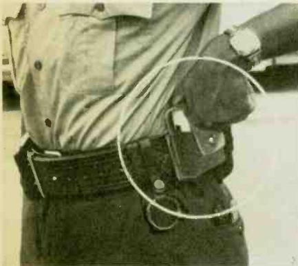
The Rescu unit on the patrolman's belt gives no indication as to its purpose. Once activated, it flashes a signal to the patrol car initiating a repeat of the last transmitted signal with an added beep.
