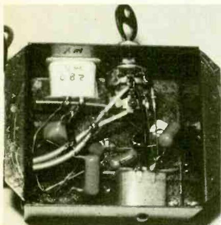
Two homemade inductors are used in this volume control; a 280 mH and a 400 mH.
