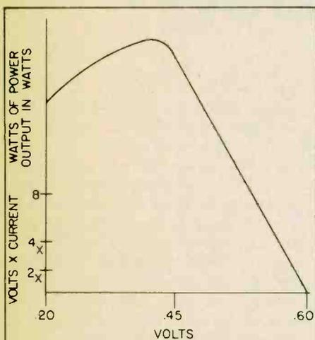
Graph above shows how the solar cell's power output in watts will vary according to voltages above and below rated voltage.
