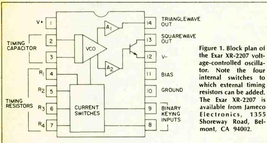
Figure 1. Block plan of the Exar XR-2207 voltage-controlled oscillator. Note the four internal switches to which external timing resistors can be added. The Exar XR-2207 is available from Jameco Electronics, 1355 Shoreway Road, Belmont, CA 94002.
