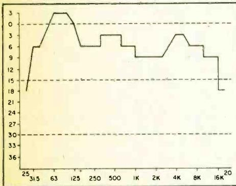
Fig. 2. The response level is raised by 3 dB when the right speaker is switched on.
