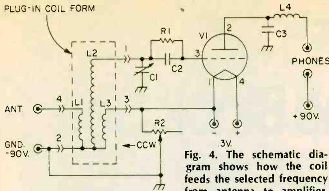
Fig. 4. The schematic diagram shows how the coil feeds the selected frequency from antenna to amplifier.
