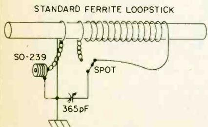
Schematic for simple loopstick antenna. See text and box for further instructions.
