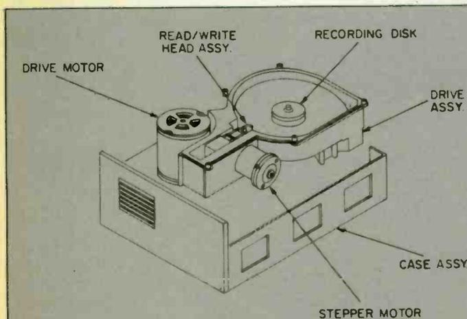
Fig. 1. The complete Winchester unit is shown in this diagram. Note how drive assembly and read/write heads are sealed in.
