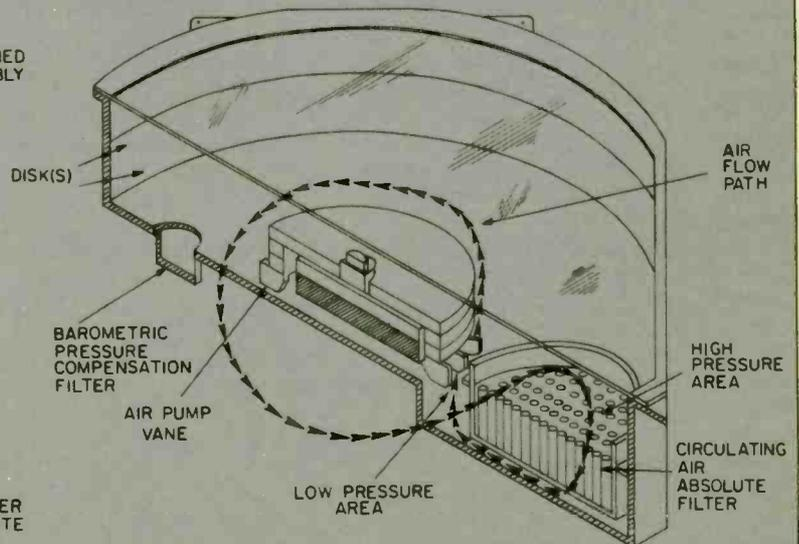
Fig. 4. Air circulation within the sealed disk drive is made possible by the rapidly spinning disk, which allows circulation.
