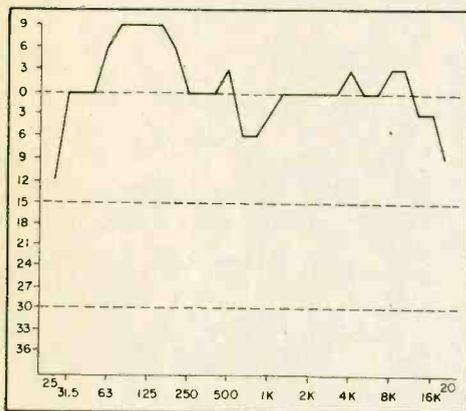
Fig. 8. Placing speakers on the floor is responsible for the dramatic bass response.
