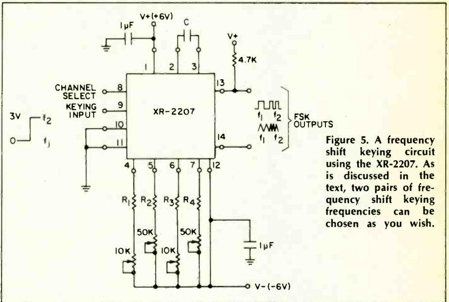
Figure 5. A frequency shift keying circuit using the XR-2207. As is discussed in the text, two pairs of frequency shift keying frequencies can be chosen as you wish.
