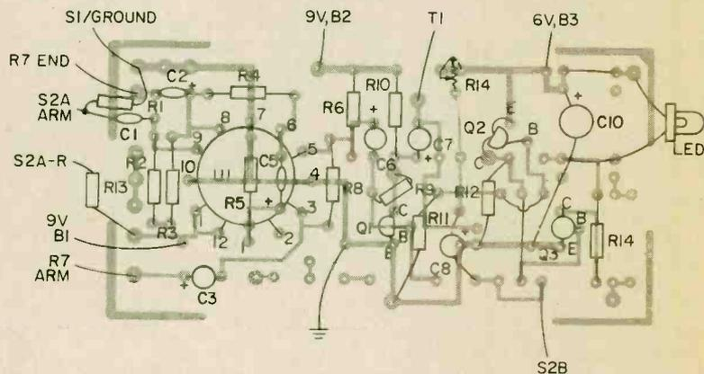
The parts overlay shows components on top of PC board. Note that all of the electronic components fit handily on board, making for easy assembly.
