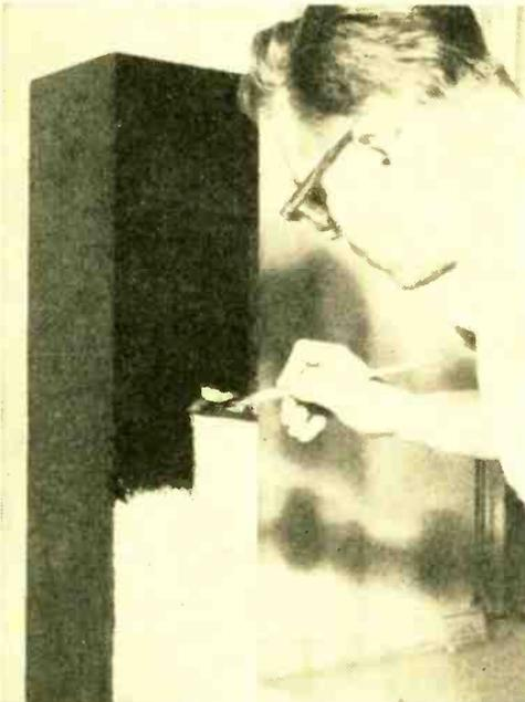
COAT the assembled column with flat, black paint. It will highlight grille cloth's coloring.
