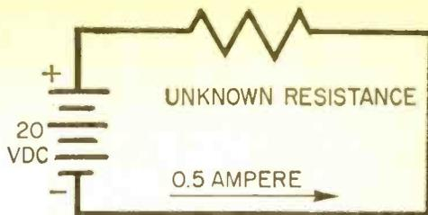
Fig. 16. Knowing the dry cell voltage and circuit current, the unknown R can be found.
