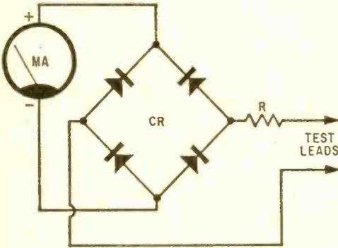
Fig. 11. Full-wave bridge rectifies AC.
