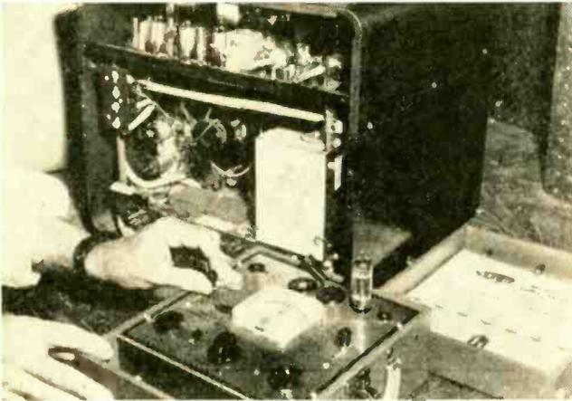
Some servicemen claim that 95% of all radio and TV set faults can be eliminated by replacing a vacuum tube. This kind of service anyone can do, including a housewife (upper right). If you have your own tube tester (left), you can cut out those trips to the corner drug store. Remember, in TV sets there are one or more tubes hidden in the HV cage (upper right). Be careful! Be sure to short out the high voltage to ground.
