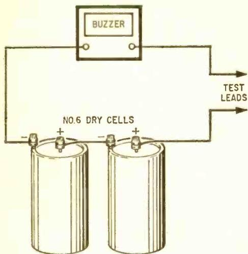
Fig. 1. The continuity checker shown above is an inexpensive testing device for checking wire shorts and opens in long hidden cables.
