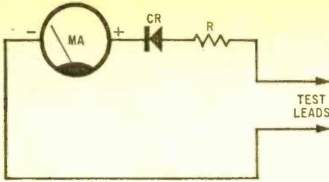
Fig. 9. Rectifier makes DC circuit go AC.
