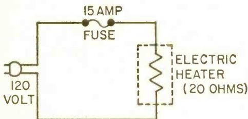
Fig. 15. Here, Ohm's law helps you determine whether the fuse size is satisfactory.
