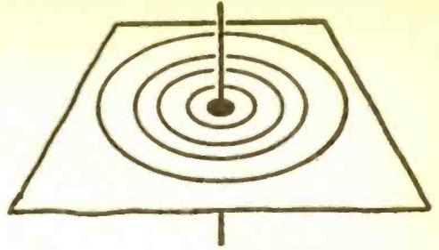
Fig. 24. The magnetic lines of force around a conducting wire is illustrated above.
