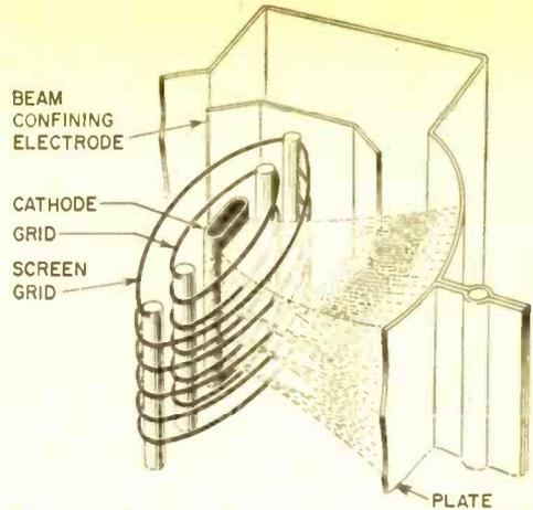
Fig. 8. The beam power tube focuses the electron cloud and aims it at the plate.
