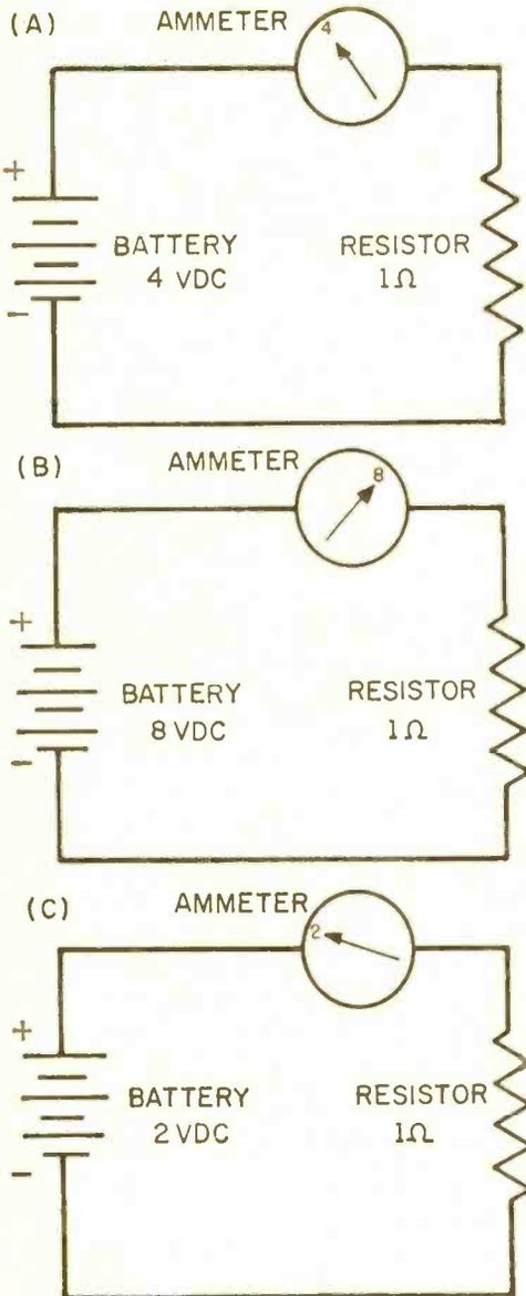
Fig. 10. Simple demonstration showing that current in a circuit is inversely proportional ( $I$  over  $R$ ) to the resistance in the closed circuit.
