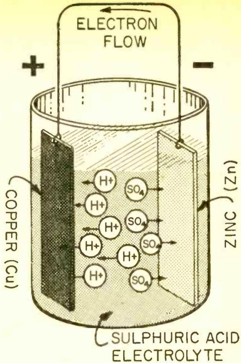
Fig. 1. Allesandro Volta's Zn-Cu cell.
