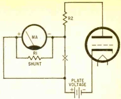
Fig. 5. A milliammeter with shunt resistor measuring plate current. Shunt bypasses most of plate's current so meter is not overloaded.
