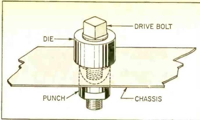
Fig. 3. If you don't have a complete set of Greenlee round and square punches, it's time you start buying. Start off with a  $\frac{5}{8}$ " ,  $\frac{3}{4}$ " , and  $1\frac{1}{8}$ " round punch and a 1" square punch. Parts stores stock these and other sizes and shapes.
