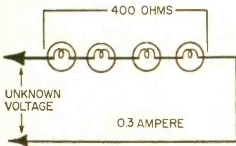
Fig. 13. Find the unknown voltage impressed across this series Christmas lamp circuit.
