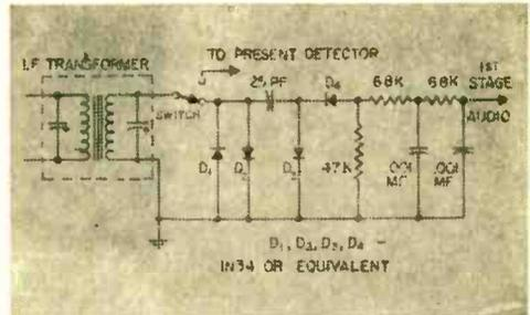
However, assuming you use it with a broadcast or communications receiver, it will only detect narrow-band FM such as is permissible but seldom used on the ham bands; and possibly that used in the 30-40 mc emer-
