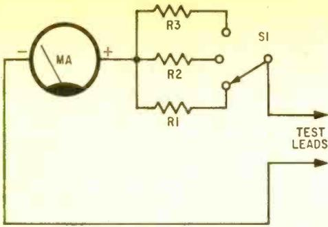
Fig. 4. DC voltmeter with three ranges.
