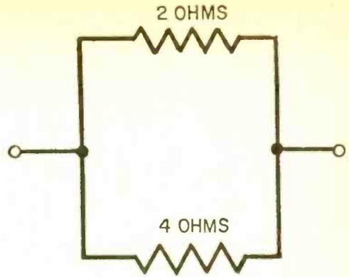
Fig. 19. Parallel resistance can be computed by the simple "product over the sum" rule.
