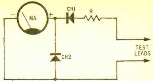
Fig. 10. CR2 eliminates negative pulses.
