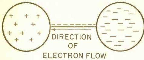
Fig. 5. Electron flow reduces charges.
