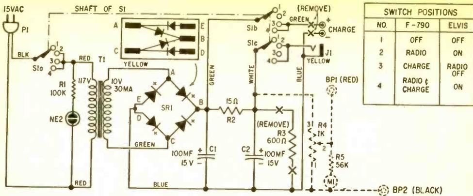
Schematic diagram for ELVIS. Dashed lines are circuit parts added to the Lafayette F-790.
