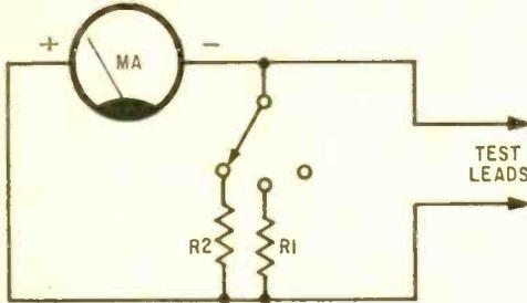
Fig. 6. A multi-range DC milliammeter.
