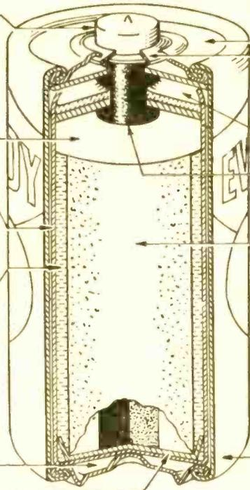
Fig. 2. "Cut away" detail diagram of a typical flashlight dry cell.
