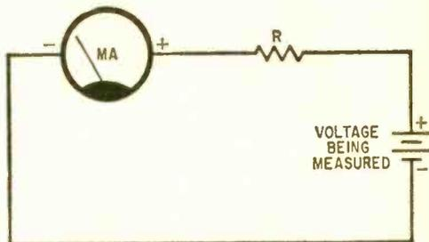
Fig. 3. Simplified DC voltmeter circuit.
