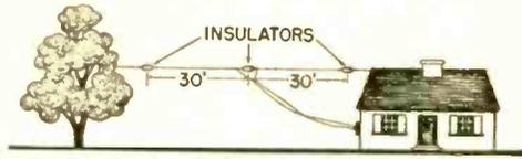
The simplest antenna for broadcast band reception is simply a 50-foot piece of wire run from the receiver, out a window, to any convenient tall support. It will not have the interference rejection of the di-poles fed with the twisted pair line, but in a quiet location it will do a good job with a good receiver. And if you are on a budget, this long-wire antenna can also serve for short-wave reception.
