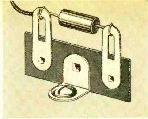
Fig. 6. Mechanically secure leads to lugs.
