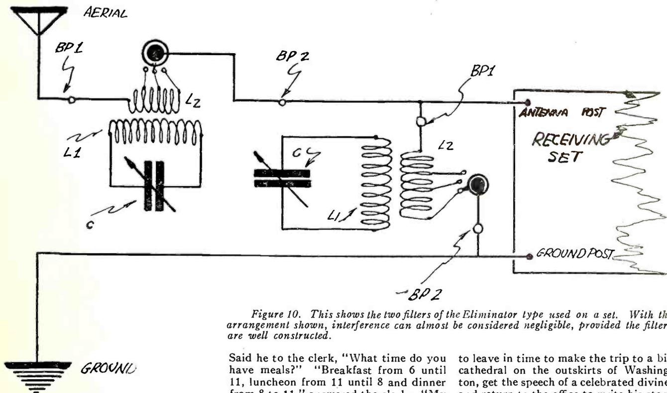
Figure 10. This shows the two filters of the Eliminator type used on a set. With the arrangement shown, interference can almost be considered negligible, provided the filters are well constructed.
