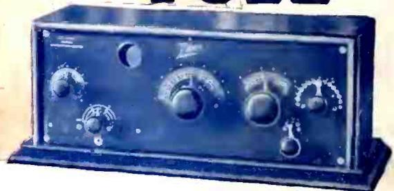
**Model 4R**—The new Zenith 4R "Long-Distance" Receiver-Amplifier comprises a complete three-circuit regenerative receiver of the feed-back type. It employs the Zenith regenerative circuit in combination with an *audion detector* and *three-stage audio-frequency amplifier*, all in one cabinet. Because of the unique Zenith "selector," unusual selectivity is accomplished without complication of adjustment.
