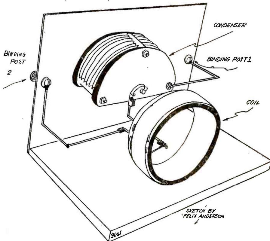
Figure 1. Isometric sketch of the Simple Series Eliminator. The condenser is a 23-plate, and the coil has 40 turns of No. 28 DCC wire wound on a three-inch cardboard tube. A filler of this type is useful in assisting to tune out interference from nearby stations.
