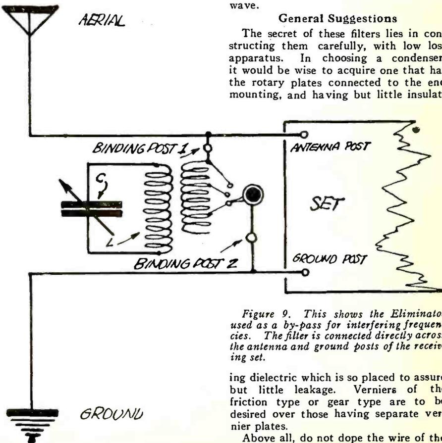
Figure 9. This shows the Eliminator used as a by-pass for interfering frequencies. The filler is connected directly across the antenna and ground posts of the receiving set.
