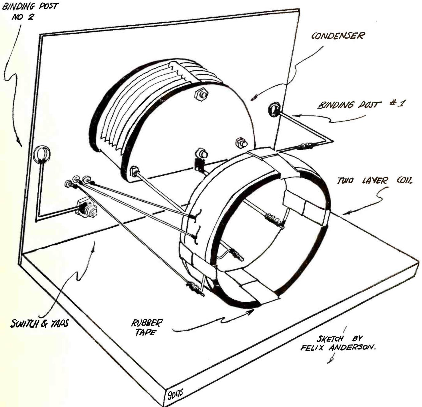
Figure 6. The isometric arrangement of the Eliminator.
