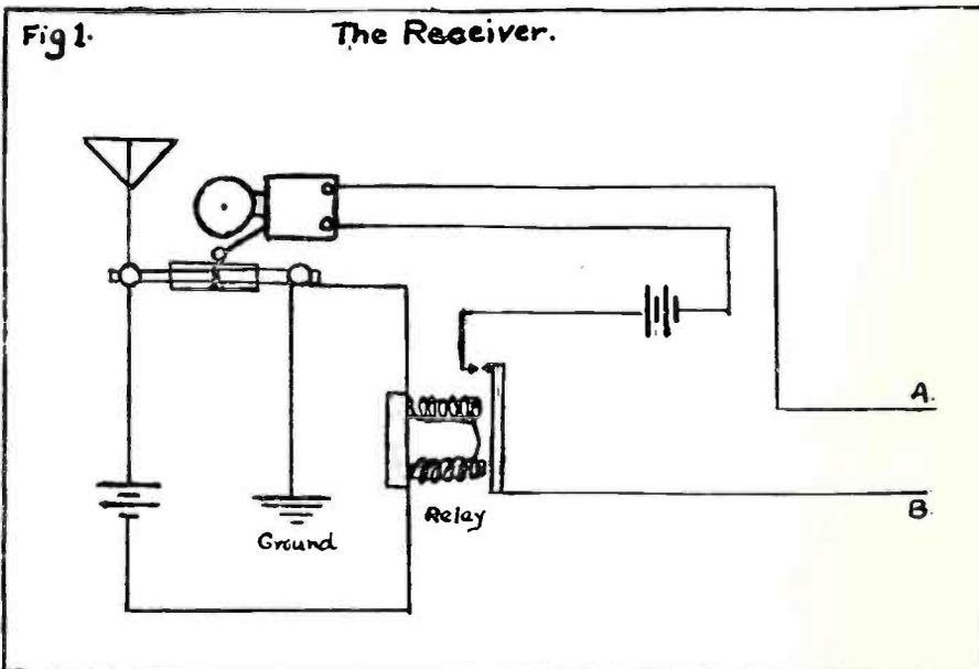
allowing the current to pass and operating the relay. But when once the filings have cohered, they will remain so, unless some means is provided to decohere them. Hence an electric bell is placed in the circuit as shown in Fig. 1. When the relay allows the current to pass, the bell will ring, and the hammer will tap the glass tube, causing the filings to decohere. An ordinary telegraph relay is used.
