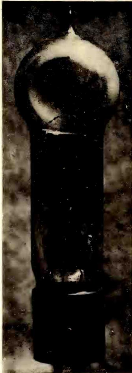
**Y**OU can truly say now that vacuum tubes have eyes, at least electrically. The tube shown above is the thermionic photo-electric tube which is adaptable to transmission of photos either by wire or radio. Much experimental work is being done on this phase of transmission and the story by Mr. Zworykn should be of interest to photo-transmission fans.
