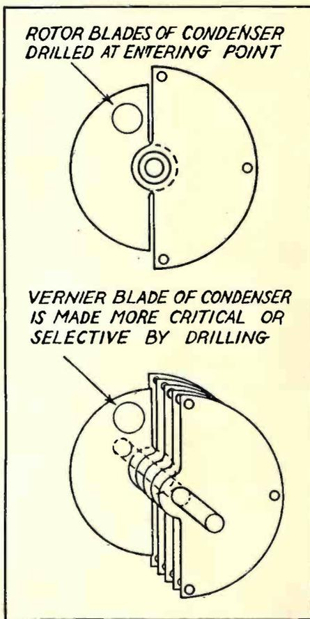
The sketch shown above explains pictorially the manner in which Mr. Luers makes capacity changes in his condensers so as to get the s. l. f. characteristic without buying a condenser of that type. If you contemplate drilling the rotor, do not drill the stator. In other words only one of the elements should be drilled, either the stator or the rotor.
