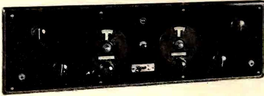
Front panel view of the Microflex, showing the switch located at center of panel
