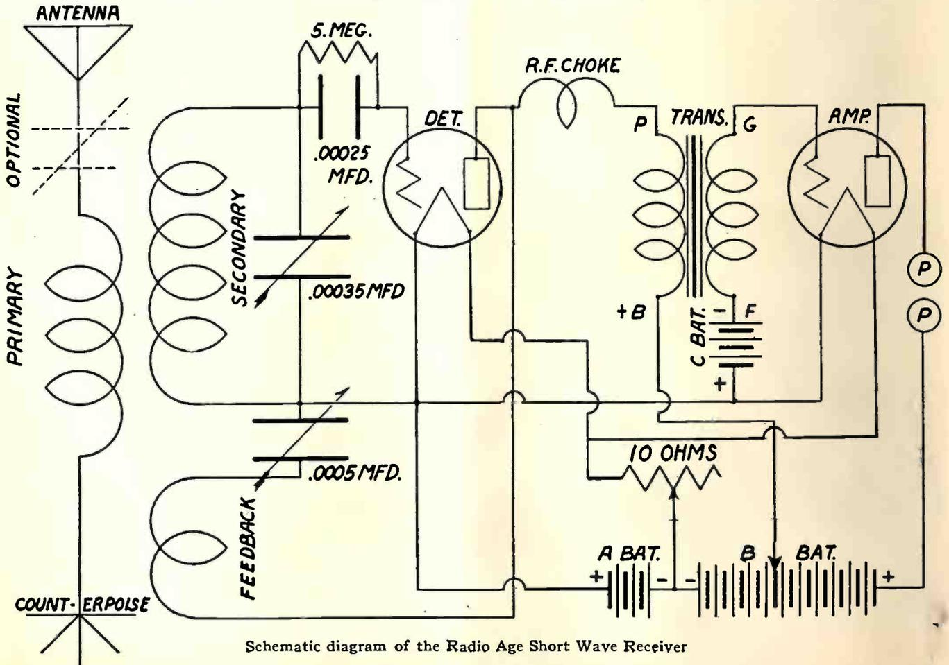
Schematic diagram of the Radio Age Short Wave Receiver
