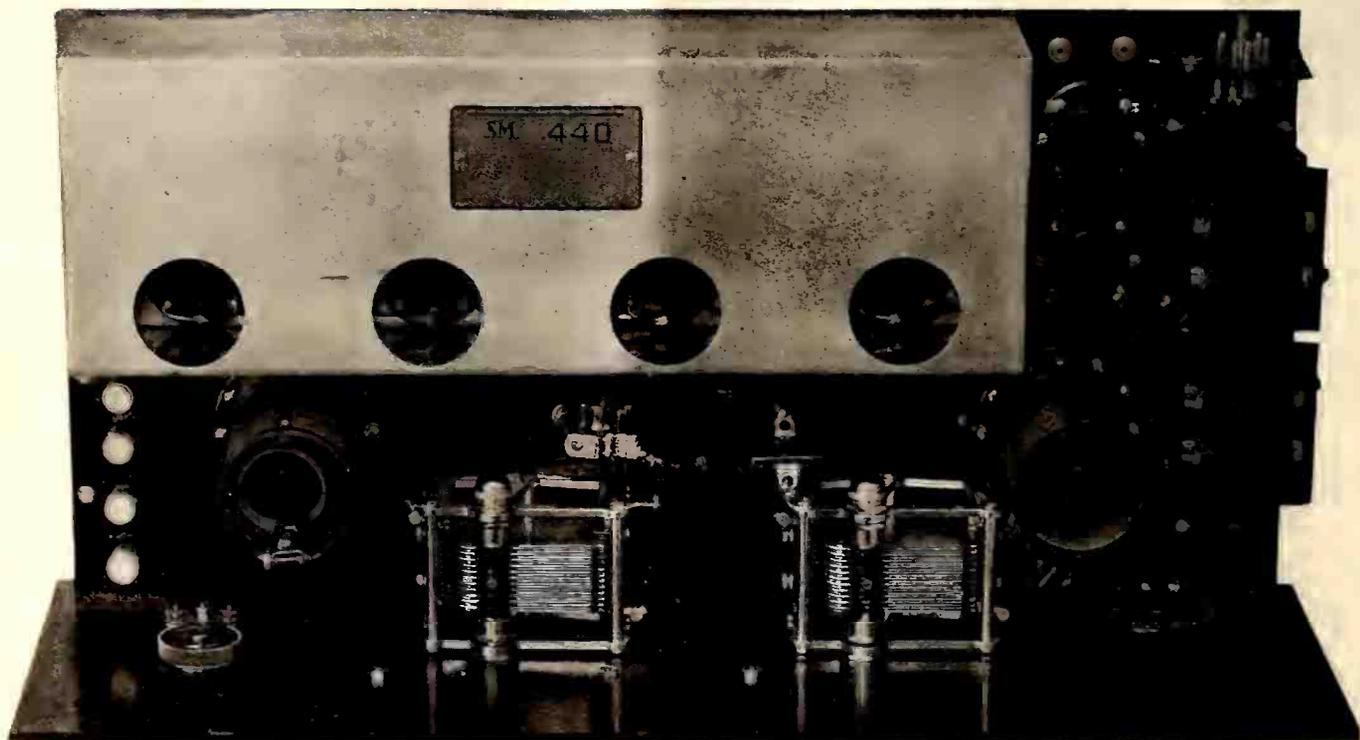
Figure 1.—Back panel view of Quadrode Superheterodyne
