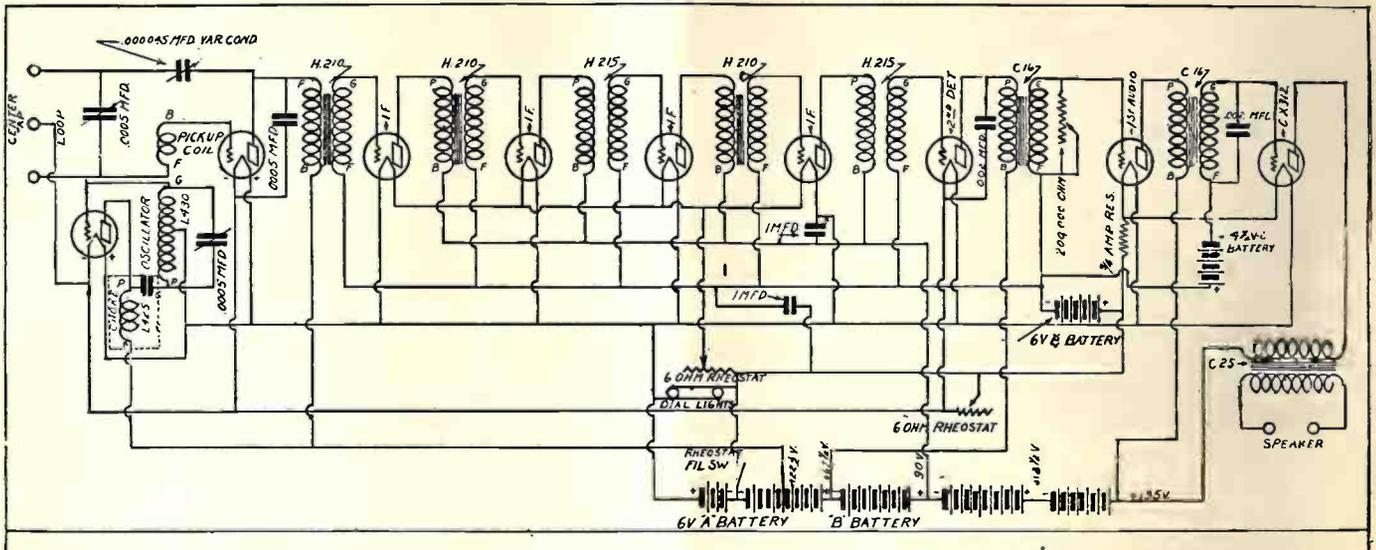
Figure 4—Schematic diagram of the Nine-in-Line.
