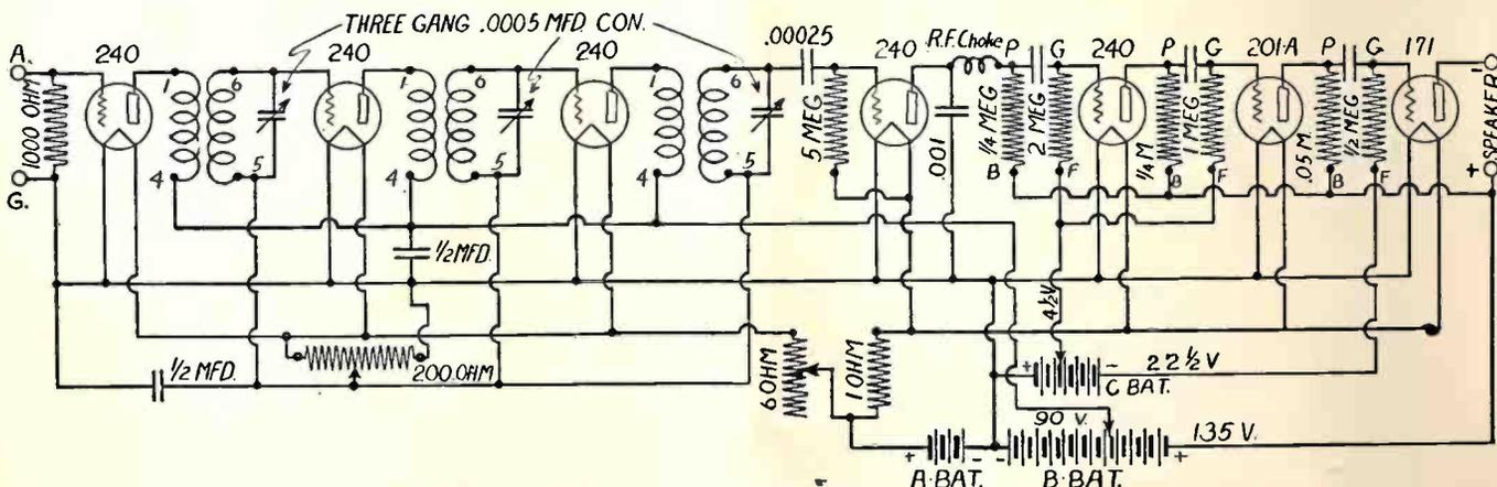
Figure 2—Schematic diagram of the Aero-Seven.
