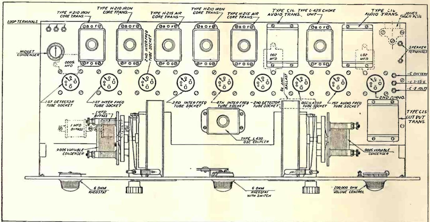
Figure 2—Showing the relative positions of parts in the 1928 Nine-in-Line Receiver.
