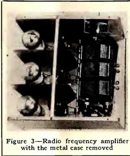
Figure 3—Radio frequency amplifier with the metal case removed
