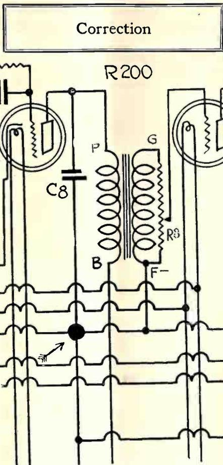
In the blue print section of the September issue, page 19, the circuit diagram of the Radio Age 6-Tube A C Receiver does not show the grid returns connecting to negative B lead. The correction is illustrated in the accompanying section of the original circuit lay-out.
