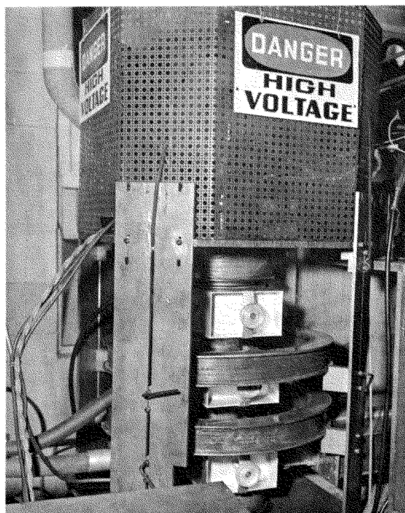
Fig. 8—The 5-kw klystron on test.
