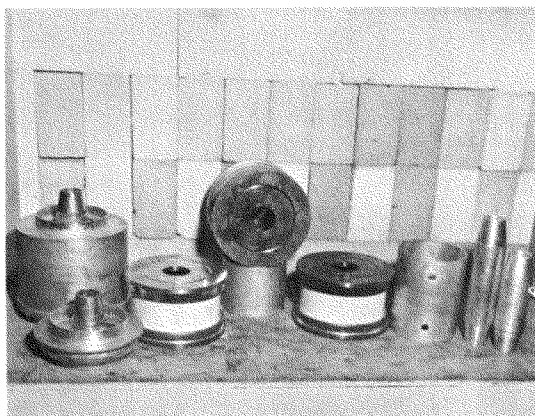
Fig. 7—Tube cavity parts and drift tube sections.
