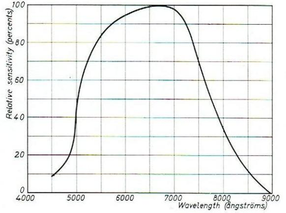
Spectral response curve of the cadmium-sulphide photoconductive cells.
